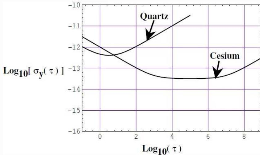
Figure 1: Cesium clock and quartz oscillator typical Allan deviations plotted.
