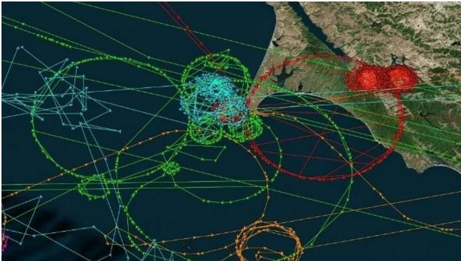
Figure 12: Vessel affected by GPS Jamming
