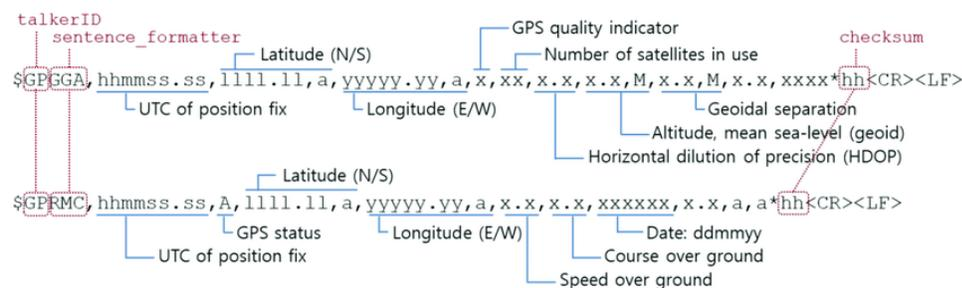
Figure 7: NMEA Protocols and format of GPS fix
