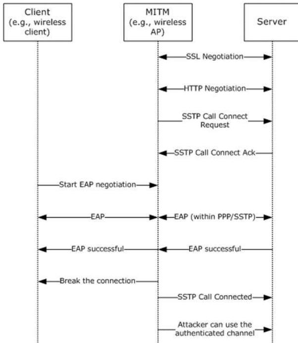
Figure 14: MITM scenario without the SSTP crypto binding solution
