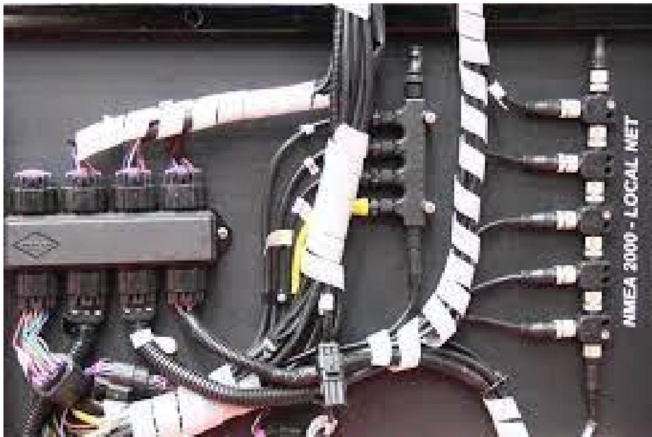
*Figure 5: NMEA 2000 for mercury outboard engine*
