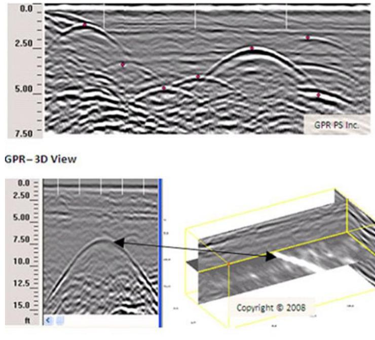
Figure 2.13. Locating Pipelines using Ground Penetrating Radar Technology
