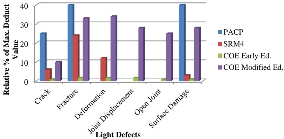
Figure 3.5. Comparison of Deduct Values for Light Structural Defects for the Protocols
