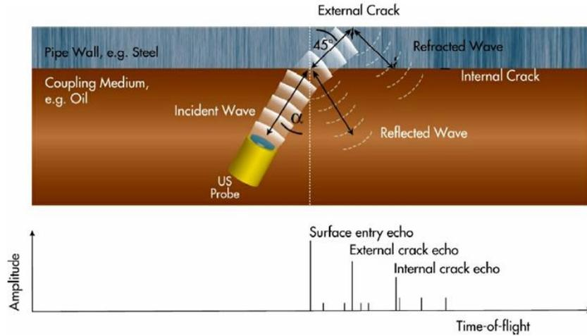
Figure 2.11. Ultra-sonic Inspection for Cracks (www.ppsa-online.com)
