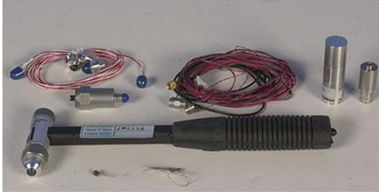
Figure 2.10. Impulse Hammer and Accelerometers (www.used-line.com)
