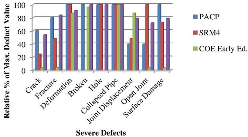
Figure 3.7. Comparison of Deduct Values for Severe Structural Defects for All Four Protocols
