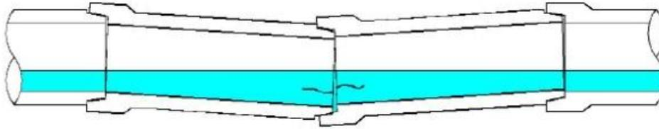
Figure 3.3. Moderate sag with displaced joint/open joints (SRM, 2001)
