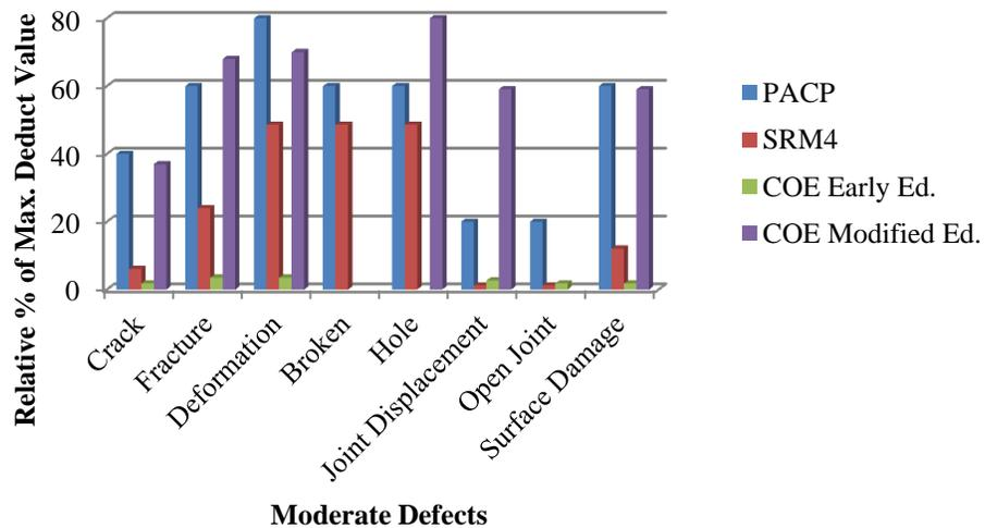
Figure 3.6. Comparison of Deduct Values for Moderate Structural Defects for All Four Protocols
