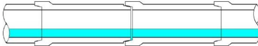
Figure 3.2. Early stage of sag, presence of gap at the middle joint (SRM, 2001)
