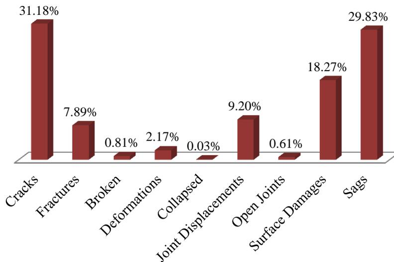
Figure 5.2. Percentages of Defect Counts per Category of Structural Defects
