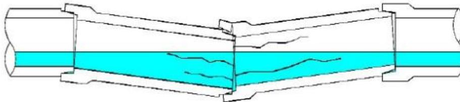
Figure 3.4. Deformations and fractures present at improved stages of sag (WRc 2001)
