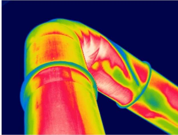
Figure 2.12. Infrared Thermography Inspection ([www.maverickinspection.com](http://www.maverickinspection.com))
