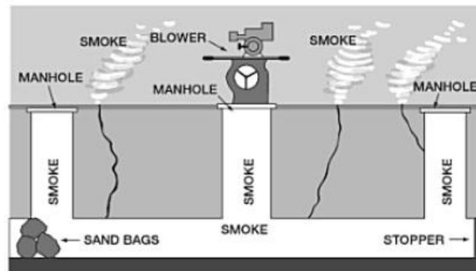
Figure 2.8. Smoke Testing (Water Environment Federation, 2009)
