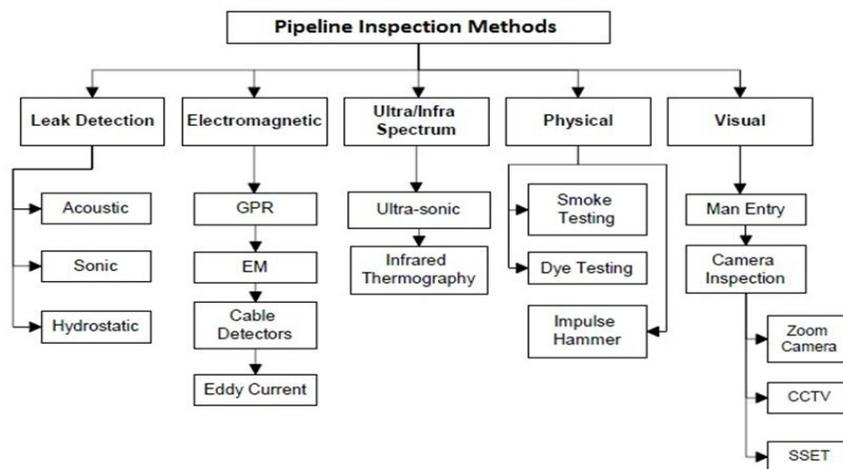
Figure 2.7. Pipeline Inspection Methods (Allouche and Freure, 2002)
