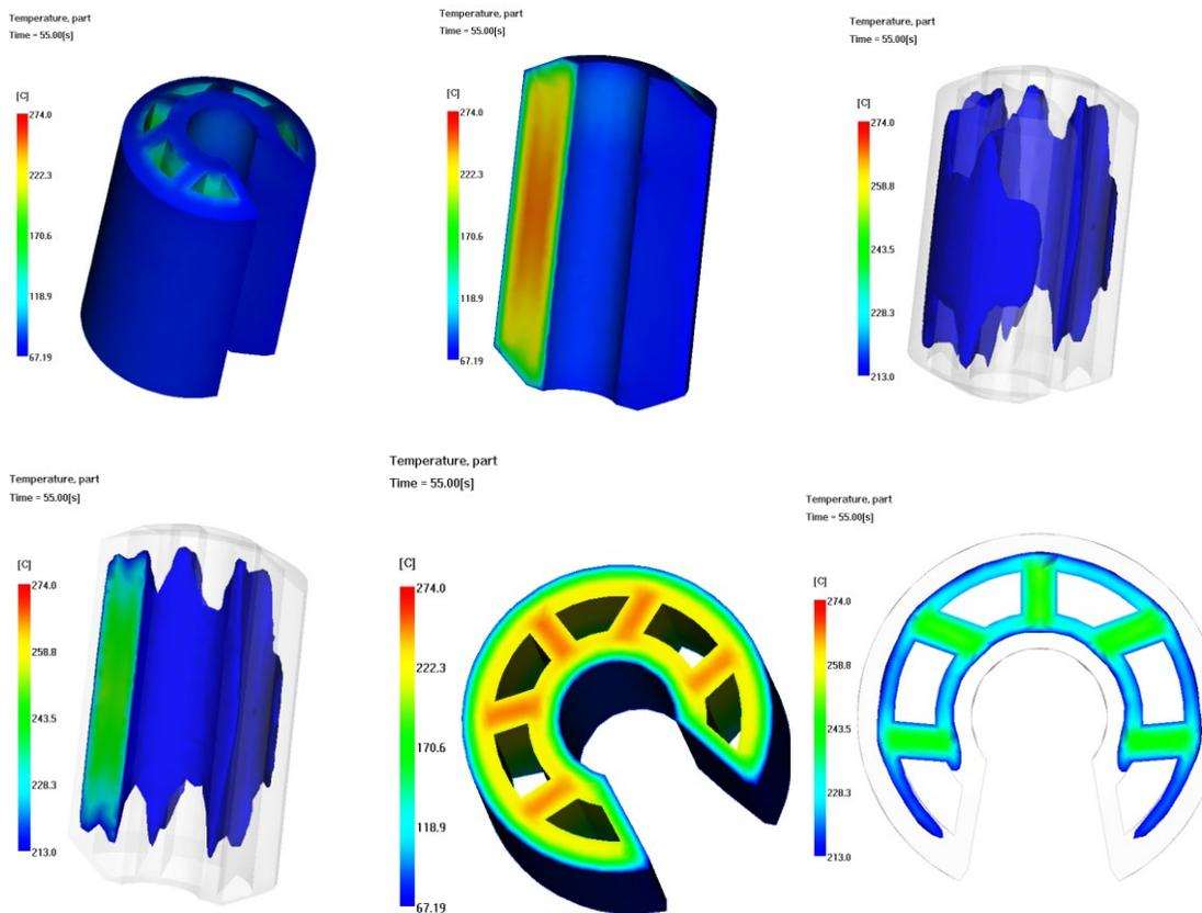
Figure 4.8 Tough grip interior temperature result
