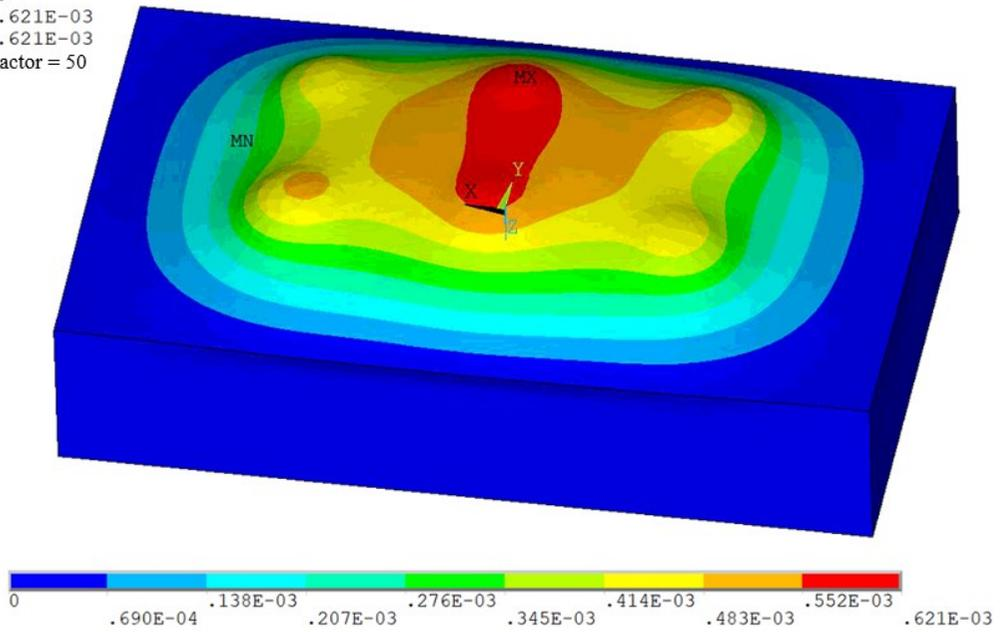
Figure 6.6 Ejection-induced plastic deformation for box product
