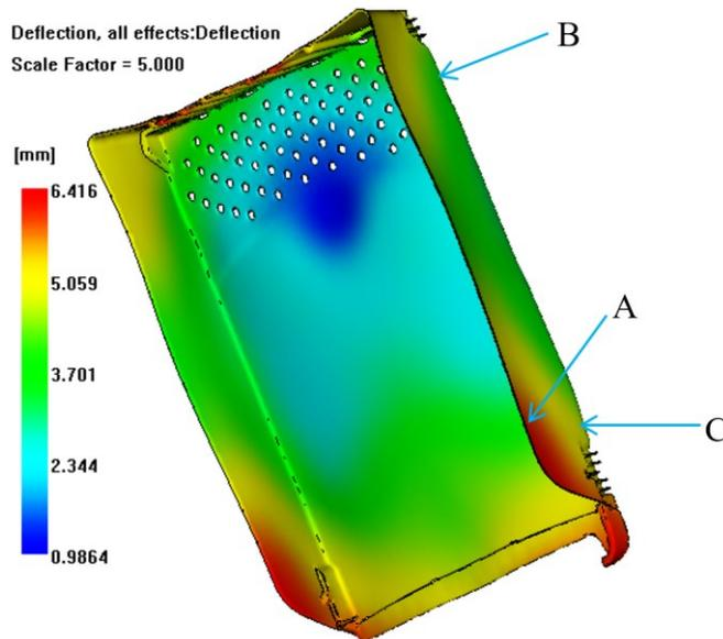
Figure 3.19 Warpage of Tray after adding more cooling (simulation)
