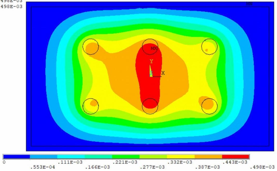
Figure 6.9 Ejection-induced plastic deformation for box product at 49s
