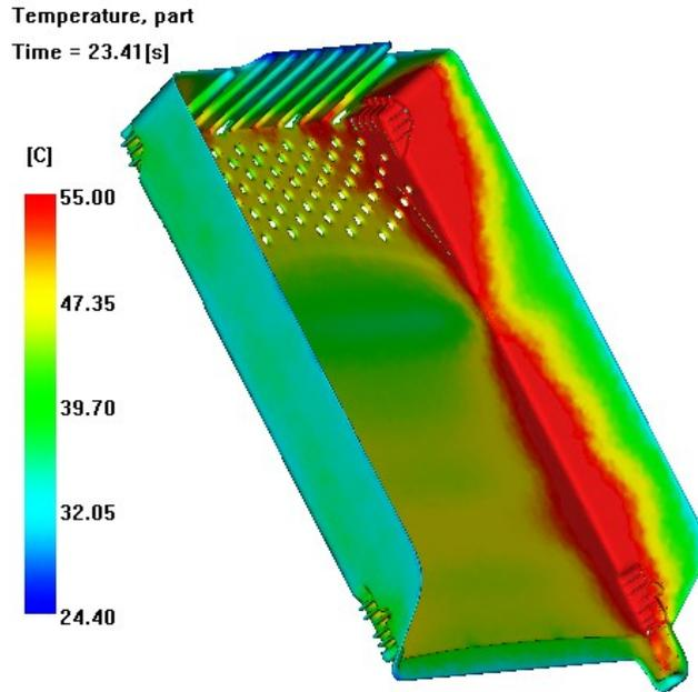
Figure 3.17 Temperature distribution of Tray (initial simulation)
