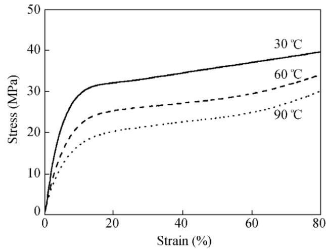
Figure 4.1 Temperature dependent stress-strain curves for PA (Guo, et al., 2015)
