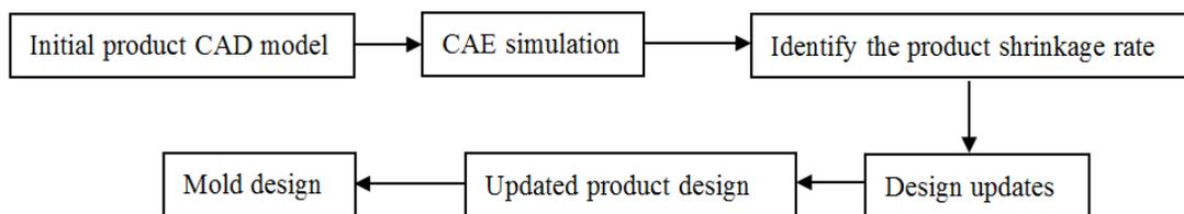
Figure 1.4 Ideal mold design workflow
