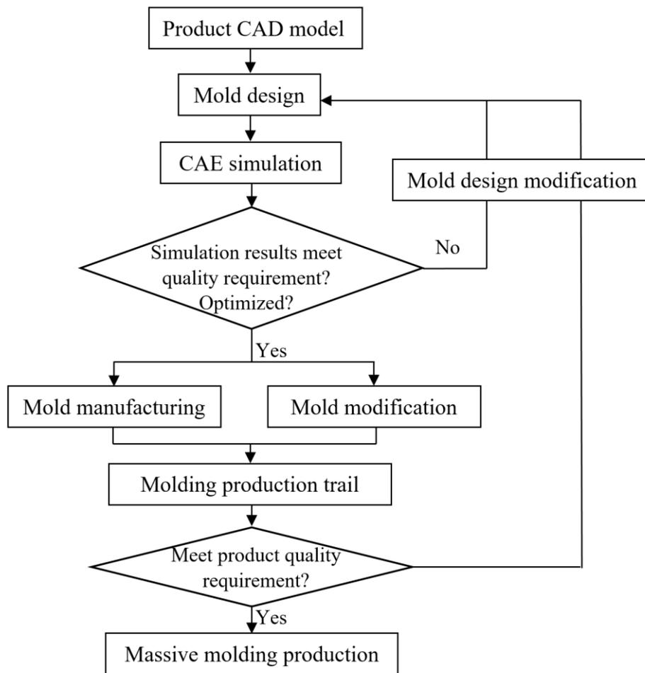
Figure 1.3 Industrial mold design workflow
