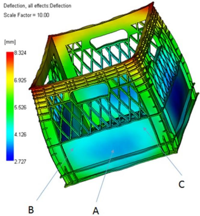
Figure 3.13 Warpage of Milkcrate with changed side inserts (simulation)
