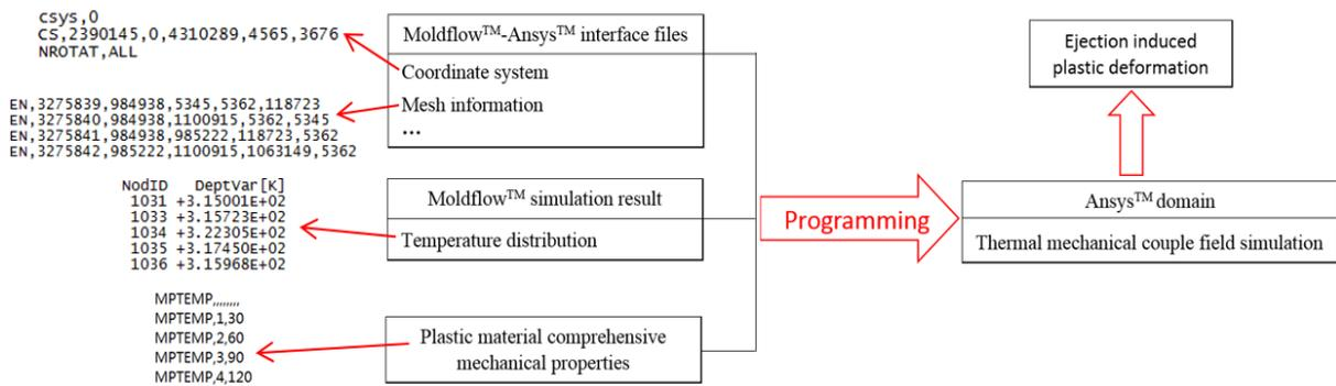
Figure 4.3 Information integration model for ejection simulation
