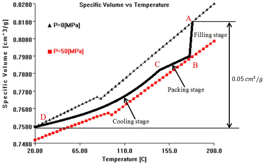
Figure 3.4 PVT curve of generic shrinkage characterized PVC (Moldflow material library)
