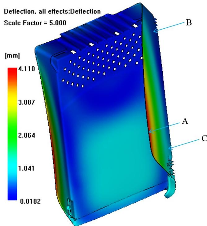
Figure 3.20 Warpage of Tray with PVC (simulation)
