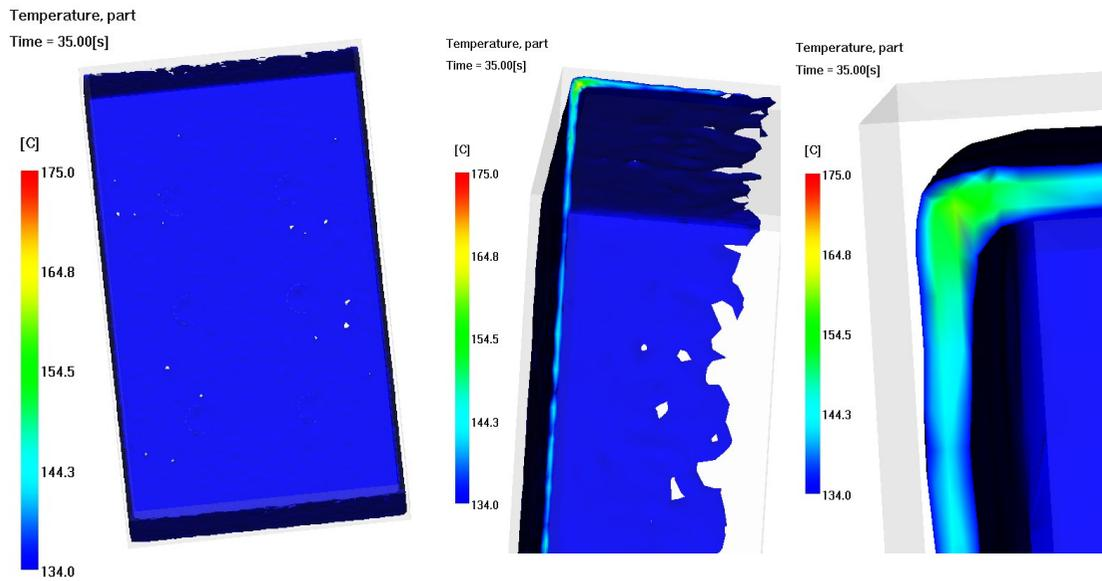
Figure 6.5 Box product interior temperature result
