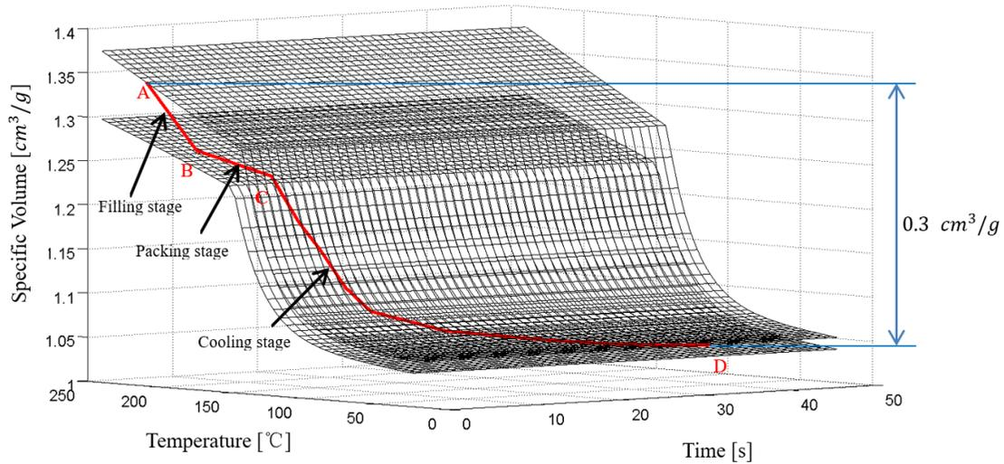
Figure 3.3 3D specific volume curve of typical HDPE
