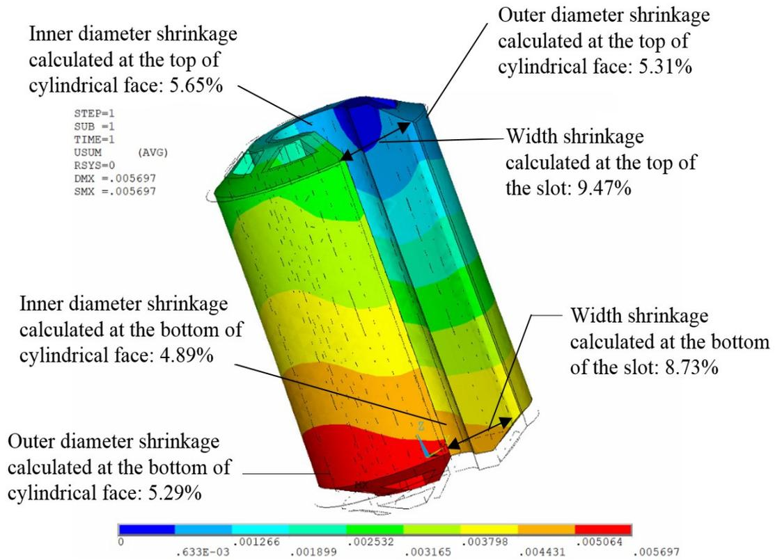
Figure 5.5 Deformation of tough grip with in-mold cooling and air-cooling
