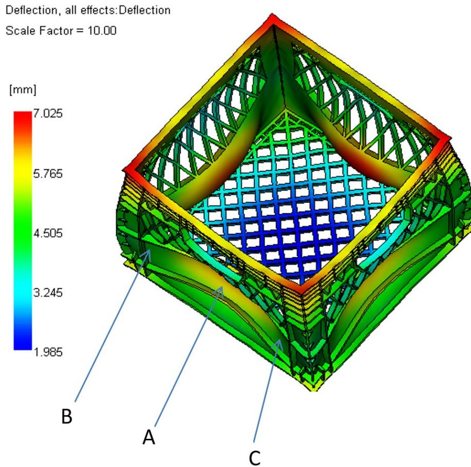
Figure 3.8 Warpage of Milkcrate (initial simulation)
