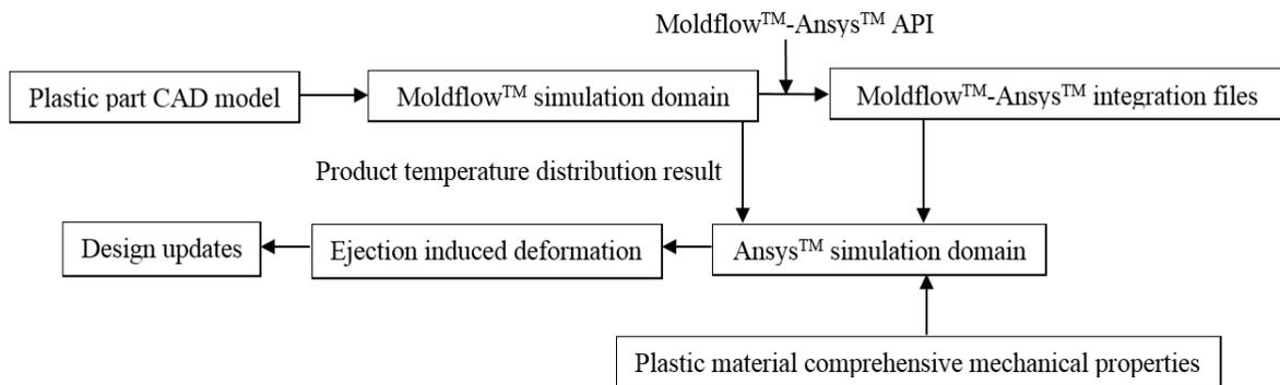
Figure 4.2 Schematic of the proposed approach for ejection simulation
