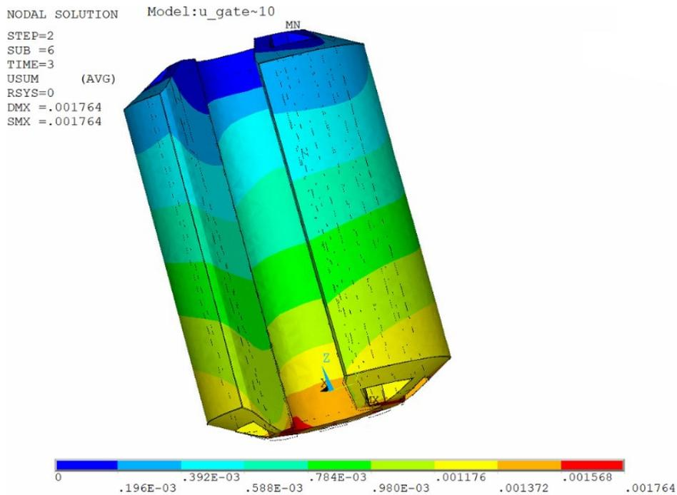
Figure 4.9 Ejection-induced deformation for tough grip
