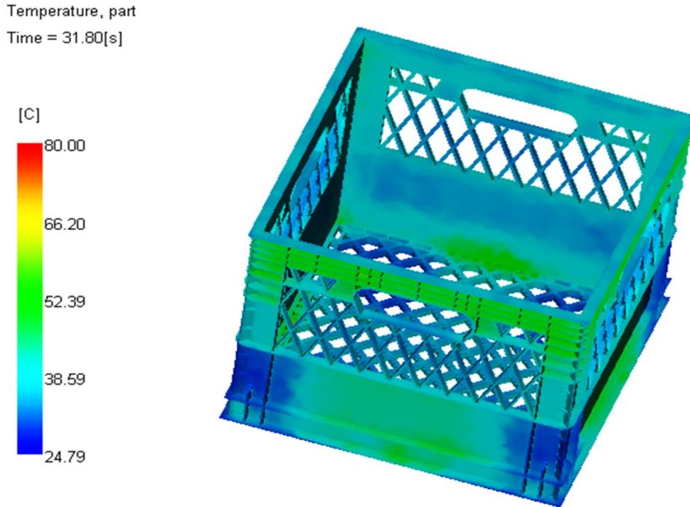
Figure 3.9 Temperature distribution of Milkcrate (initial simulation)
