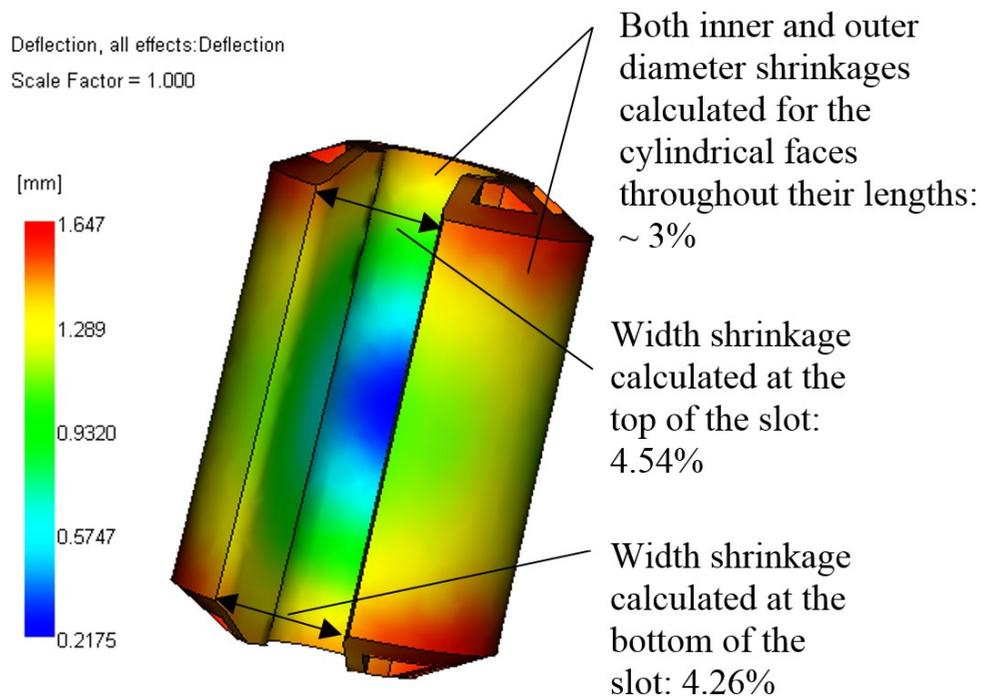
Figure 4.6 Moldflow deflection simulation result for tough grip
