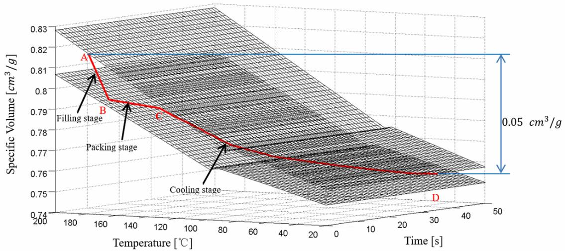
Figure 3.5 3D specific volume curve of typical PVC
