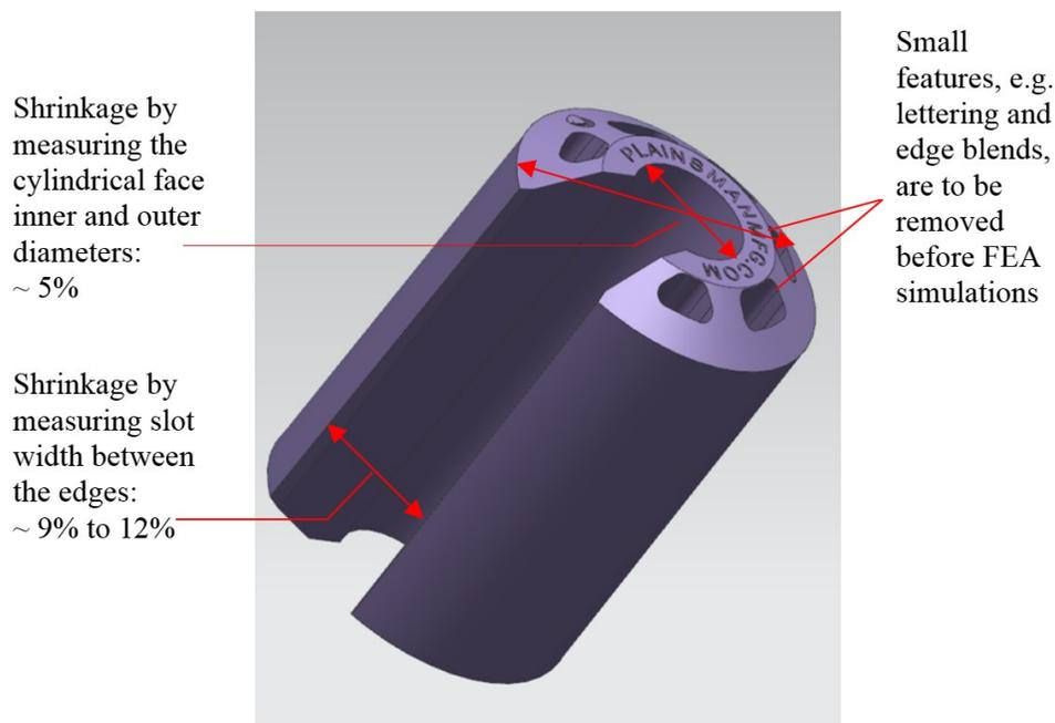
Figure 4.4 Original 3D CAD model of tough grip
