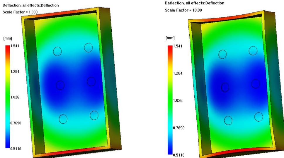
Figure 6.3 Moldflow deflection simulation result for box product
