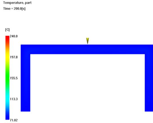
(b) Temperature distribution simulation result for case a
