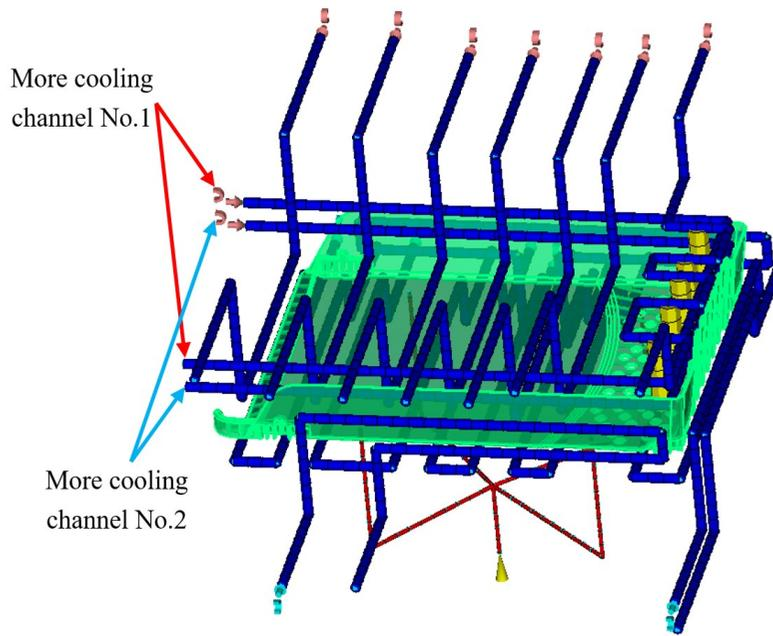
Figure 3.18 Mold configuration of Tray (more cooling channels)
