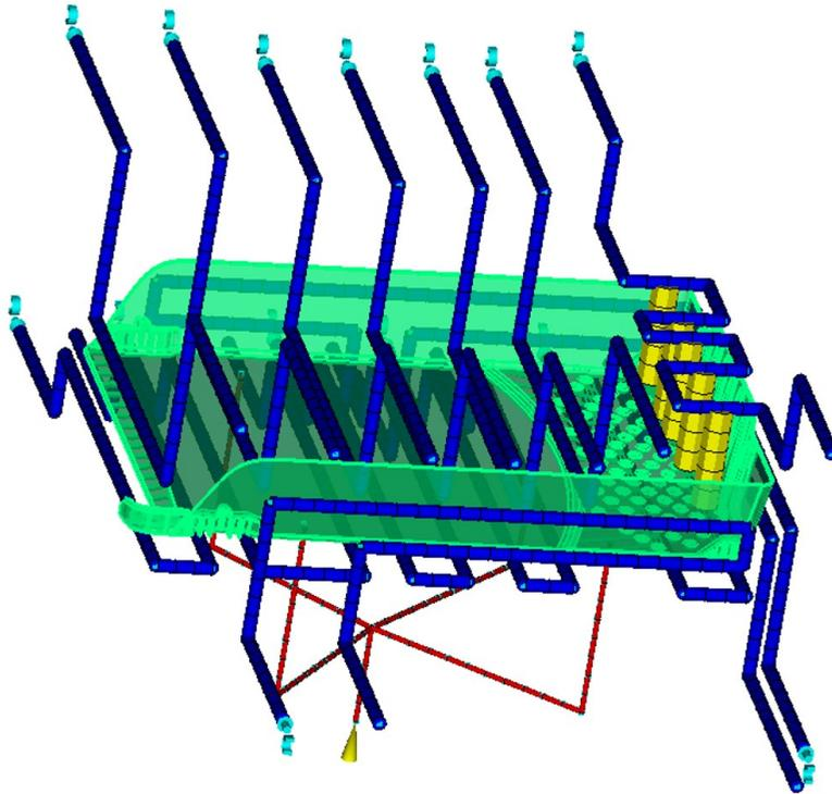
Figure 3.15 Mold configuration of Tray
