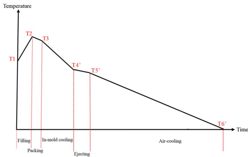
Figure 5.2 Temperature history of the proposed early-ejected injection molding product
