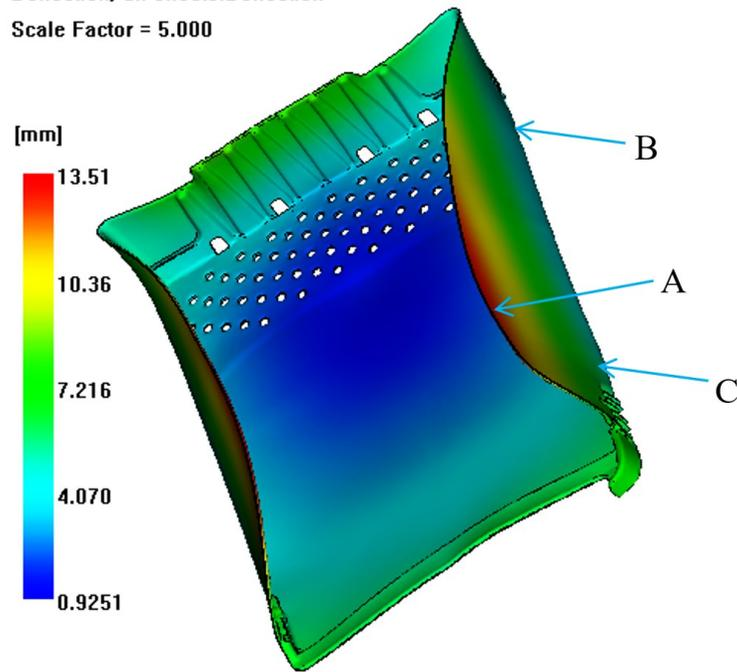
Figure 3.16 Warpage of Tray (initial simulation)
