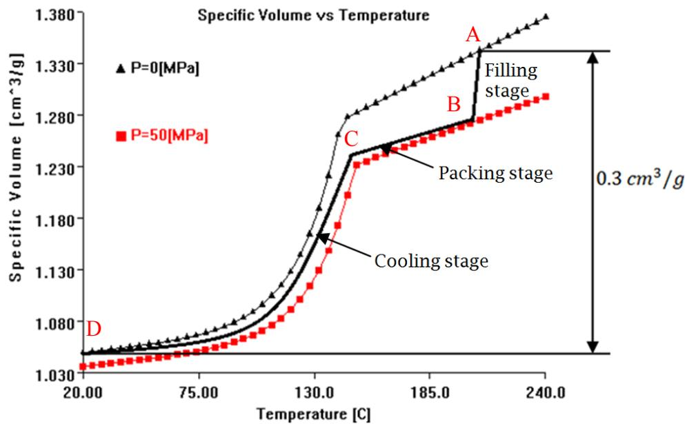
Figure 3.2 PVT curve of HDPE under different pressures (Moldflow material library)
