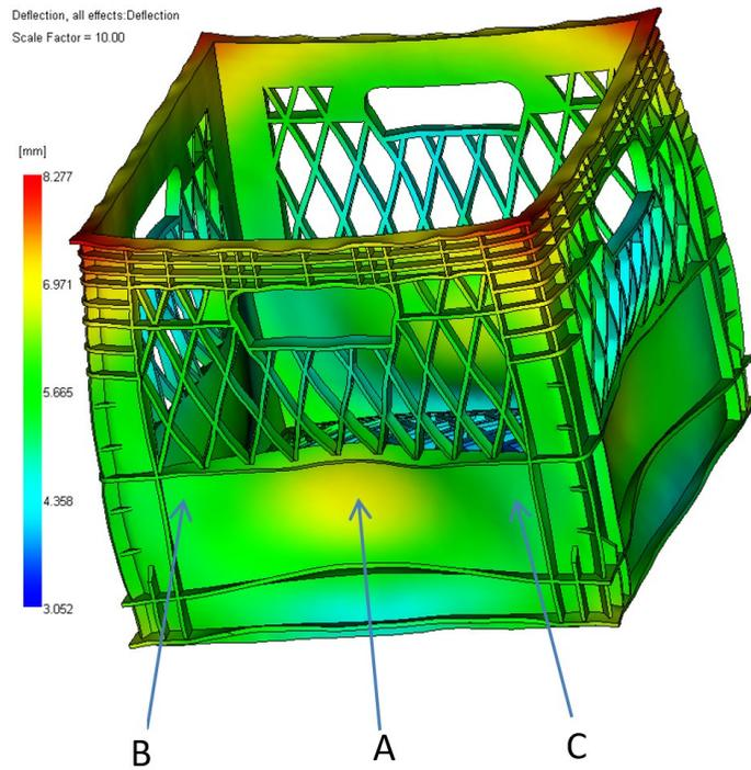
Figure 3.11 Warpage of Milkcrate with the enhanced cooling channels (simulation)
