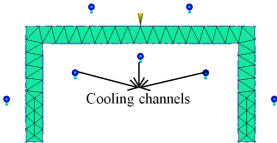
(e) Practical mold design with cooling channels in both cavity and core side
