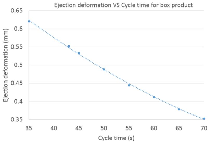
Figure 6.8 Deformation of box product with in-mold cooling and air-cooling
