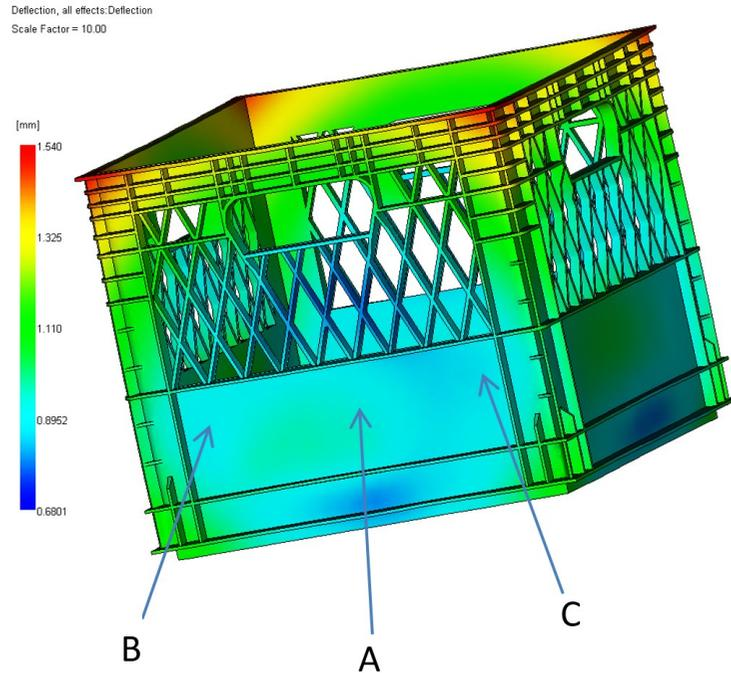
Figure 3.12 Warpage of Milkcrate with PVC (simulation)
