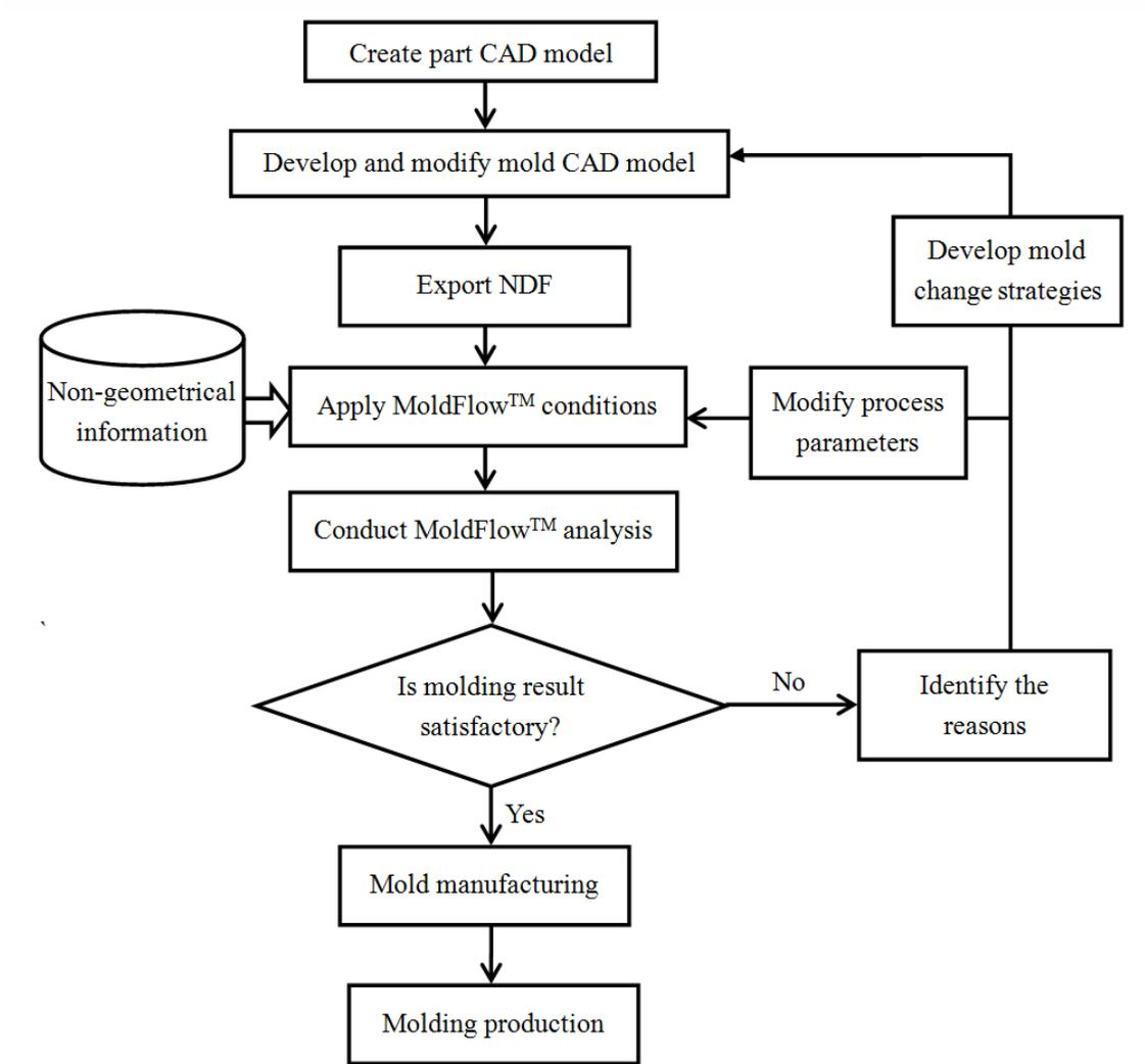
Figure 3.1 Proposed workflow addressing warpage after the mold made
