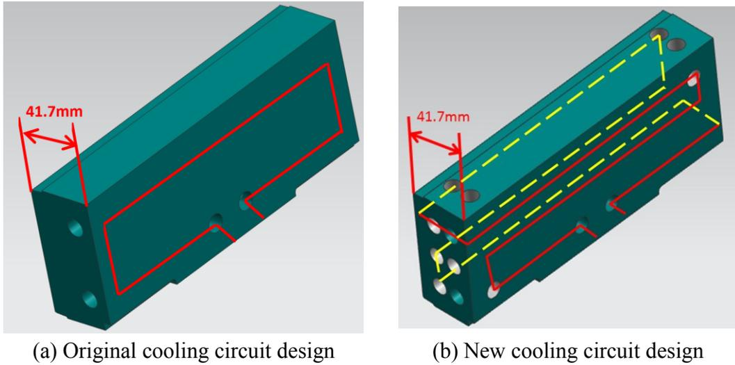
Figure 3.10 Original and new design of the cooling circuit for side insert
