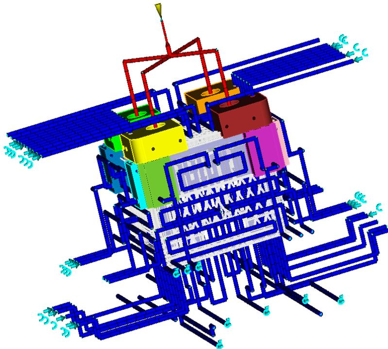
Figure 3.7 Mold configuration of Milkcrate
