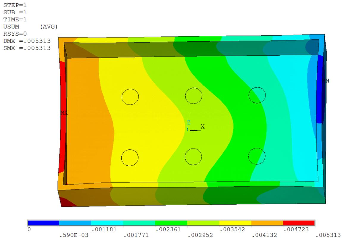
Figure 6.7 Deformation of box product with in-mold cooling and air-cooling
