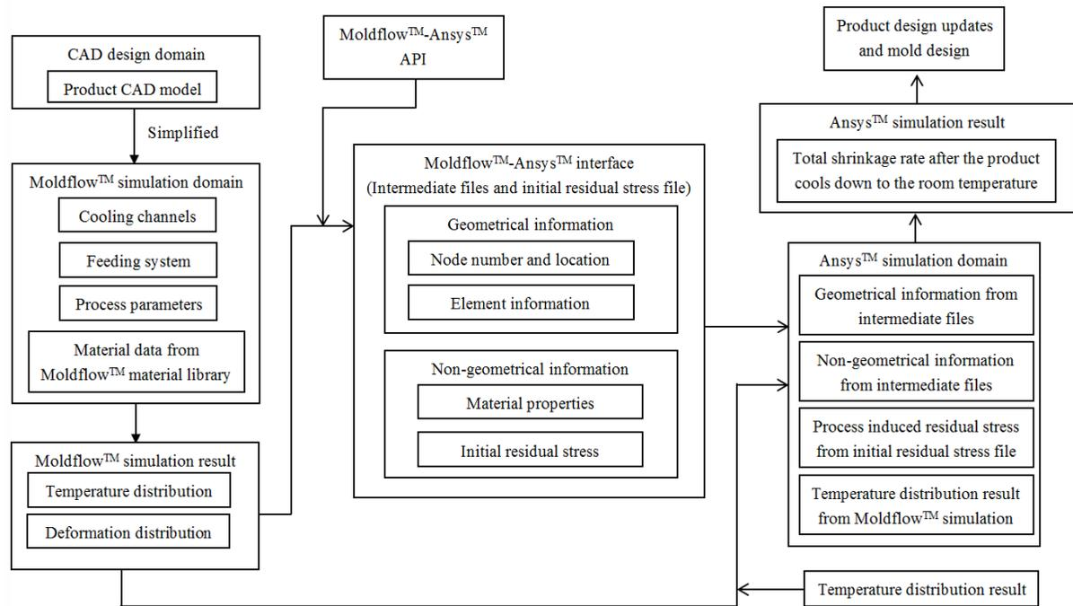
Figure 5.4 Schematic of the proposed approach for air-cooling simulation
