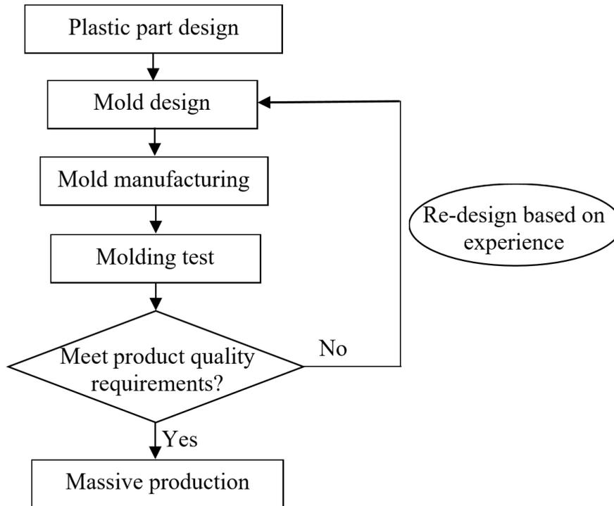
Figure 1.2 Traditional mold design process
