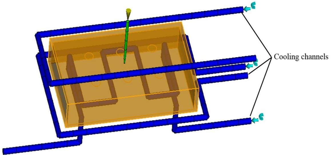
Figure 6.2 Mold configuration for box product
