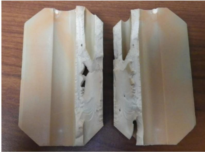
Figure 7.1 Failure example of a tough grip
