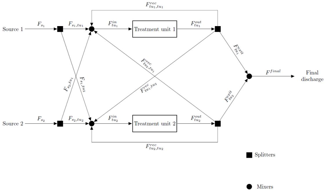
Figure 2.1: Schematic representation of the small water treatment model
