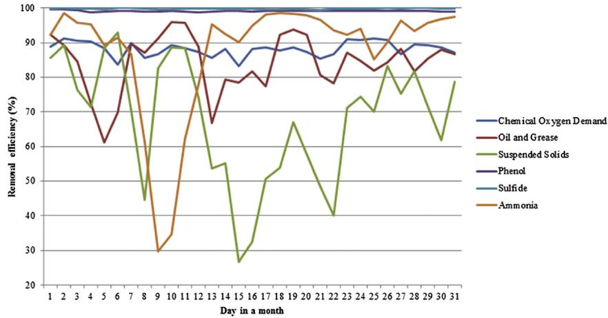
Figure 1.2: Variation in the contaminant removal efficiency of a reverse osmosis unit over a one-month period
