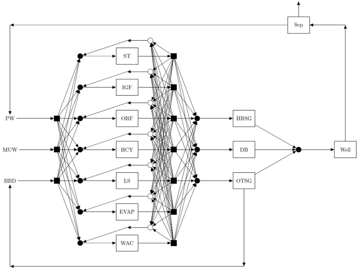
Figure 5.1: Superstructure of the SAGD effluent treatment and steam generation network
