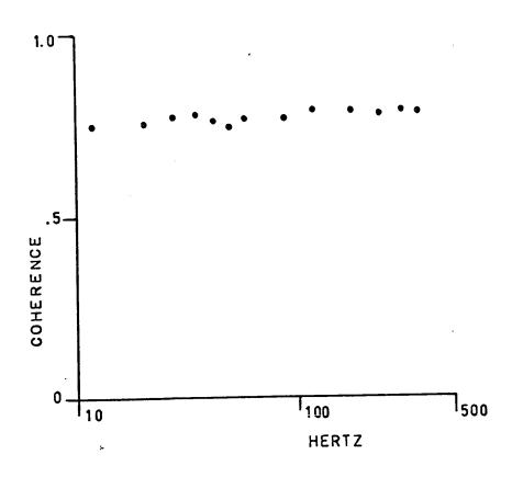
Figure 4.10 . Estimate of the coherence function of a Germanium diode .
