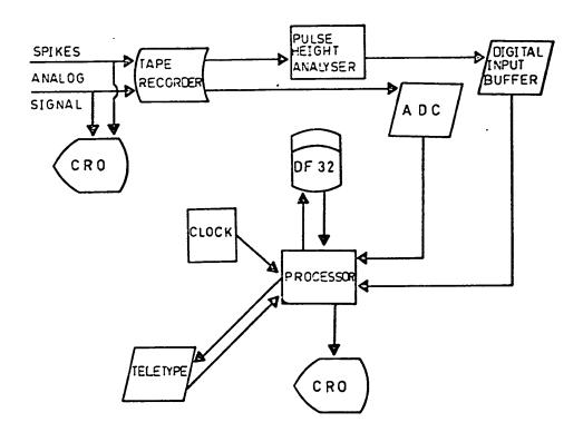
Figure 3.1 . Principal information flow-paths of data processing system .
