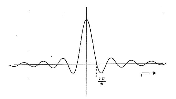
Figure 3.3 . Fourier Transform of rectangular lag window .
