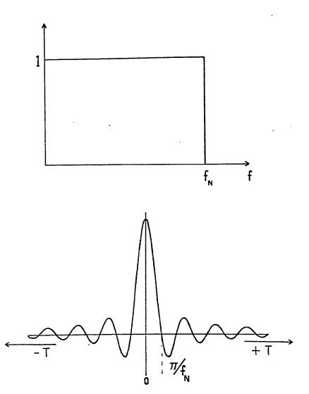
Figure 3.4 . Ideal , rectangular low-pass filter and its impulse response .
