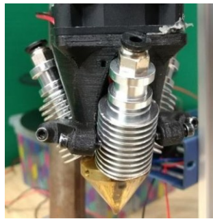
Figure 4.2 Mixing nozzle hotend (three inputs and one output)
