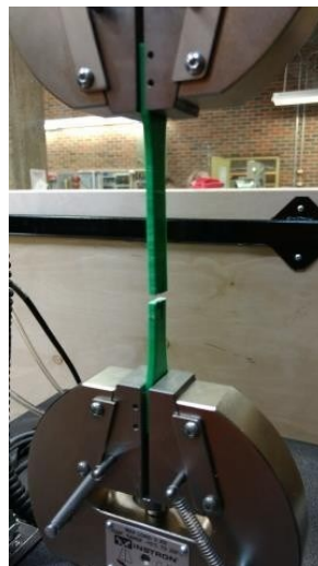
Figure 4.7 Specimen ABS positioned and tested in the tensile machine
