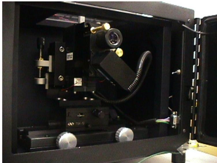
Figure C.3: The  $\mu$ TK optics module. The observation heart of the  $\mu$ TK is the epiluminescent confocal microscope which induces and captures laser induced fluorescence detection by exciting TAMRA dye via a 532 nm laser (schematic and image courtesy of MicraLyne Inc.).
