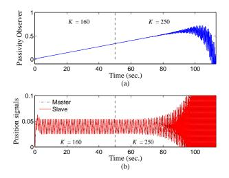
Figure 3.4: Passivity observer output in simulations for a teleoperator with a changing controller gain. The controller gain changes from K = 160 to K = 250 at  $t = 50^{\text{sec}}$  and makes the teleoperator non-passive. The other system parameters are  $T = 5^{\text{ms}}$ , b = 1 and B = 0.
