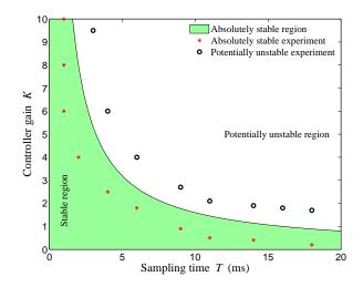
Figure 4.6: The theoretical absolute stability region in K - T plane versus experimental data points obtained from a sampled-data teleoperator with  $n_c = n_p = 3$ .
