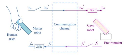
Figure 2.3: The operator is indenting a soft object remotely and receives force feedback
