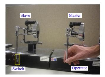
Figure 4.10: The experimental setup for flipping the three-way slide switch.
