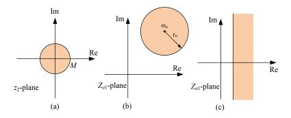
Figure 5.9: (a) a disc in the  $z_2$ -plane inside  $\mathcal{C}(M,0)$ , (b) if  $|Z_{22}| \neq M$ , the mapped region is also a disc in the  $Z_{a1}$ -plane, (c) if  $|Z_{22}| = M$ , the mapped region is a shifted RHP.
