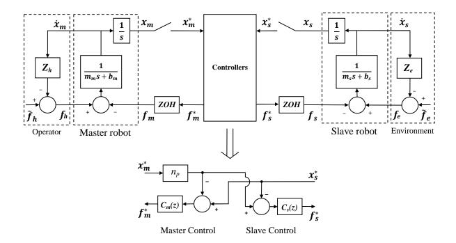
Figure 3.2: The block diagrams of a teleoperation system, which includes discretized controller models.
