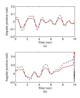
Figure 5.15: Master-slave positions for an ISP environment in DFR teleoperation with (a) a DFR(P+D) controller, and (b) a DFR(PD) controller.
