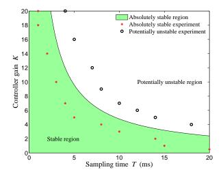
Figure 4.5: The theoretical absolute stability region in K - T plane versus experimental data points obtained from a sampled-data teleoperator with  $n_c = n_p = 1$ .
