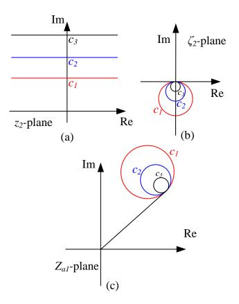
Figure 5.6: The horizontal lines in the  $z_2$ -plane are transformed into circles in the  $Z_{a1}$ -plane. As the horizontal line moves up, the radius of the circles decreases. Yet, all of the circles are tangent at one point.
