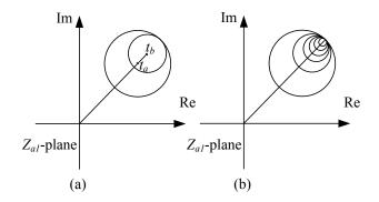
Figure 5.5: The vertical lines in the  $z_2$ -plane are mapped to circles in the  $Z_{a1}$ -plane. The vertical line at  $\operatorname{Re} z_2 = -a$  is mapped to the larger circle in the  $Z_{a1}$ -plane while the vertical line at  $\operatorname{Re} z_2 = b$  is mapped to the smaller circle (a). As the real value of  $z_2$  is allowed to increase (i.e., larger b), the radius of the smaller circle decreases while the circles still share the same tangent point.
