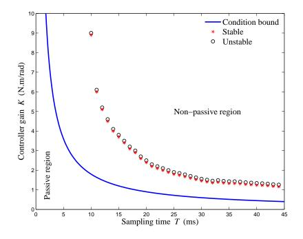
Figure 3.7: Free-motion/clamped (FC) experiment data points and theoretical passivity borderline. Stars represent stable, and circles represent unstable systems.
