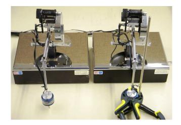
Figure 3.5: Experimental setup for the case where the master arm (left) is in free motion and the slave arm (right) is clamped (FC).
