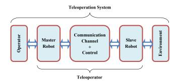
Figure 2.1: The teleoperation system versus the teleoperator.
