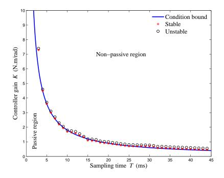
Figure 3.6: Free-motion/free-motion (FF) experiment data points and theoretical passivity borderline. Stars represent stable, and circles represent unstable systems.
