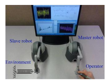
Figure 4.4: Experimental setup – The master arm is controlled by the human operator and the slave arm interacts with its environment.
