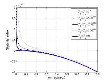
Figure 4.3: Stability index vs. time delay when the controller gain K = 800. As long as the delays satisfy (4.25), the stability index remains negative (i.e., the teleoperation system remains absolutely stable).
