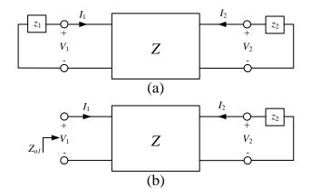
Figure 5.1: (a) A two-port network connected to two one-port network terminations, and (b) the driving-point impedance at port 1,  $Z_{a1} = V_1/I_1$ , when port 2 is terminated to a passive impedance  $z_2$ .
