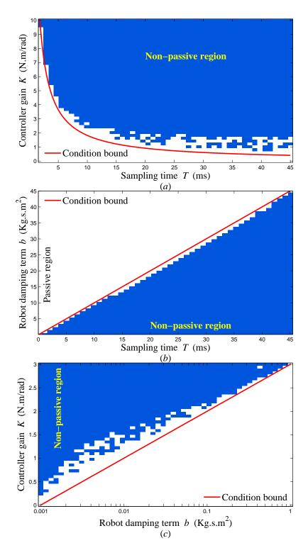
Figure 3.3: Passive and non-passive regions (a) in K - T plane for B = 0 m = 0.015 and b = 0.01822, (b) in b - T plane for K = 1, m = 0.015 and B = 0, and (c) in K - b plane for B = 0, m = 0.015 and  $T = 1^{\text{ms}}$ .
