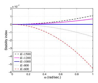
Figure 4.2: Stability index vs. the controller gain when the delays  $T_1 = T_2 = 0$ . As long as the controller gain K satisfies (4.37), which is K < 1000, the stability index remains negative (i.e., the teleoperation system remains absolutely stable).
