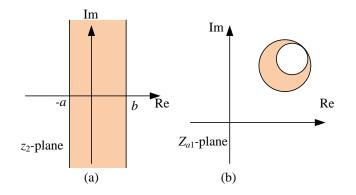
Figure 5.4: In analysis of the strip-like impedances the strip in the  $z_2$ -plane (a) is mapped to a rotated crescent in the  $Z_{a1}$ -plane (b).
