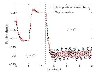
Figure 4.8: The position of the master and slave. The sampling time is  $T = 2^{\text{ms}}$  in  $0 < t \le 2.35^{ms}$  and  $T = 6^{\text{ms}}$  in  $2.35 < t < 6^{ms}$ .
