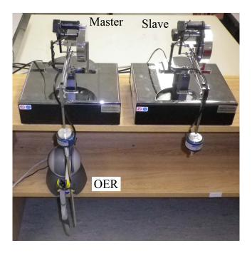
Figure 5.16: An OER is used as a human operator in a bilateral teleoperation systems.
