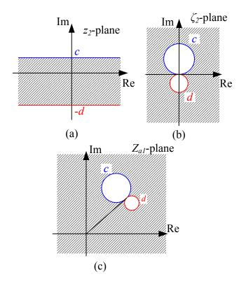
Figure 5.7: The area between the two horizontal lines in the  $z_2$ -plane are transformed into the hatched area in  $Z_{a1}$ -plane.
