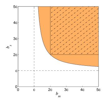
Figure 4.1: Absolute stability and passivity regions in the plane of the master robot damping  $b_m$  versus the slave robot damping  $b_s$ . Blue shows the absolute stability region and hatched corresponds to the passivity region and c is the right hand side of (4.37).
