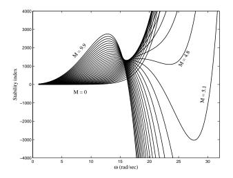
Figure 5.11: The stability index is evaluated for different values of the disc radius for a range of frequencies.
