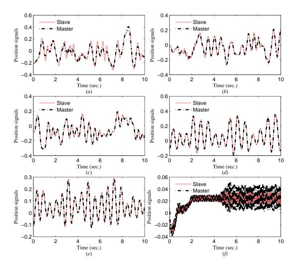
Figure 4.7: The positions of the master and the slave when the operator moved the master and the slave was in free space. The proportional controller gain was K = 0.5, K = 1.5, K = 2.5, K = 3, K = 3.5 and K = 4.5 for parts (a) to (f), respectively. The means of absolute value of the tracking errors are  $2.20 \times 10^{-3}$ ,  $1.59 \times 10^{-4}$ ,  $2.86 \times 10^{-5}$ ,  $2.43 \times 10^{-5}$ ,  $1.22 \times 10^{-5}$  and  $2.59 \times 10^{-4}$  rad, respectively.
