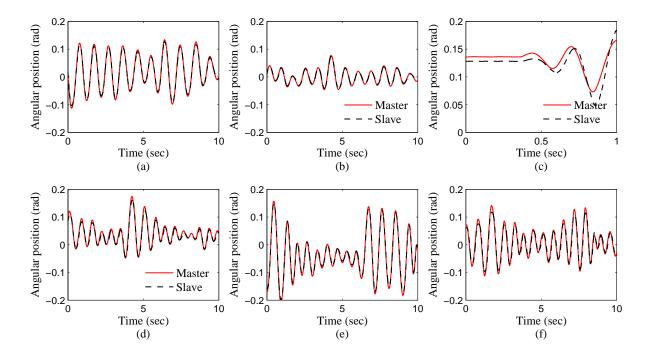
Figure 5.14: Master-slave positions for strictly-passive environment with PEB architecture. Top row has  $\tau_y = 0$  and and bottom row has torque of  $\tau_y = 0.2$  N.m. The controller gains are given in Table 5.5.
