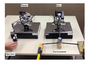
Figure 5.13: The experimental setup for testing ISP environment.
