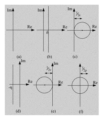
Figure 5.2: Nyquist diagrams of (a) a passive system, (b) an ISP system with EOP of  $\delta$ , (c) an OSP system with EOP of  $\epsilon$ , (d) an INP system with SOP of  $\eta$ , (e) an ONP system with SOP of v, (f) a DNP system with SOP of  $\rho$ .
