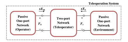
Figure 3.1: The passivity of the teleoperation system is guaranteed when a two-port network teleoperator is passive and is connected to two passive one-port network terminations.
