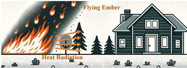
Figure 2.10: Visualization of wildfire transfer from ember and radiation. Image generated by DALL-E, OpenAI, 2024
