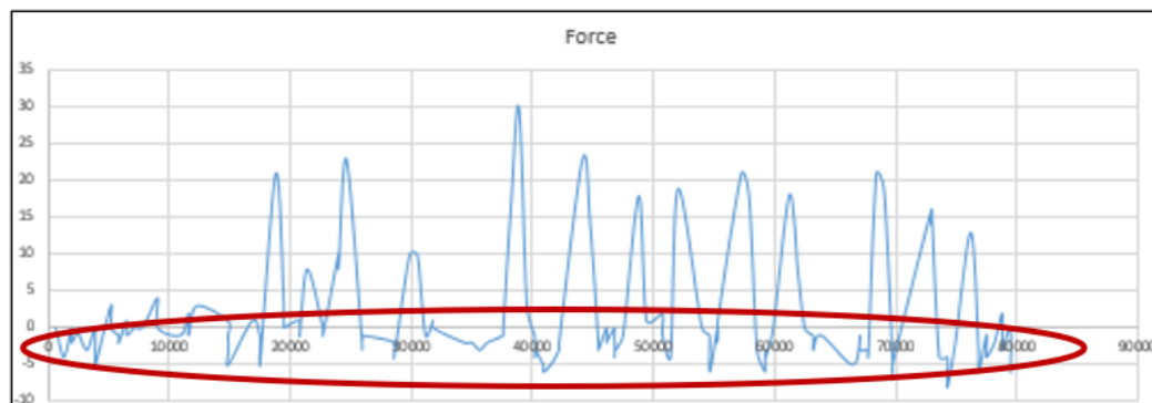
Figure 4. Negative force output values (< 0 Newtons) circled in red obtained from preliminary testing of the TONE device on August 11 th 2021.
