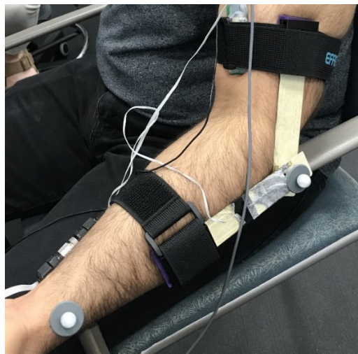
Figure 2. Electronic goniometer aligned with anatomical landmarks for obtaining kinematic measures of elbow flexion and extension. *Note marker placement for joint axis on top of electronic goniometer to enable simultaneous OptiTrack Trio system and TONE device measurements.
