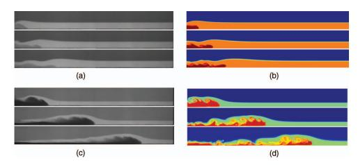
FIG. 2. (Color online) Flow evolution in a complementary pair of experiments (panels (a) and (c)) and numerical simulations (panels (b) and (d)). In the top and bottom row, respectively, images measure  $176 \text{ cm} \times 20 \text{ cm}$  and  $178 \text{ cm} \times 20 \text{ cm}$ . Further experimental and numerical parameters are summarized in the text.
