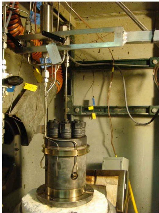
Fig A6: Correct configuration of the view cell
