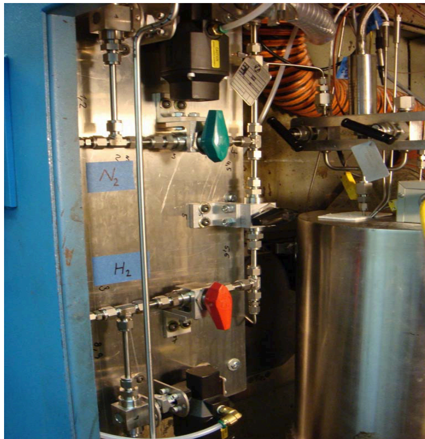
Fig A1: Closed valves configuration at the start of the experiment
