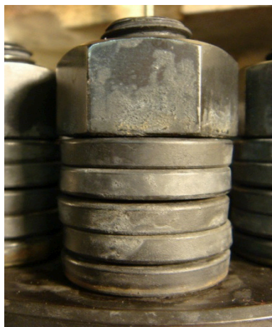
Fig A4: Correct configuration of washers
