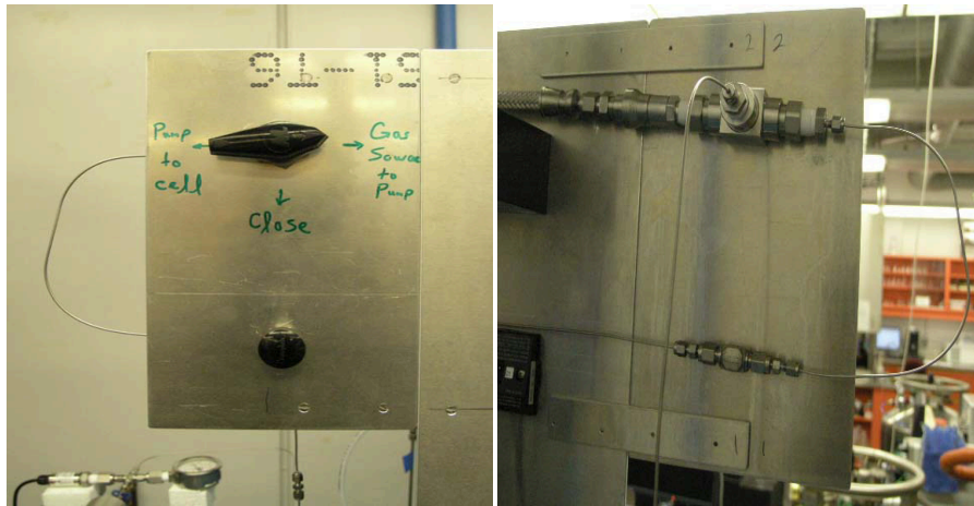
Figure 16: Front (photo on the left) and Rear (photo on the left) view of the Injection System Control Panel
