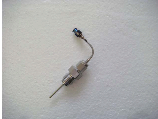
Fig A9: Sampling device which can be attached to a syringe
