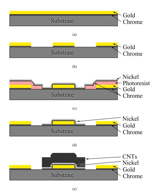
Figure A.1: Process flow for the carbon nanotube test substrate showing cross-sections at key process steps.
