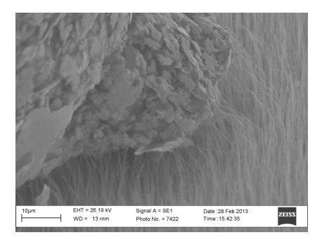
Figure 5.7: CNT adhesion to silver epoxy.
