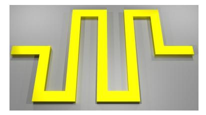
Figure 2.4: Two-turn meander inductor
