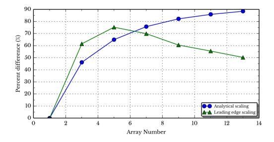
Figure 3.32: Percent difference between the analytical inductor scaling models and the simulated inductor scaling behaviour.
