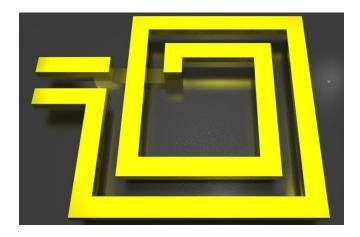
Figure 2.3: Two-turn square-spiral planar inductor. Note that the inner turn is connected to the outer terminal by a set of vias and a wire on a second layer.
