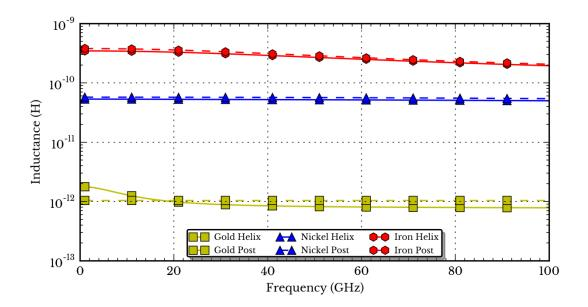
Figure 3.9: Comparison of the inductance of the wide helix and the equivalent linear wire.
