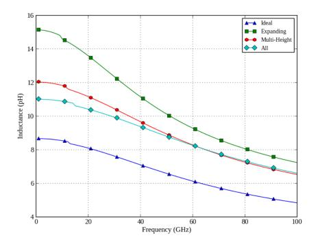
Figure 3.34: Inductance of a  $7 \times 7$  helix array with defects added.
