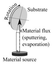
Figure 4.1: Glancing angle deposition setup.
