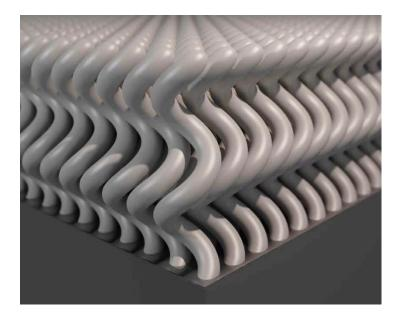
Figure 2.6: Conceptual diagram of the cross section of a helical GLAD film.
