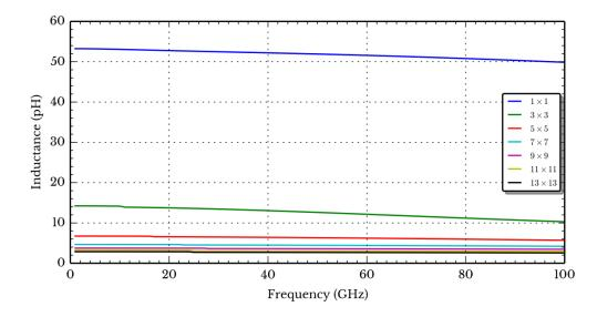
Figure 3.27: Simulated inductance of nickel helix arrays.
