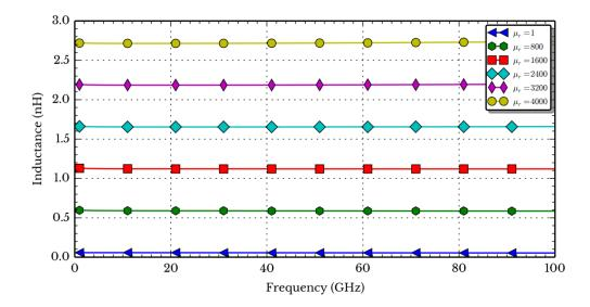
Figure 3.15: Inductance of a single helix in an ideal magnetic material.
