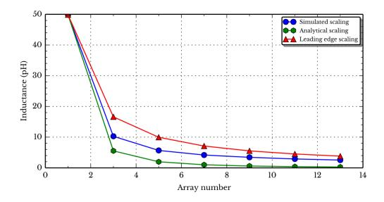
Figure 3.30: Inductance scaling of helix arrays. The array number is the number of helices along each side of the square (eg. an array number of 5 means the simulation is a 5x5 array). The inductances are simulated at 100 GHz.
