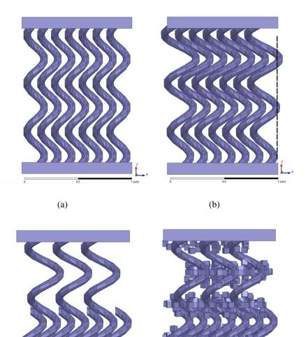
Figure 3.33: Helix width comparison. (a) An idealized helical film. (b) The same film but with a radius change of 50% between bottom and top. The radius change is emphasized by the vertical, dashed line. (c) Addition of helix termination defects to the model in (b). (d) Addition to random growth defects to the model in (c). The defects are modeled as arrays of cubes of material that are placed pseudo-randomly. This model includes all observed defects.
