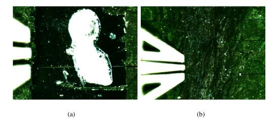
Figure 4.10: Measurement setup with: (a) silver epoxy capping layer (white), gold (green) and anisotropic film (black) and (b) with the film removed.
