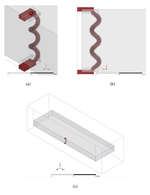
Figure 3.14: Model of a single inductor embedded in an effective medium.
