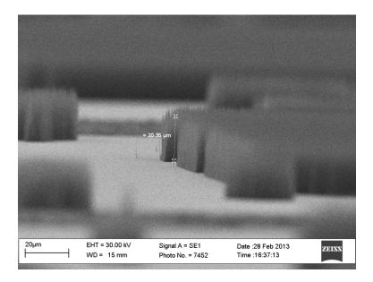
Figure 5.5: Carbon nanotube growth on substrate.
