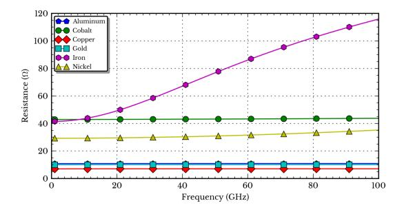
Figure 3.7: Resistance of a single wire shown in Figure 3.3 in free space.
