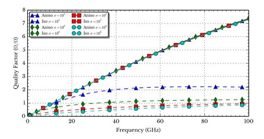
Figure 3.23: Quality factor of an anisotropic conductive film compared to the isotropic film.
