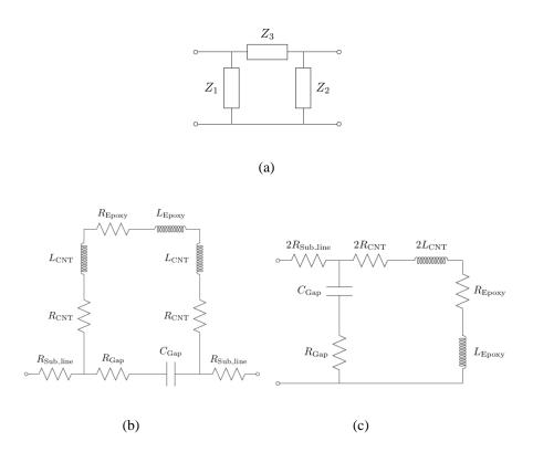
Figure 5.9: Circuit extraction models. (a) The generic  $\pi$ -model for a 2-port network. (b) An expanded model for  $Z_3$  from (a), including the capacitance of the gap and the resistance of the gold connecting traces. (c) The same model as shown in (b), with duplicate elements combined.
