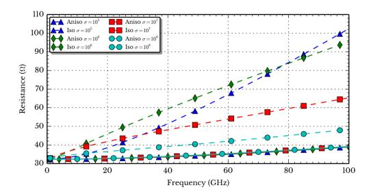
Figure 3.22: Resistance of an anisotropic conductive film compared to the isotropic film.
