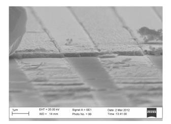
Figure 4.6: SEM image of a non-uniform section of GLAD film. The image clearly shows gaps in the film that are smaller than 2 microns (1 bar in the scale graph).
