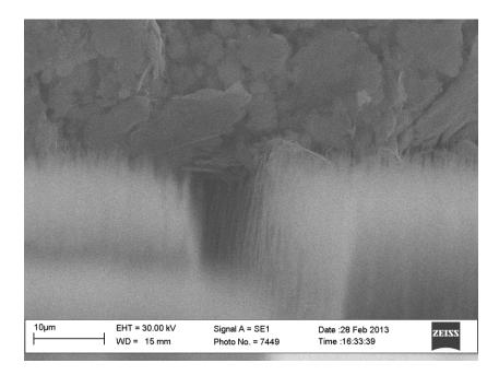
Figure 5.8: Epoxy bridge over CNT gap. The integrity of the gap between the CNTs as well as the structure of the CNTs under the silver epoxy is clearly visible.
