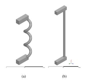
Figure 3.8: (a) Helix model shown in Figure 3.3a next to (b) its post inductor of equivalent length and wire width.
