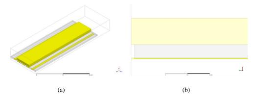
Figure 4.15: One-port simulation model of the measured chip. (a) Full structure including boundary. (b) Side view of the port and layers.
