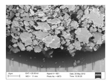
Figure 4.9: Silver particles suspended in the epoxy material.
