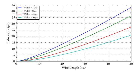
Figure 2.2: Self inductance of a single wire as a function of length. Multiple curves are shown which represent various wire widths as shown in equation 2.29.
