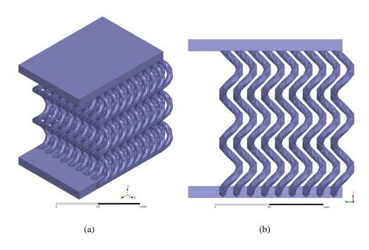
Figure 3.26: Detailed view of the **9** × **9** helix array. (a) isometric view of the helix array showing the 2dimensional square array. (b) side view of the helix array showing the top and bottom lines that connect to the port as well as the completely separated nature of the helices.
