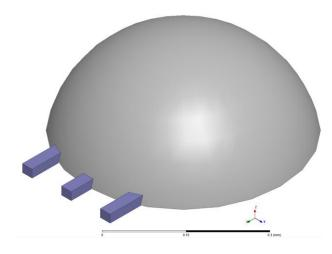
Figure 4.13: Simulation model of the silver epoxy. The blue lines on the left are the GSG probe lines which end on the surface of the silver (grey).
