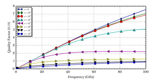
Figure 3.20: Quality factor of a single helix embedded in a conducting magnetic material ( $\mu_r = 600$ )
