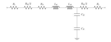
Figure 2.9: Circuit model for a short, single-wall carbon nanotube [60].  $R_c$  is the contact resistance,  $R_q$  is the quantum resistance,  $R_s$  is the scattering (ohmic-like) resistance,  $L_K$  is the kinetic inductance,  $L_M$  is the magnetic inductance,  $C_Q$  is the quantum capacitance, and  $C_E$  is the electrostatic capacitance of a CNT to ground.
