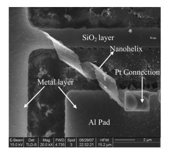
Figure 2.5: Stressed thin-film inductor © 2008 IEEE, reproduced from [38]. The original figure text: SEM image of a suspended two-turn nanohelix aluminum inductor fabricated using FIB-SIT. The inductor with an air-core is 2  $\mu$ m higher [sic] above [the] silicon substrate and is isolated from the substrate through a silicon dioxide layer between the metal layer and the substrate.
