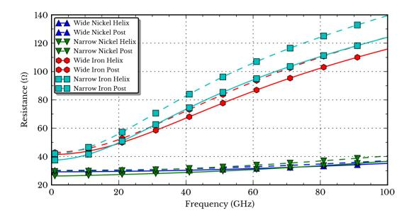
Figure 3.13: Comparison of the resistance of wide and narrow helices and the equivelent length of a straight wire.
