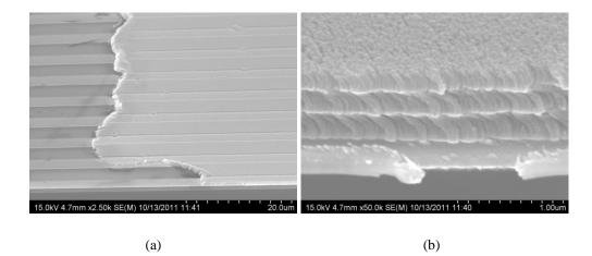
Figure 4.3: Fabricated nickel film. (a) A portion of the GLAD film with good uniformity. (b) A close-up view of the nano-structure of the film featuring the closely-packed helices.
