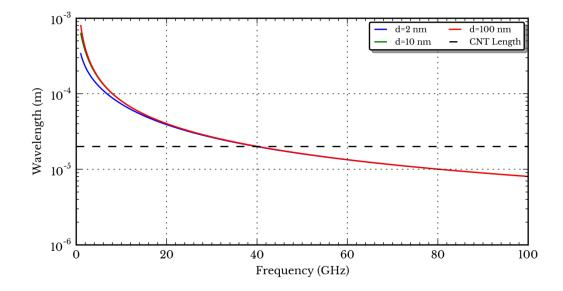
Figure 5.1: Wavelength of a SWCNT of varying diameters and 20 um in length. As the frequency increases, the CNT length becomes close to the wavelength and the CNT length is equal to the wavelength around 40 GHz. This ultra-short wavelength for a CNT transmission line causes even short CNT devices to act as distributed elements.
