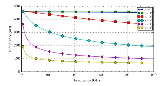
Figure 3.18: Inductance of a single helix embedded in a conducting magnetic material ( $\mu_r = 600$ )
