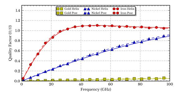
Figure 3.10: Comparison of the quality factor of the wide helix and the equivalent wire.
