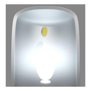
Figure 2.7: Set-up to perform glancing angle deposition with a sputtering system.
