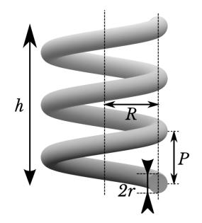
Figure B.1: Parameters of a helix; h is the helix height, R is the helix radius, r is the radius of the wire, and P is the helix pitch.
