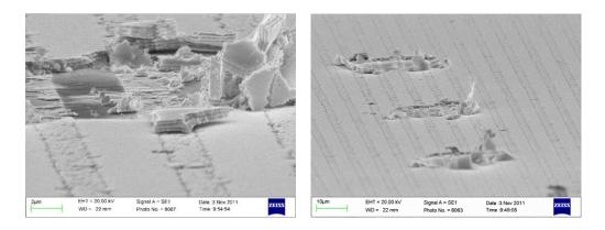
Figure 4.5: SEM image of damage to the GLAD film due to direct contact with the RF probe.
