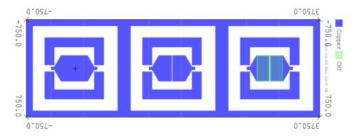
Figure 5.4: CNT test structures (short, open, CNT)
