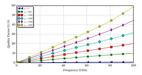
Figure 3.16: Quality factor of a single helix in an ideal magnetic material.
