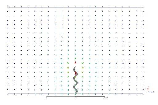
Figure 3.4: Wave port excitation in relation to the inductor model. The colored arrows show the electric field solution in the wave port plane.
