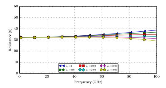
Figure 3.17: Resistance of a single helix in an ideal magnetic material.
