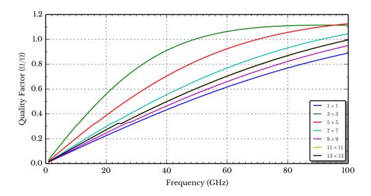
Figure 3.28: Simulated quality factor of nickel helix arrays.
