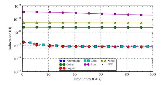
Figure 3.5: Inductance of the single wire shown in Figure 3.3 in free space.
