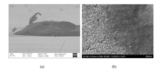
Figure 4.8: SEM micrographs of the silver conductive epoxy capping layer. (a) Epoxy shown deposited on top of the film. (b) Interface between the epoxy and the film.
