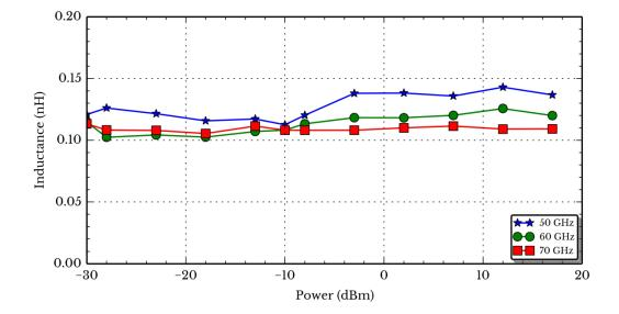
Figure 4.18: Measured inductance at 50, 60, and 70 GHz over a range of powers from -30 dBm to 17 dBm.
