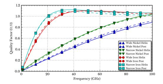
Figure 3.12: Comparison of the quality factor of wide and narrow helices made of iron and nickel. Also shown are the quality factors of the equivalent post inductors for both the narrow and wide helix.
