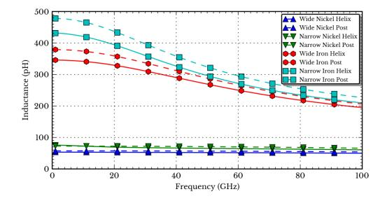
Figure 3.11: Comparison of the inductance of the wide and narrow helix made of iron and nickel. Also shown are the inductances of the equivalent post inductors for both the narrow and wide helix.
