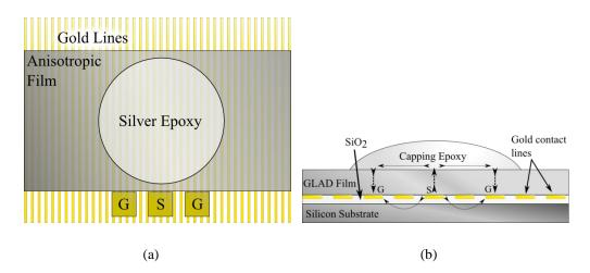
Figure 4.7: Capping technique measurement layout. (a) Top-down view of the conductive capping material (labeled silver epoxy). The material is placed directly on top of the film. (b) Cross-section view of the capping layer. The dashed lines show the direction of current through the device.
