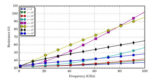
Figure 3.19: Resistance of a single helix embedded in a conducting magnetic material ( $\mu_r = 600$ )
