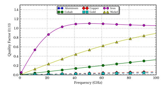
Figure 3.6: Quality factor of a single wire shown in Figure 3.3 in free space
