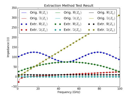
Figure D.1: Extracted impedance values for an arbitrary 2-port pi-model circuit plotted along the analytical values. The extraction process produced an exact match for the extracted devices.
