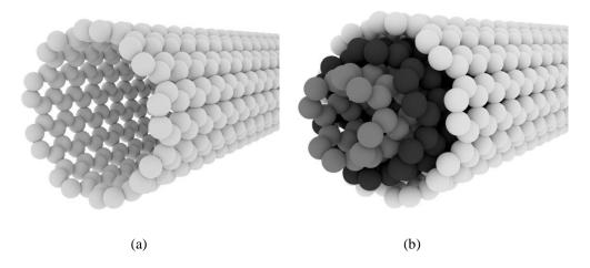
Figure 2.8: The structure of a carbon nanotube (ends not shown). On the left (a) is a single-wall carbon nanotube that consists of a single tube of carbon atoms. On the right (b) is a multi-wall carbon nanotube which consists of concentric rings of carbon atoms. The spheres in the multi-wall carbon nanotube are all carbon and are shaded to show how each tube is positioned in relation to the other tubes.
