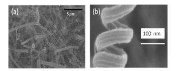
Figure 3.1: Image © IEEE 2010, reproduced from [70]. Original image caption: (a) SEM image for coiled CNWs [sic] with a (b) more detailed view. No preferred alignment was observed.
