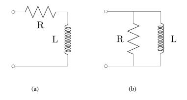
Figure 2.1: Inductor circuits. (a) Inductor model with a series resistance. Increasing the resistance in this model means that more power is lost in the resistor when compared to the inductor. (b) Inductor model with a parallel resistance. Increasing the resistance means that more power is stored in the inductor when compared to the resistor.
