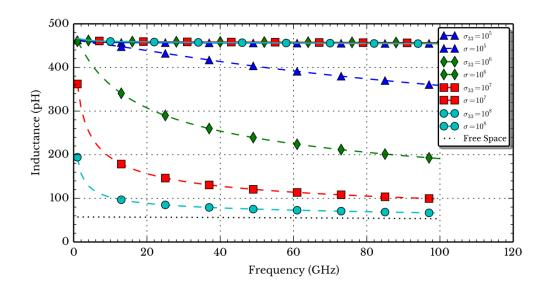
Figure 3.21: Inductance of an anisotropic conductive film compared to the isotropic film.
