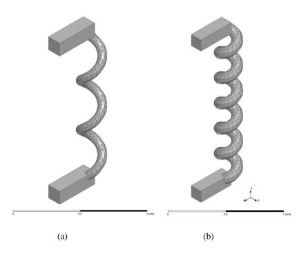
Figure 3.3: Models of single helices in free space. (a) Model of an individual element from the film shown in Figure 3.2a. (b) Model of an individual element from the film shown in Figure 3.2b
