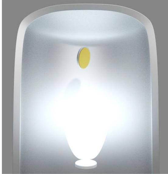
Figure 2.7: Set-up to perform glancing angle deposition with a sputtering system.
