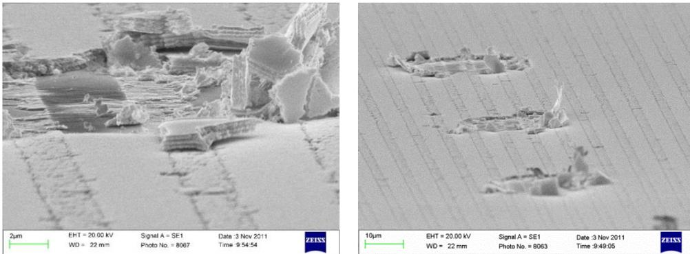
Figure 4.5: SEM image of damage to the GLAD film due to direct contact with the RF probe.
