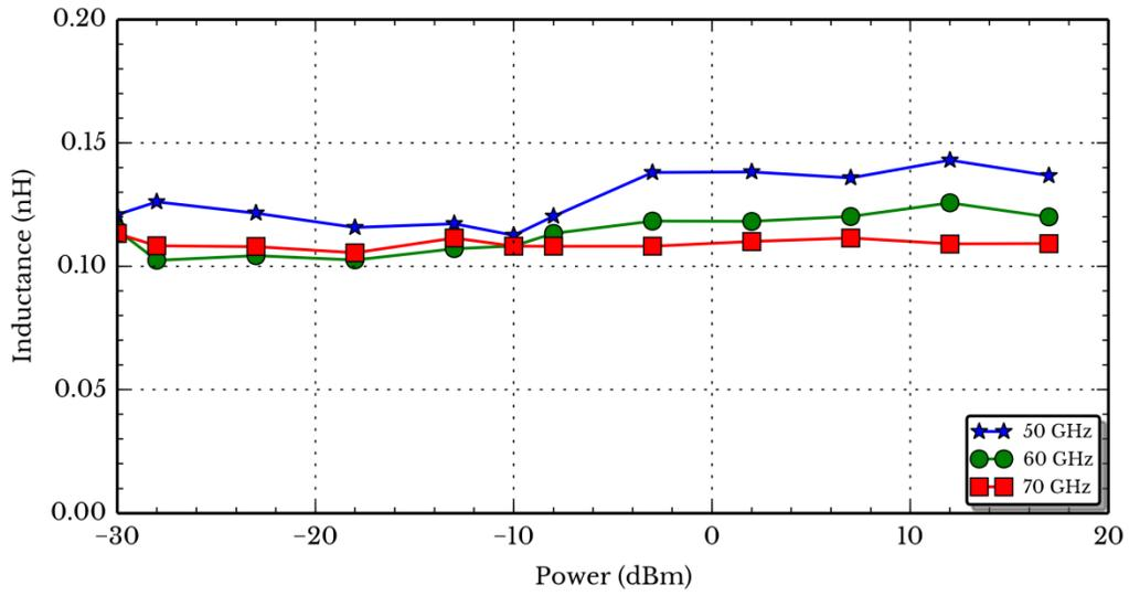
Figure 4.18: Measured inductance at 50, 60, and 70 GHz over a range of powers from -30 dBm to 17 dBm.
