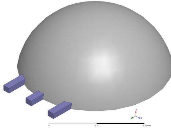
Figure 4.13: Simulation model of the silver epoxy. The blue lines on the left are the GSG probe lines which end on the surface of the silver (grey).
