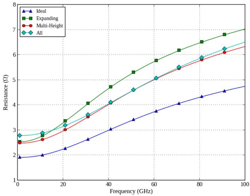
Figure 3.35: Resistance of a  $7 \times 7$  helix array with defects added.
