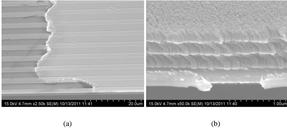
Figure 4.3: Fabricated nickel film. (a) A portion of the GLAD film with good uniformity. (b) A close-up view of the nano-structure of the film featuring the closely-packed helices.
