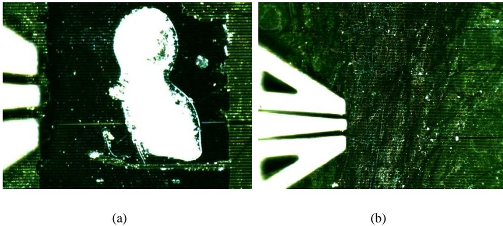
Figure 4.10: Measurement setup with: (a) silver epoxy capping layer (white), gold (green) and anisotropic film (black) and (b) with the film removed.
