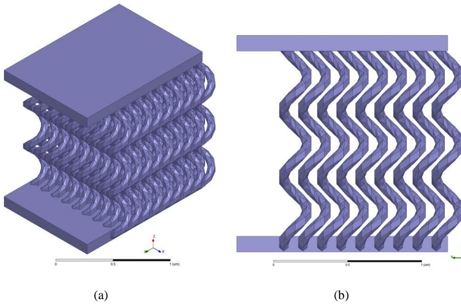
Figure 3.26: Detailed view of the  $9 \times 9$  helix array. (a) isometric view of the helix array showing the 2-dimensional square array. (b) side view of the helix array showing the top and bottom lines that connect to the port as well as the completely separated nature of the helices.
