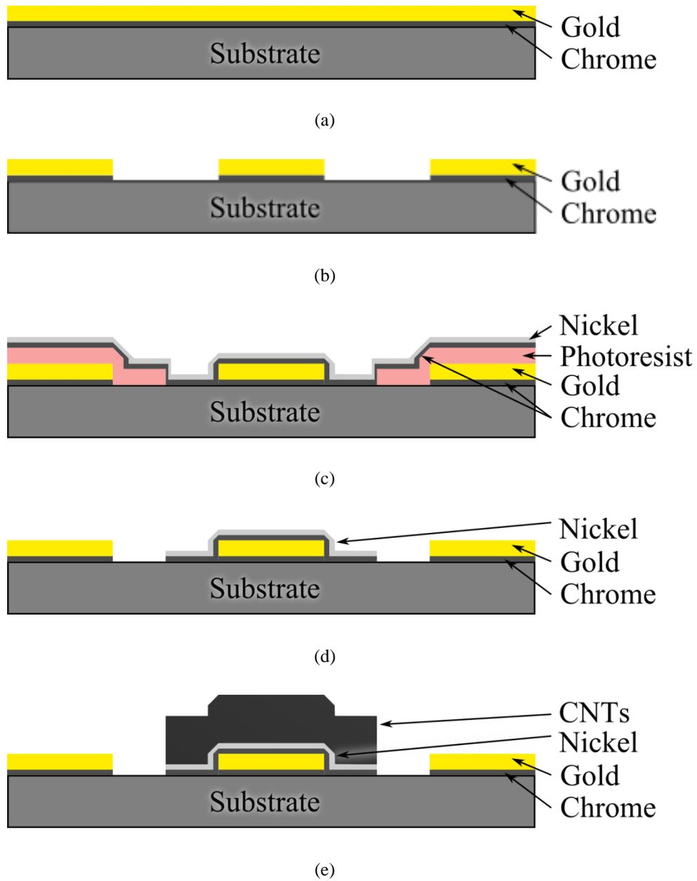
Figure A.1: Process flow for the carbon nanotube test substrate showing cross-sections at key process steps.
