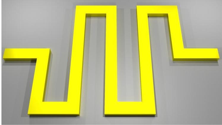
Figure 2.4: Two-turn meander inductor
