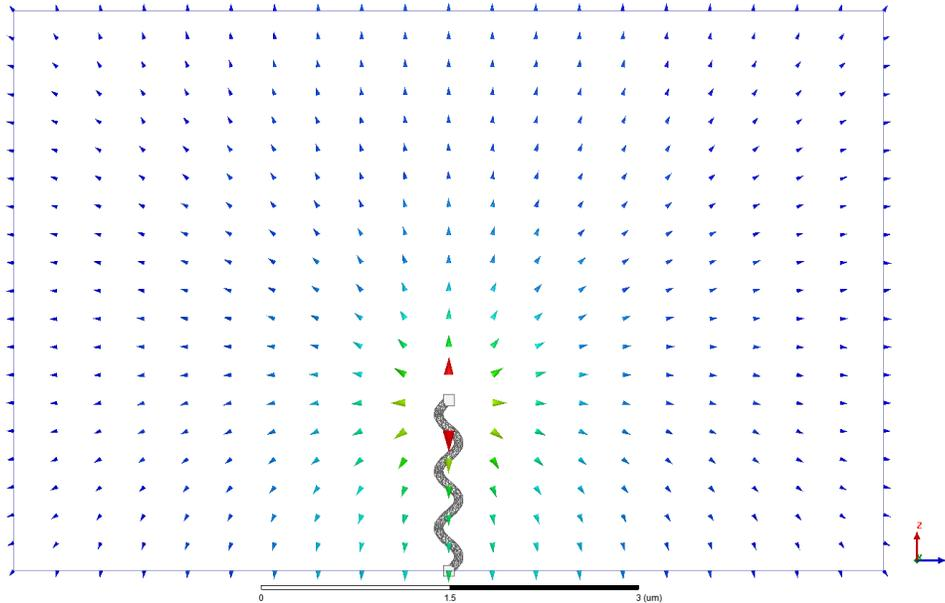
Figure 3.4: Wave port excitation in relation to the inductor model. The colored arrows show the electric field solution in the wave port plane.
