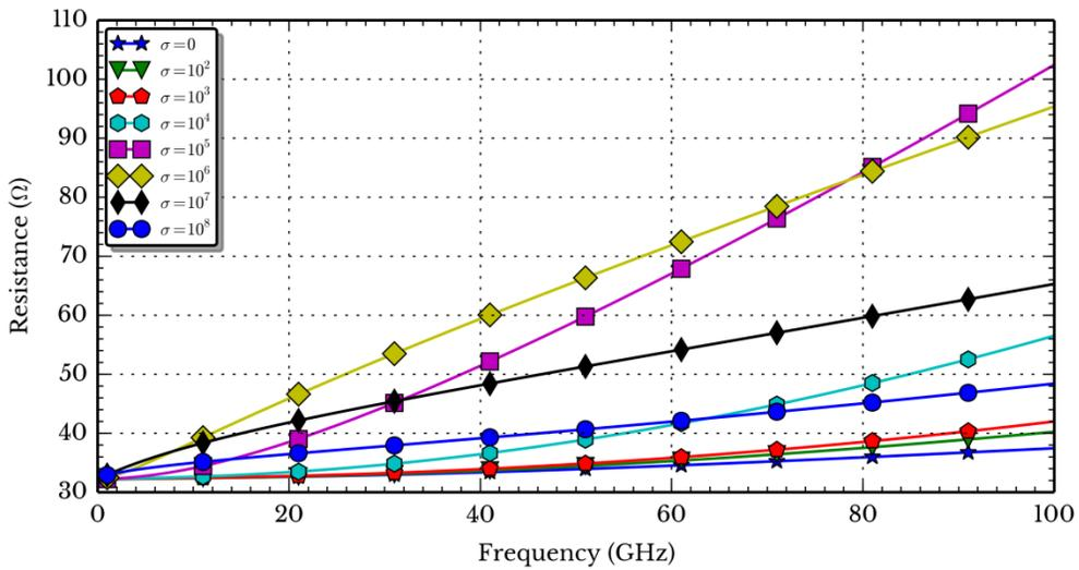
Figure 3.19: Resistance of a single helix embedded in a conducting magnetic material ( $\mu_r = 600$ )
