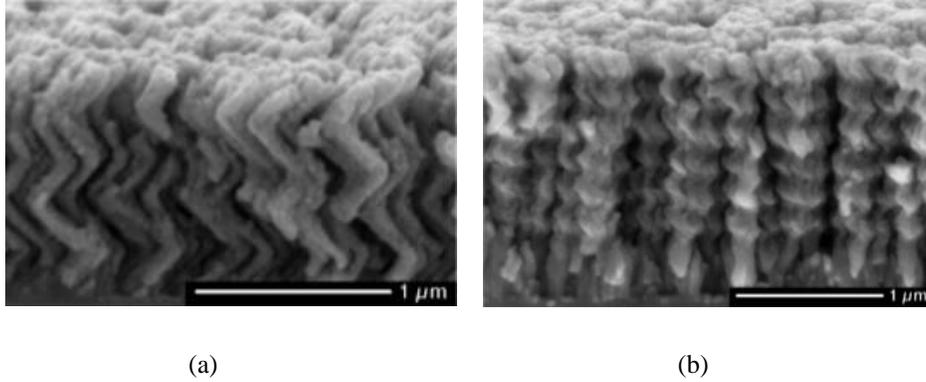
Figure 3.2: Nano-scale helix structures fabricated using physical vapour deposition from [69]. Both (a) and (b) were modeled as part of this work. In this work, (a) is called a wide helix and (b) is called a narrow helix.
