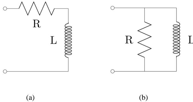
Figure 2.1: Inductor circuits. (a) Inductor model with a series resistance. Increasing the resistance in this model means that more power is lost in the resistor when compared to the inductor. (b) Inductor model with a parallel resistance. Increasing the resistance means that more power is stored in the inductor when compared to the resistor.
