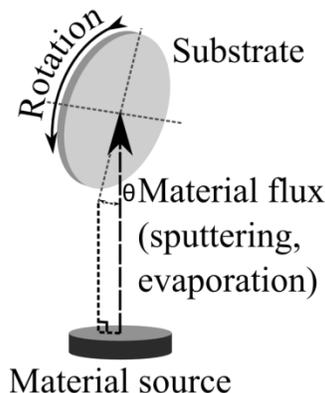
Figure 4.1: Glancing angle deposition setup.
