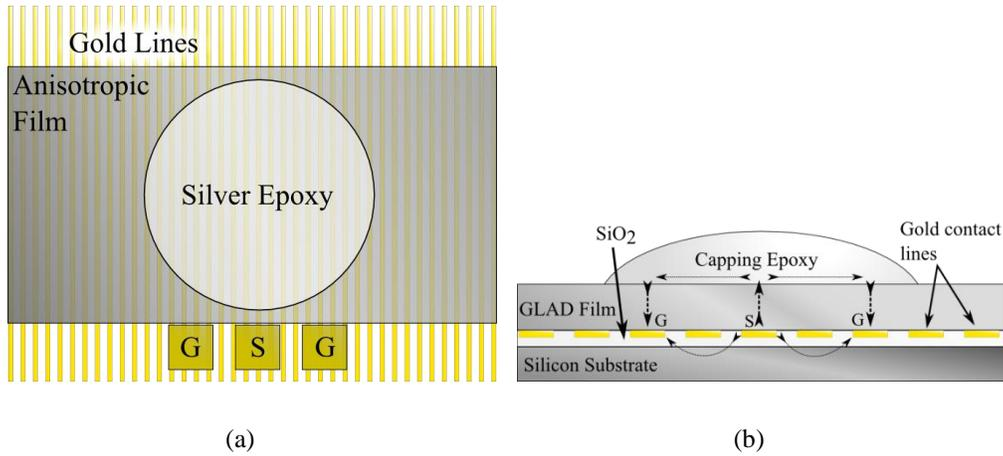
Figure 4.7: Capping technique measurement layout. (a) Top-down view of the conductive capping material (labeled silver epoxy). The material is placed directly on top of the film. (b) Cross-section view of the capping layer. The dashed lines show the direction of current through the device.
