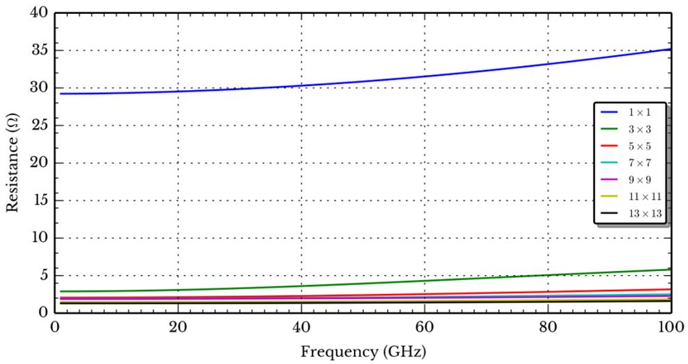
Figure 3.29: Simulated resistance of nickel helix arrays.
