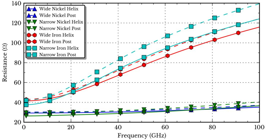
Figure 3.13: Comparison of the resistance of wide and narrow helices and the equivalent length of a straight wire.
