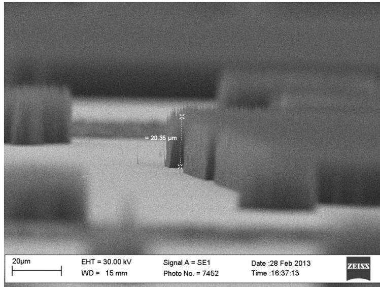
Figure 5.5: Carbon nanotube growth on substrate.
