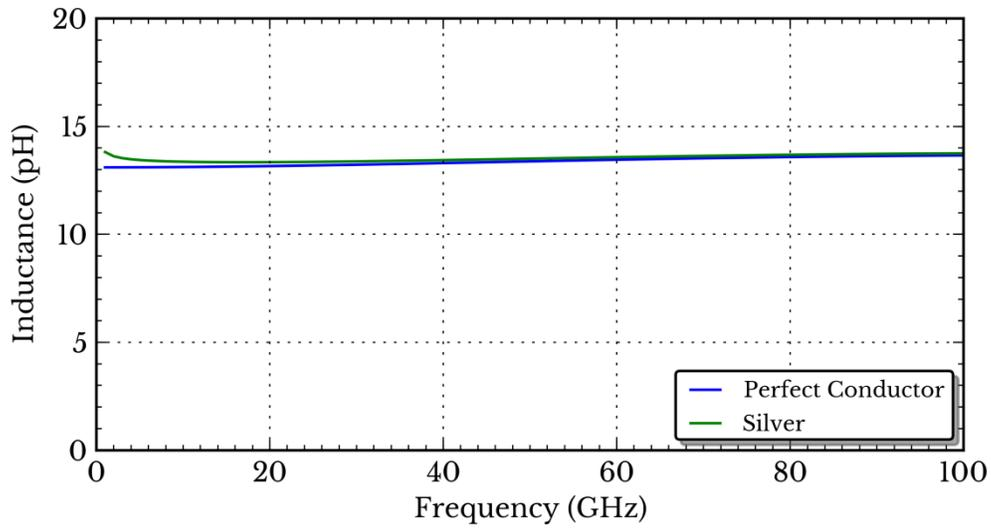
Figure 4.14: Simulated inductance of the silver epoxy.
