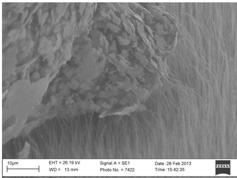
Figure 5.7: CNT adhesion to silver epoxy.
