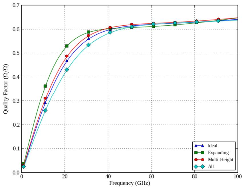
Figure 3.36: Quality factor of a  $7 \times 7$  helix array with defects added.
