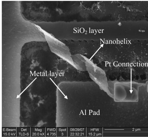
Figure 2.5: Stressed thin-film inductor © 2008 IEEE, reproduced from [38]. The original figure text: SEM image of a suspended two-turn nanohelix aluminum inductor fabricated using FIB-SIT. The inductor with an air-core is 2  $\mu\text{m}$  higher [sic] above [the] silicon substrate and is isolated from the substrate through a silicon dioxide layer between the metal layer and the substrate.
