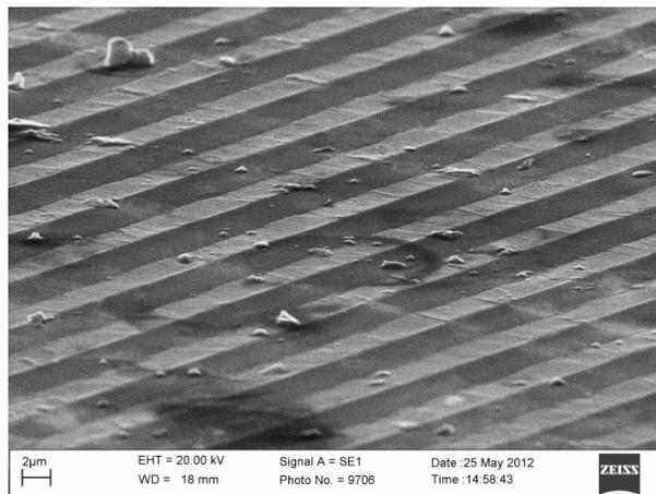
Figure 4.11: SEM image of gold lines after the GLAD film was manually removed.
