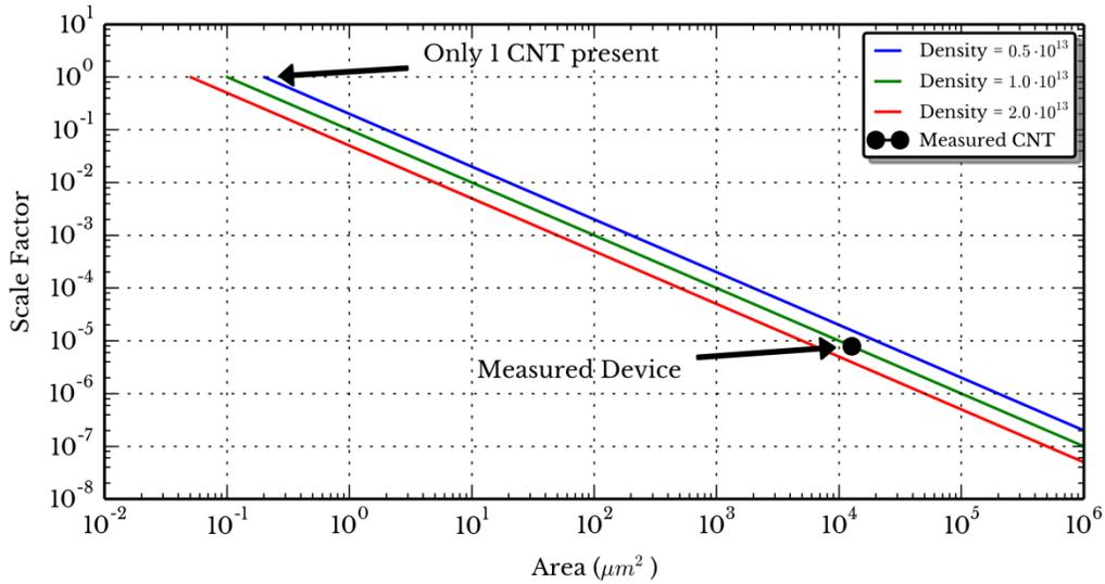
Figure 5.3: Scaling behaviour of CNT bundles by area.
