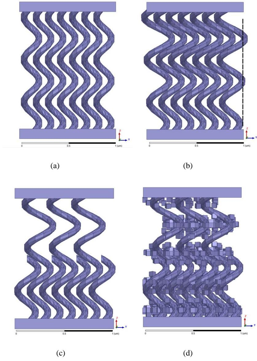
Figure 3.33: Helix width comparison. (a) An idealized helical film. (b) The same film but with a radius change of 50% between bottom and top. The radius change is emphasized by the vertical, dashed line. (c) Addition of helix termination defects to the model in (b). (d) Addition to random growth defects to the model in (c). The defects are modeled as arrays of cubes of material that are placed pseudo-randomly. This model includes all observed defects.
