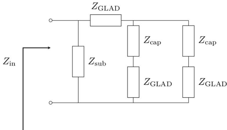
Figure 4.12: Circuit model for extraction of the GLAD film.
