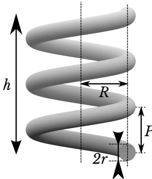
Figure B.1: Parameters of a helix;  $h$  is the helix height,  $R$  is the helix radius,  $r$  is the radius of the wire, and  $P$  is the helix pitch.
