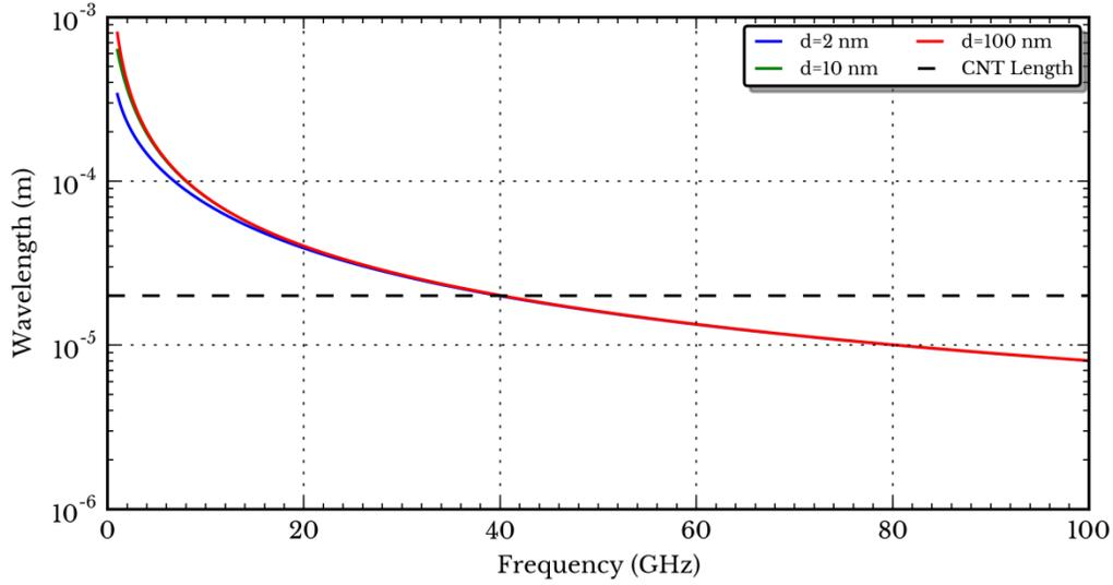
Figure 5.1: Wavelength of a SWCNT of varying diameters and 20  $\mu\text{m}$  in length. As the frequency increases, the CNT length becomes close to the wavelength and the CNT length is equal to the wavelength around 40 GHz. This ultra-short wavelength for a CNT transmission line causes even short CNT devices to act as distributed elements.
