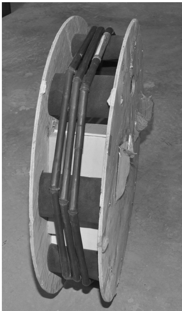
FIG. 2—SAA on spool (7.2 m (24 ft) array shown).
