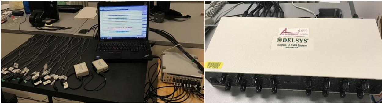
Figure 11. The utilized EMG setup. Left: Powerlab 16/35 data acquisition system, the LabChart data acquisition software, and the EMG electrodes; right: the Bagnoli-16 EMG system amplifier.
