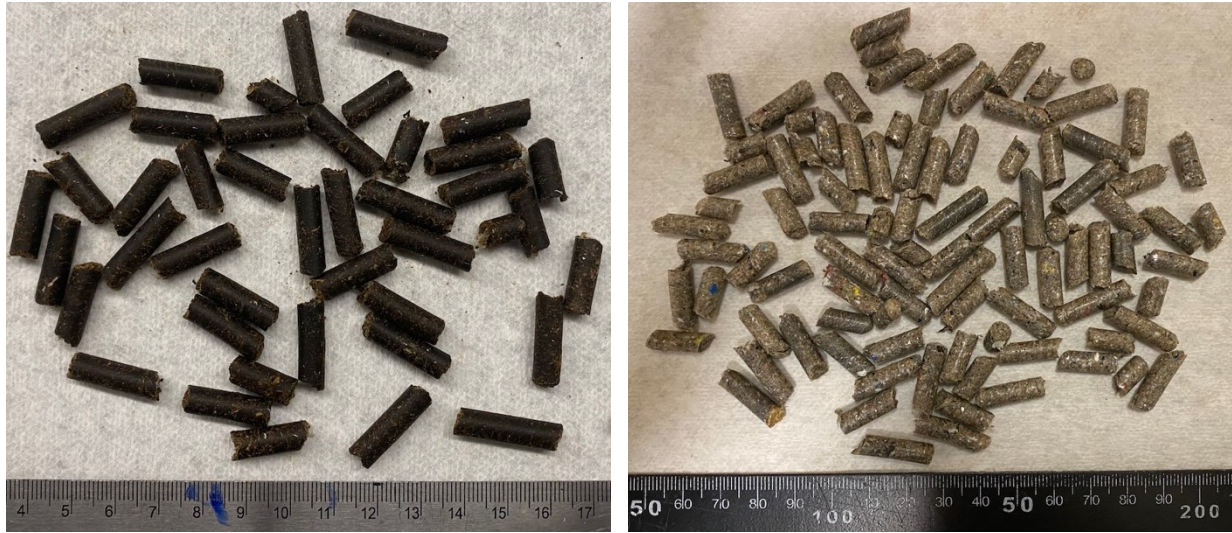
Figure 6: Produced pellets. Left: SSO pellets; Right: RDF pellets. Both at 4 mm and 10 %.
