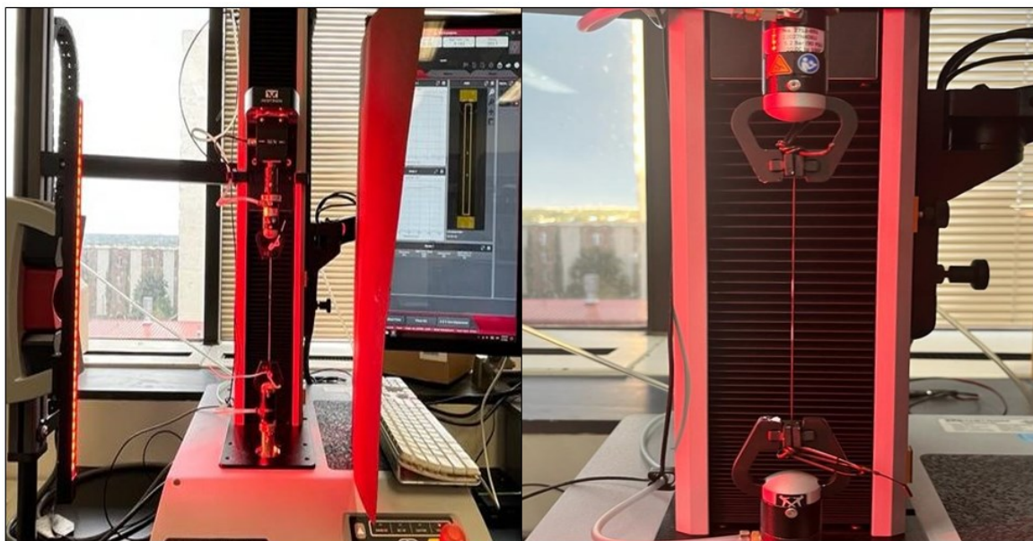
Figure 5: Intron tensile machine testing of pigmented LLDPE filaments
