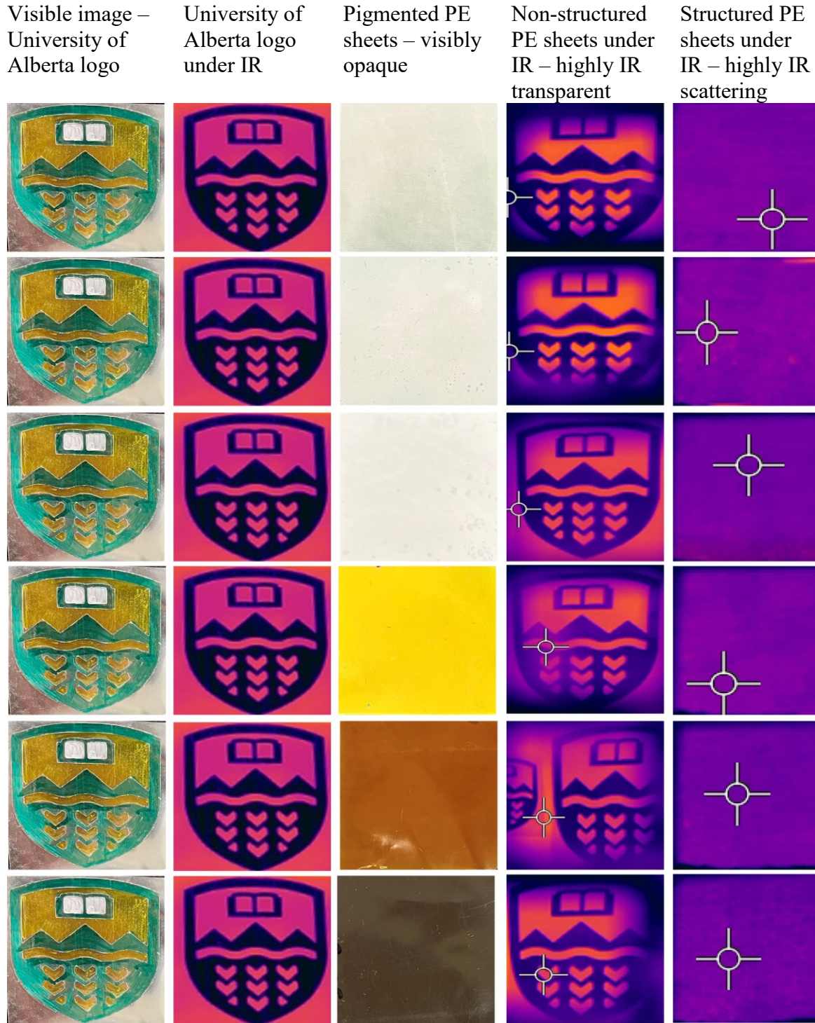
Figure 30: Results of micro-structuring of pigmented PE sheets- conversion of PE from highly IR transparent to highly IR scattering
