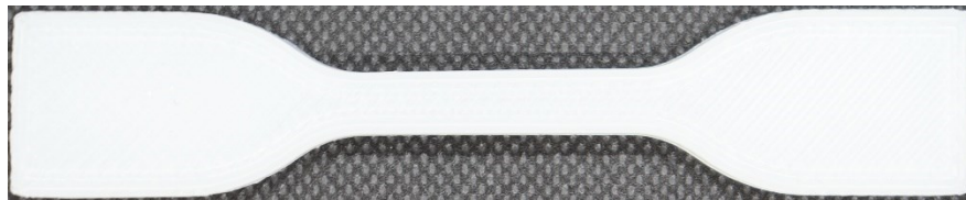
Figure 33:ASTM D638-IV - 3D printed Tensile test specimen: 100% infill density
