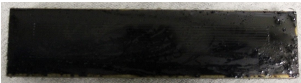
Figure A3.1. Photograph of a coated plate with frozen wall-coating prior to the flow tests.
