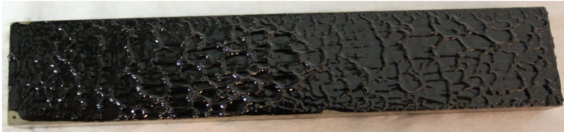
Figure A3.2. Photograph of a frozen wall-coating layer after the flow tests.
