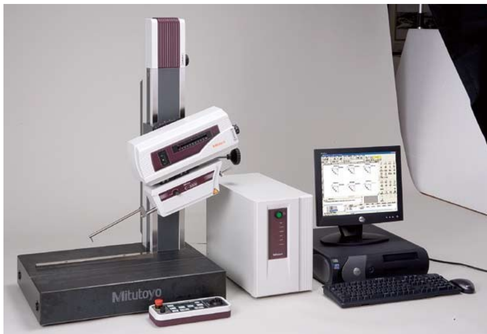
Figure A4.1. Photograph showing basic parts of the MITUTOYO Contracer.
