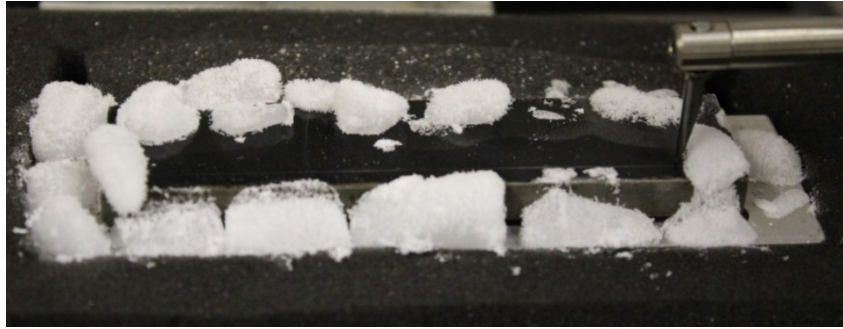
Figure A4.2. Photographs showing the roughness measurement with MITUTOYO Contracer: (a) Complete setup of Contracer in operation; (b) The stylus moving over the oil surface frozen with dry ice.
