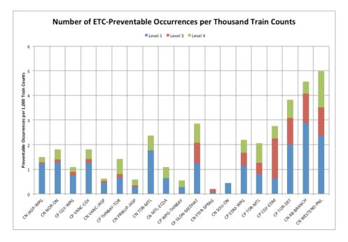
**Figure 2-8.** Normalized ETC preventable occurrences within each corridor at each ETC Level per thousand train counts.
