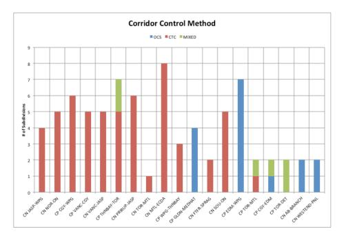
Figure 2-5. Breakdown in control method by number of subdivisions within each corridor.
