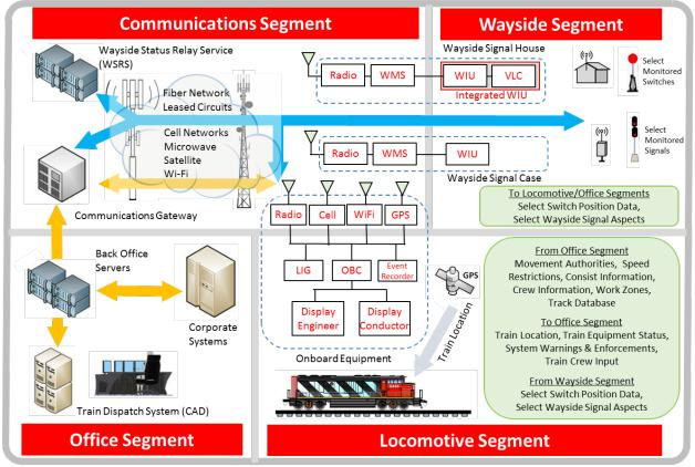
Figure 1-3. Level 2 ETC system.
