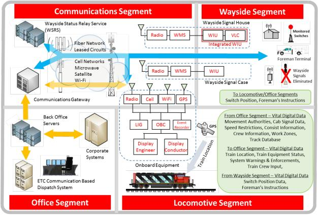
Figure 1-5. Level 4 ETC system.
