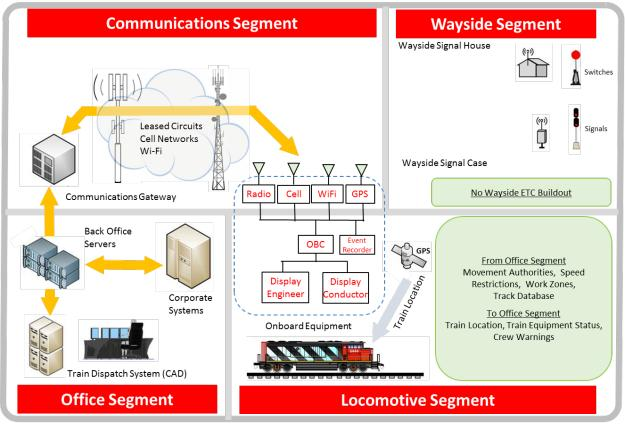
Figure 1-2. Level 1 ETC system.
