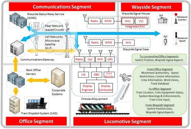
Figure 1-4. Level 3 ETC System.
