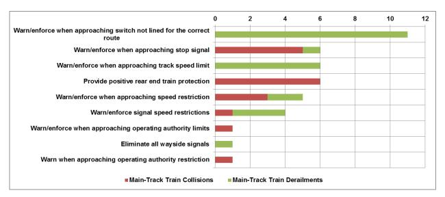
**Figure 1-16.** Breakdown in the key functionality of a Level 4 ETC system in terms of the number main-track train accidents it would prevent (40 in total). Red and green bars represent the main-track train collision and derailment contributions, respectively.
