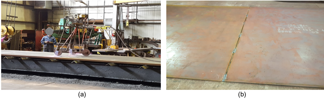
Figure 2.12. (a) Journeyman operating at web cutting workstation; (b) two web plates tacked together ready for shop splicing.
