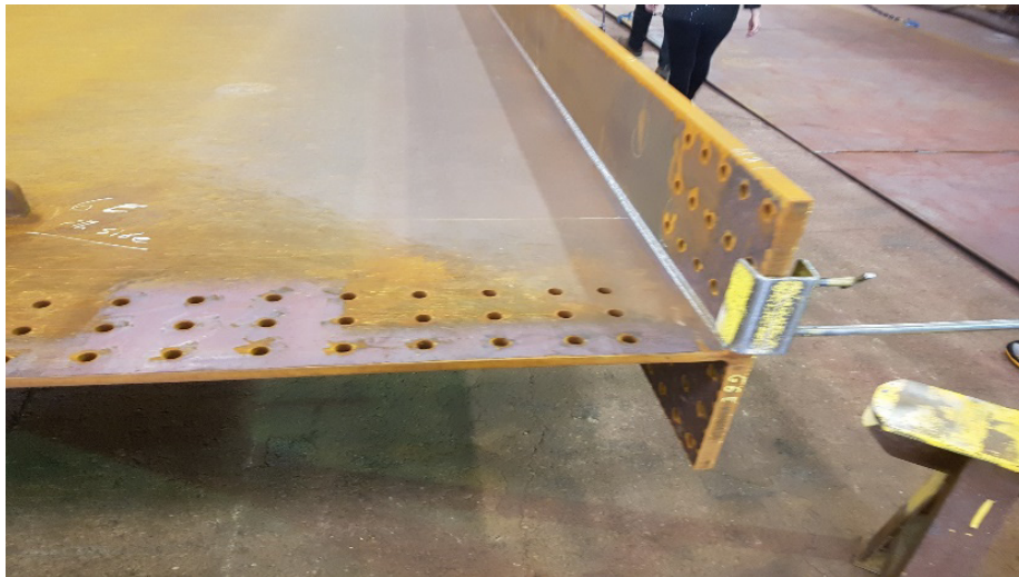
Figure 2.14. A girder with finished field splice drilling.
