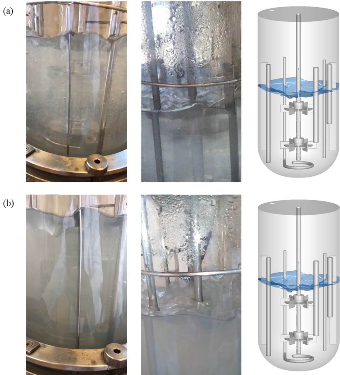
Figure 7.2. Interface surface prediction for the batch abiotic systems with non-Newtonian fluids, using the domain GeomC. Comparison between the experimental and simulated surface, for (a) Xanthan Sol B and (b) Xanthan Sol A. For the computed results, the water-air interface was plotted as an instantaneous iso-surface of volume fraction of air equal to 0.1.
