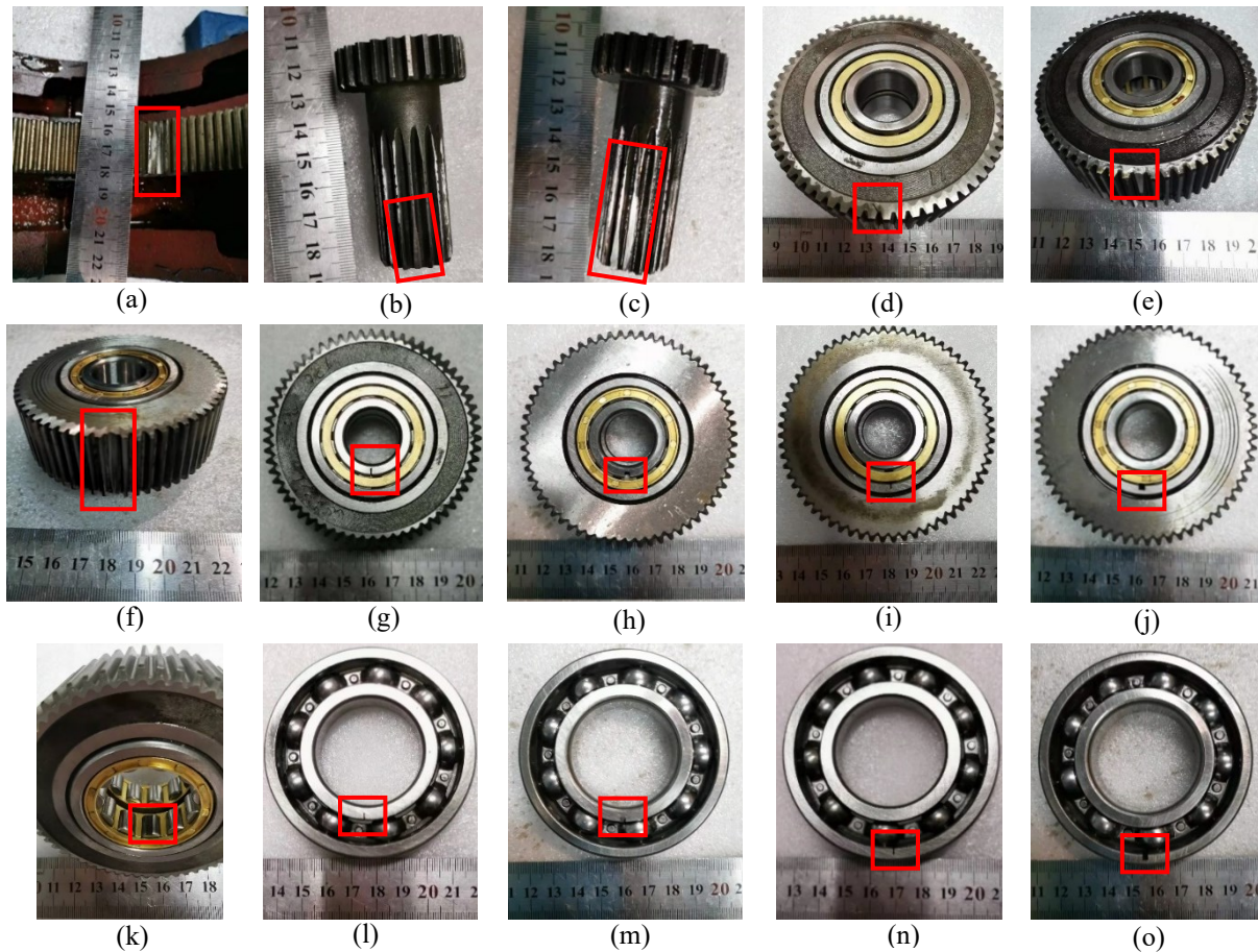
Fig. 4.7: Seeded faults of planetary gearbox: (a) Ring gear tooth missing, (b) Sun gear chipped tooth, (c) Sun gear tooth missing, (d) Planetary gear tooth root crack, (e) Planetary gear chipped tooth, (f) Planetary gear tooth missing, (g) Planetary bearing inner race crack (hereinafter, bearing race crack means the crack width = 0.4 mm), (h) Planetary bearing inner race fault (hereinafter, bearing race fault means induced crack width = 2 mm), (i) Planetary bearing outer race crack, (j) Planetary bearing outer race fault, (k) Planetary bearing rolling element fault, (l) Input shaft bearing inner race crack, (m) Input shaft bearing inner race fault, (n) Input shaft bearing outer race crack and (o) Input shaft bearing outer race fault. Seeded faults are marked in red rectangles.
