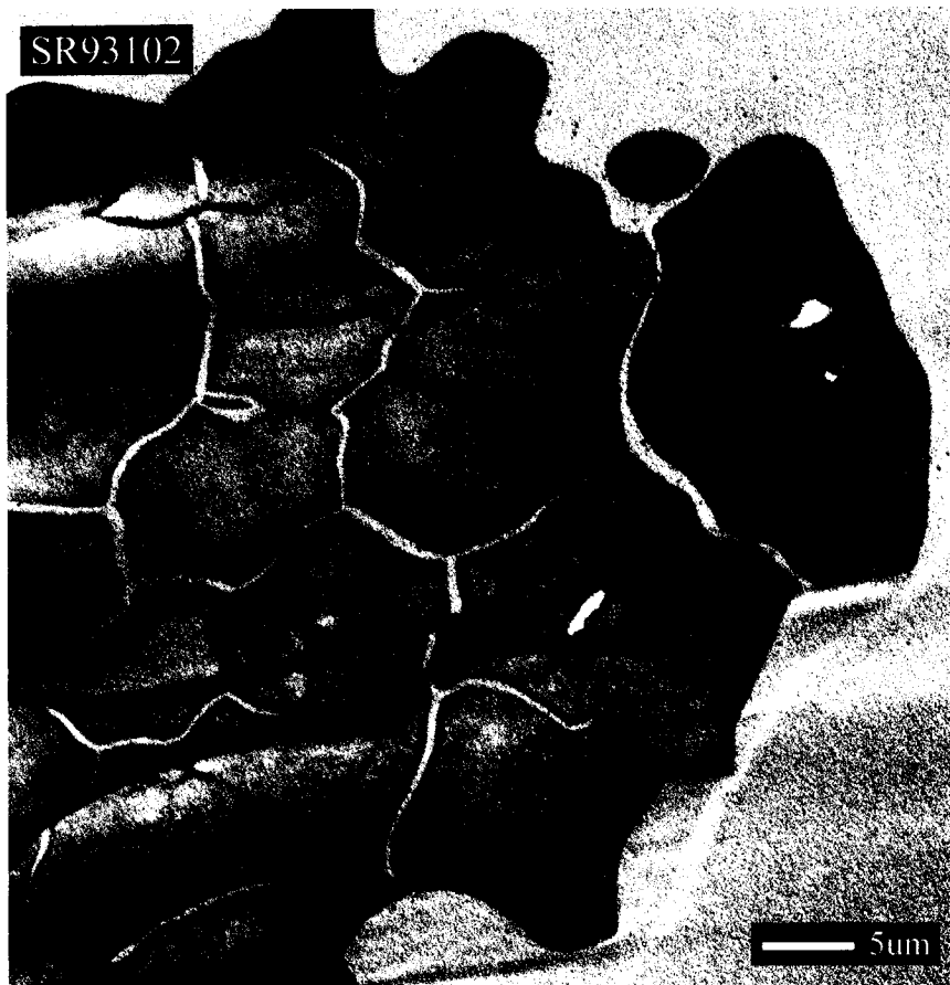
Figure 2-4 Transmission electron micrograph of compound hull-less barley starch granules from SR 93102 (Magnification X7200).
