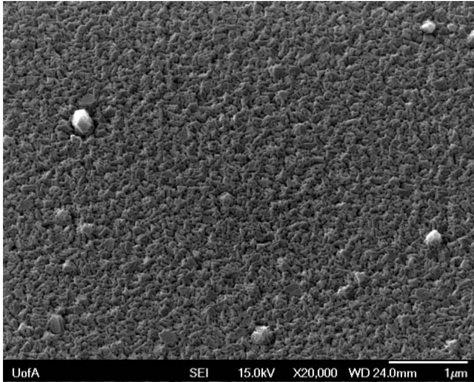
Figure 5.44 Anodized Sputtered Aluminum/Tantalum film 16 V, 10 min, 20KX
