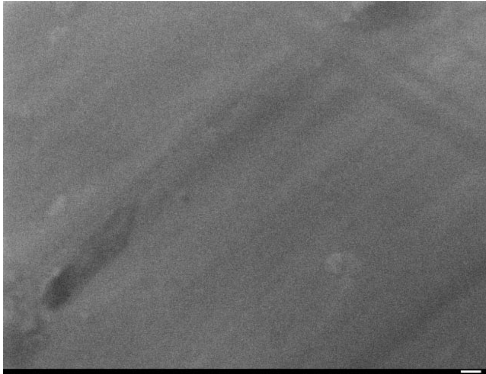
Figure 5.5: 10 min Anodized Aluminum Foil at 20 V, 50KX Magnification
