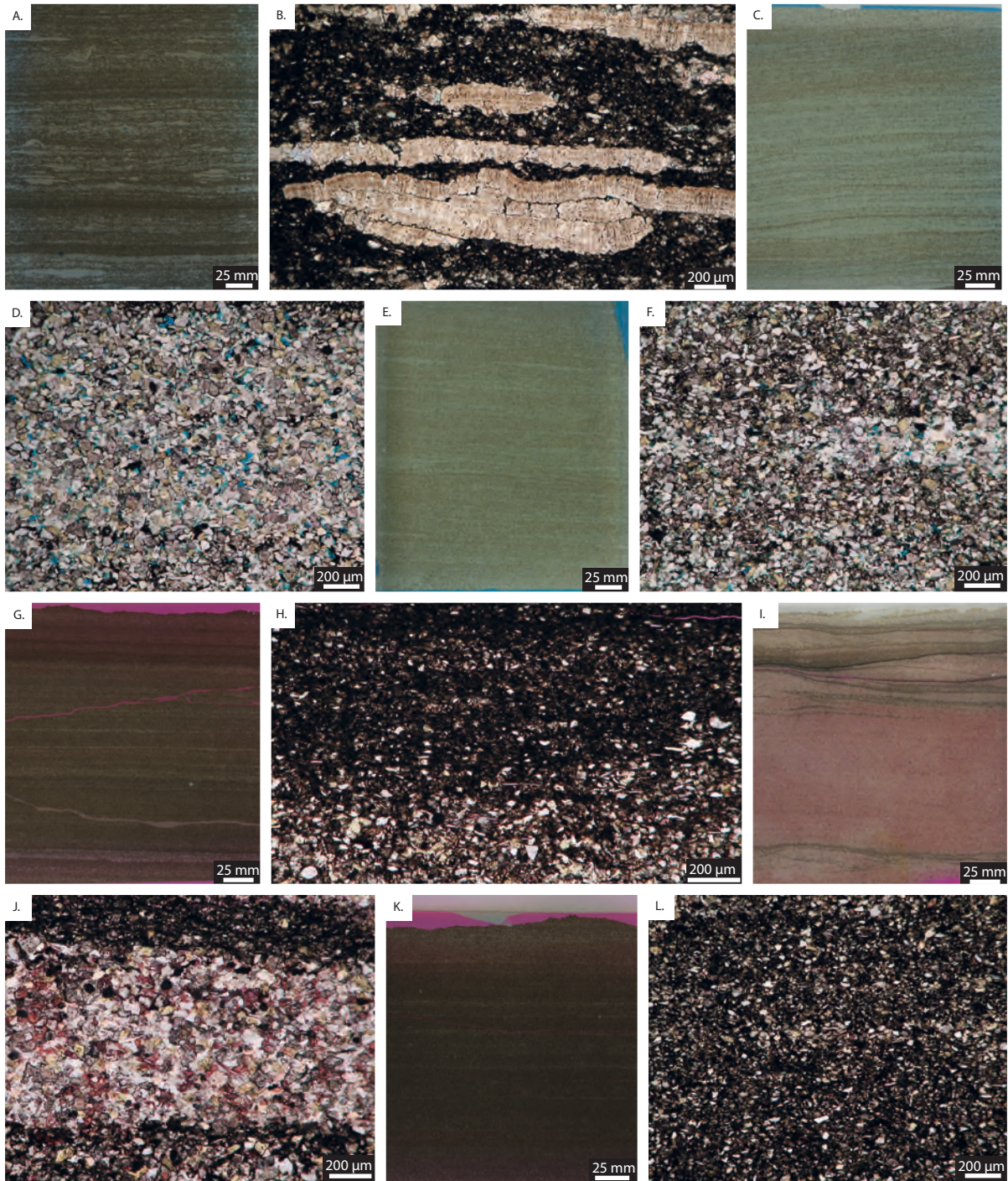
Fig 2.6- Scanned images of thin sections and thin section photomicrographs of each facies. All think section photomicrograph photos are in PPL and 20X magnification, thin sections have been double carbonate stained and feldspar stained. A-B. Fragmented Claraia shells in Lithofacies 3; 15-31-77-10; 2224.65m. C-D. Coarser bed in Lithofacies 5, note lack of calcite cement; 14-33-78-11w6; 2106.25m. E-F. Lithofacies 5; 14-33-78-11w6; 2109.75m. G-H. Lithofacies 6; interbedded silty shale and siltstone beds; 4-16-78-12w6; 2262.06m. I-J. Lithofacies 7; lenticular bedded siltstone, note intensive calcite cementation throughout coarse lense; 2-5-79-11w6; 2045.82m. K-L. Lithofacies 8; fine bituminous siltstone; 4-16-78-12w6; 2264.31m.
