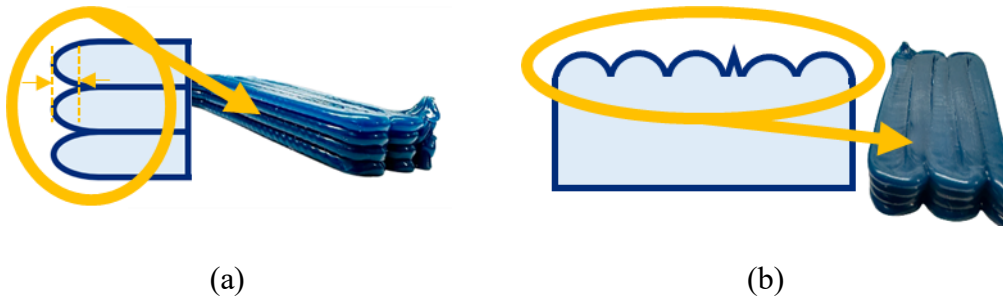
Figure 4-5. Response variables selected for the DoE (a) Stair-Stepping depth and (b) Valleys & Ridges
