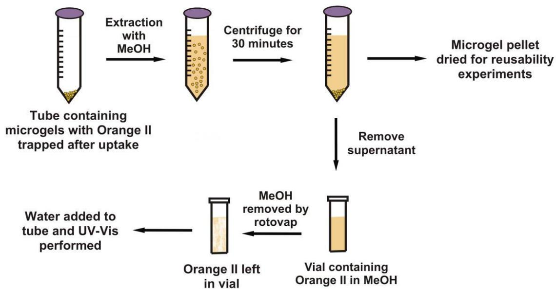
**Scheme 1.** Schematic depicting the extraction process used in this study.
