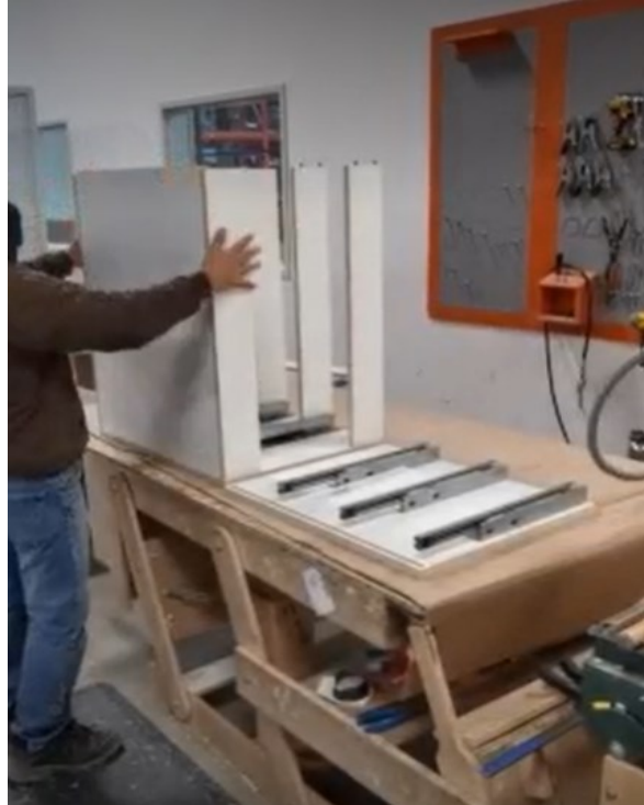
Figure 12: Cabinet building in the pre-assembly stage after hardware installation
