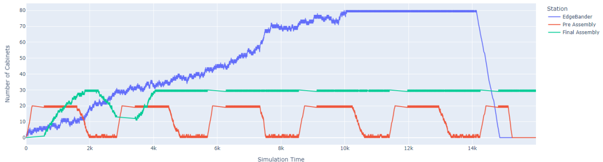
Figure 33: WIP levels of EB, pre-assembly, and final assembly stations over simulation time
