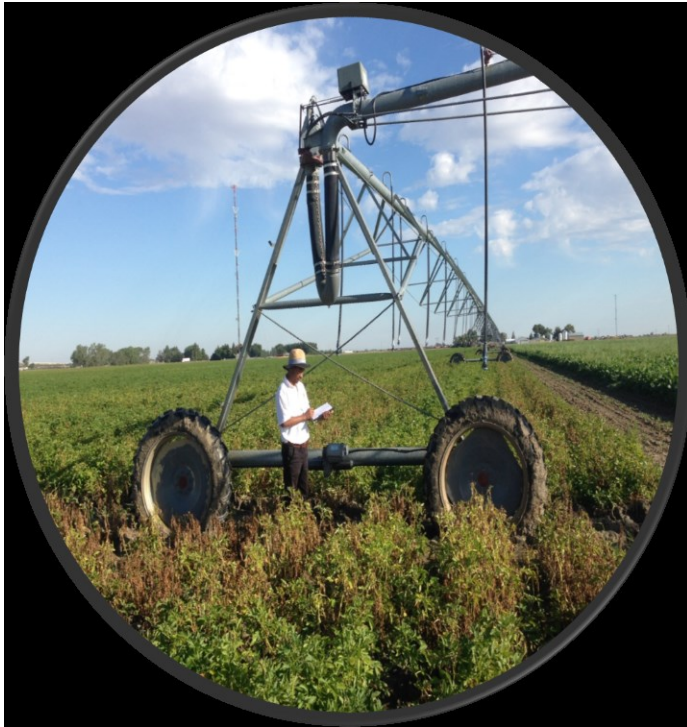
Figure 3-5: A typical low pressure pivot system in southern Alberta Source: Author (August 2015)
