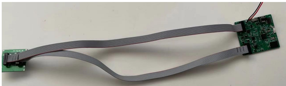
Figure 5-4 The connection between the data acquisition board and the sensing board
