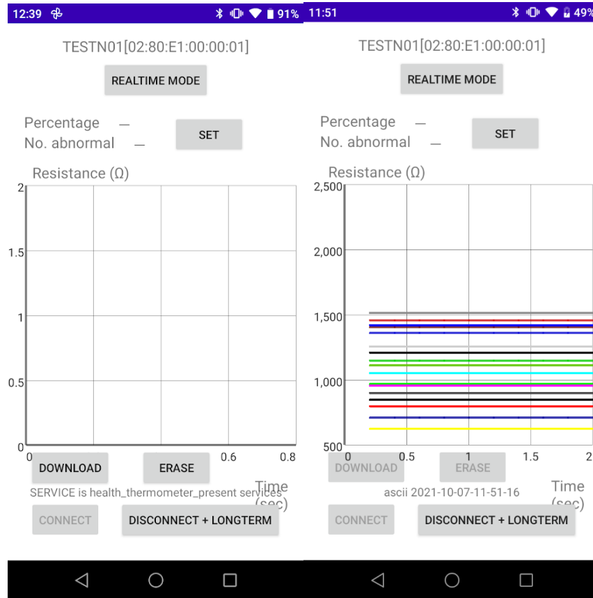
Figure 4-5 Communication page of the graphical user interface when just connected (Left) and in real-time mode (Right)
