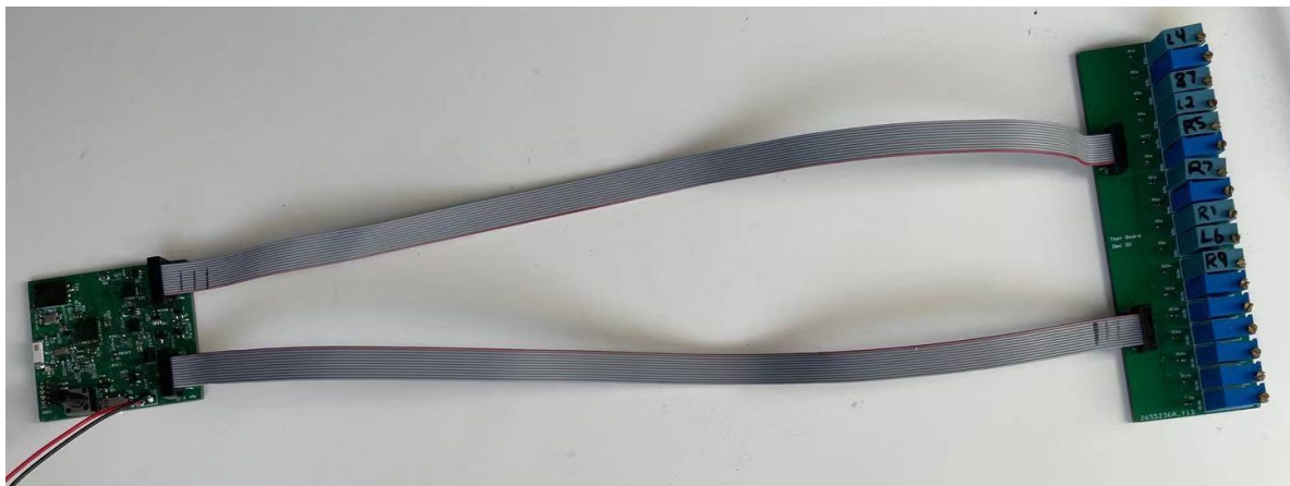
Figure 5-8 The connection between the simulated sensor board and node data acquisition board
