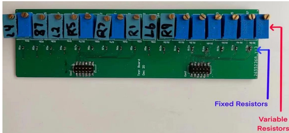
Figure 5-7 The simulated sensor board
