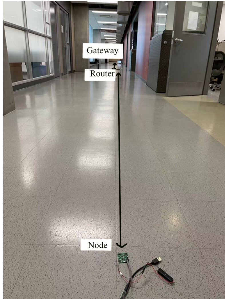
Figure 5-16 Experimental setups for communication range test between node and gateway
