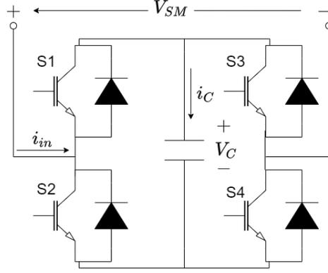
Figure 2.6: Full Bridge Submodule [34]
