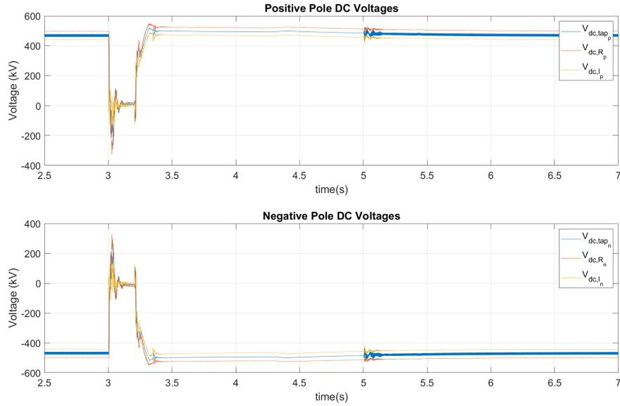
Figure 4.31: Pole DC Voltages of LCC-HVDC System during a Three phase AC Fault at the Inverter Station with pre-fault loading scenario  $P_{dc,p} = P_{dc,n} = 0 \text{ MW}$
