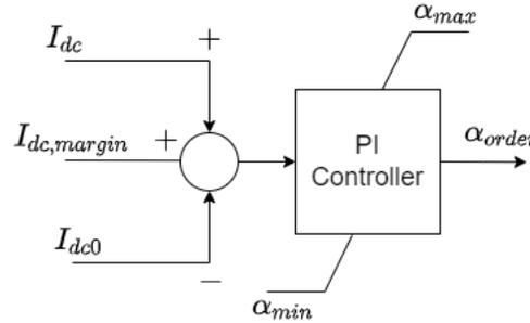
Figure 2.13: Current Control Amplifier [35]
