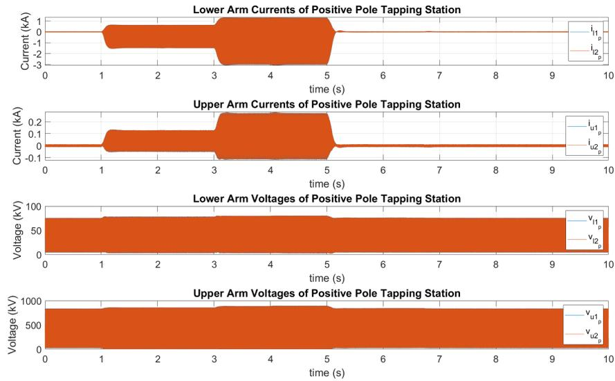
Figure 3.7: Arm Currents and Voltages of Positive Pole Tapping Station M2DC-CT,  $P_{dc,p} = P_{dc,n}$
