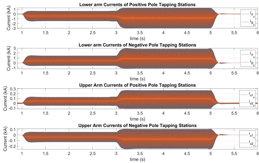
Figure 3.17: Arm Currents of Tapping Stations M2DC-CTs when  $P_{dc,p} = -P_{dc,n}$
