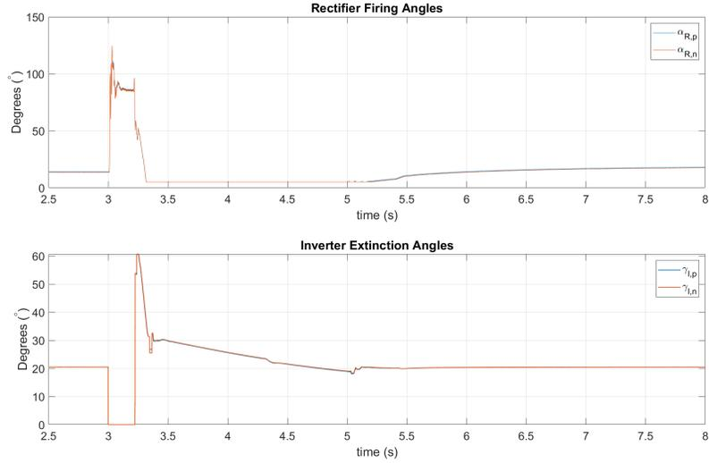
Figure 4.33: Firing Angles and Extinction Angles Variations during a Three phase AC Fault at the Inverter Station with pre-fault loading scenario  $P_{dc,p} = P_{dc,n} = 0$  MW
