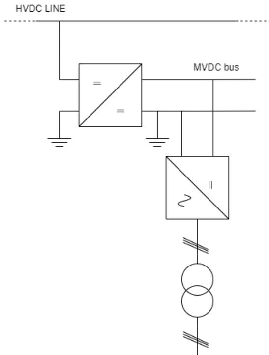
Figure 1.5: DC Tapping using parallel connection [24]
