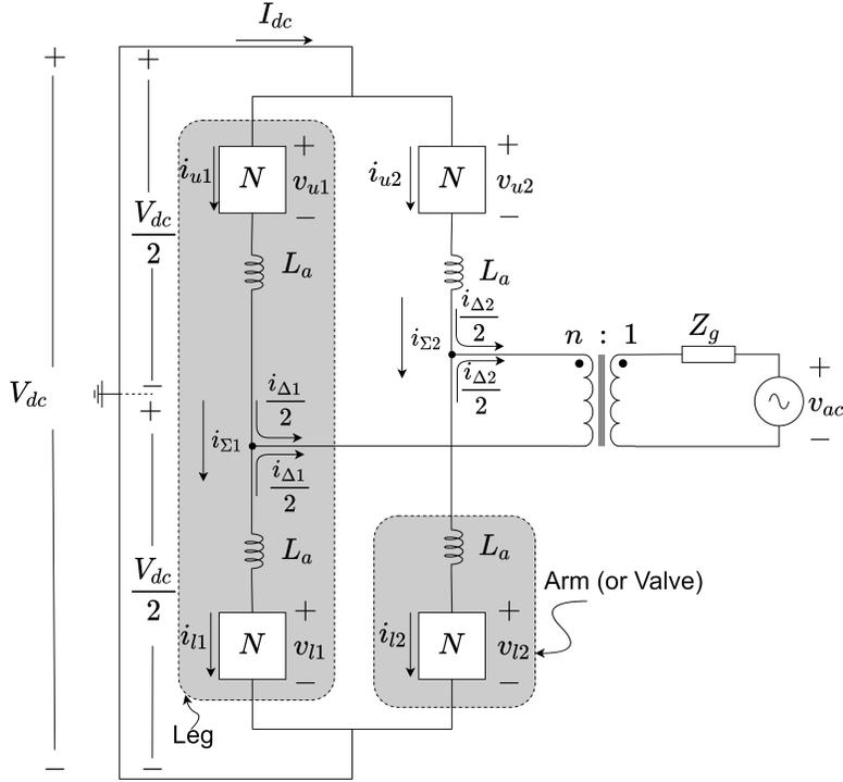
Figure 2.4: Single Phase MMC using Two Phase Legs
