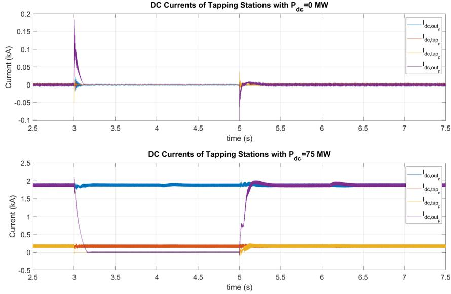
Figure 4.13: Tapping Stations DC Input and Output Currents during an MVDC bus DC Fault at positive pole tapping station
