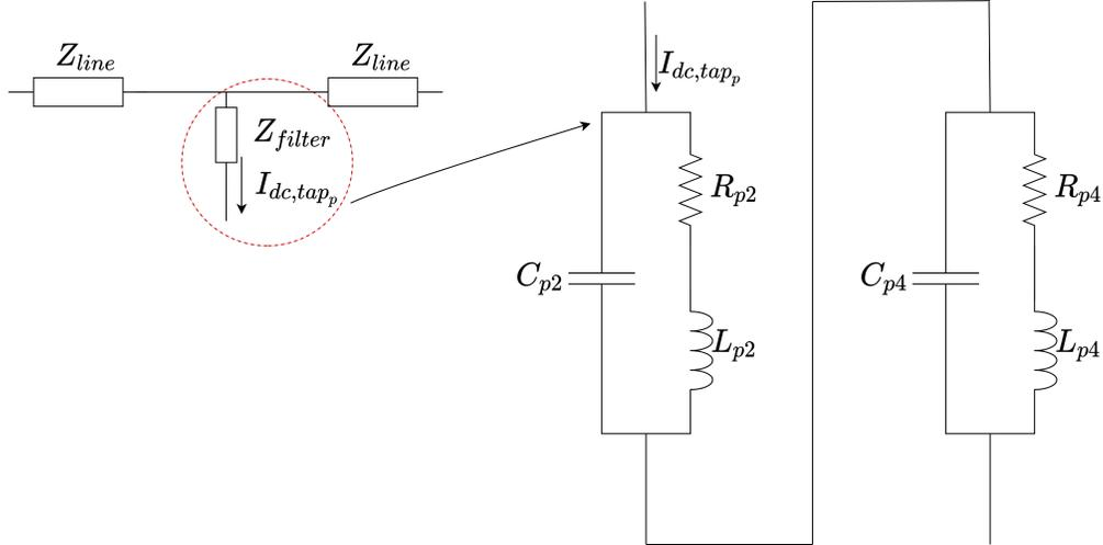
Figure 2.16: Parallel LC Filters ( $Z_{filter}$ ) used at M2DC-CT inputs in Figure 2.9 [17]
