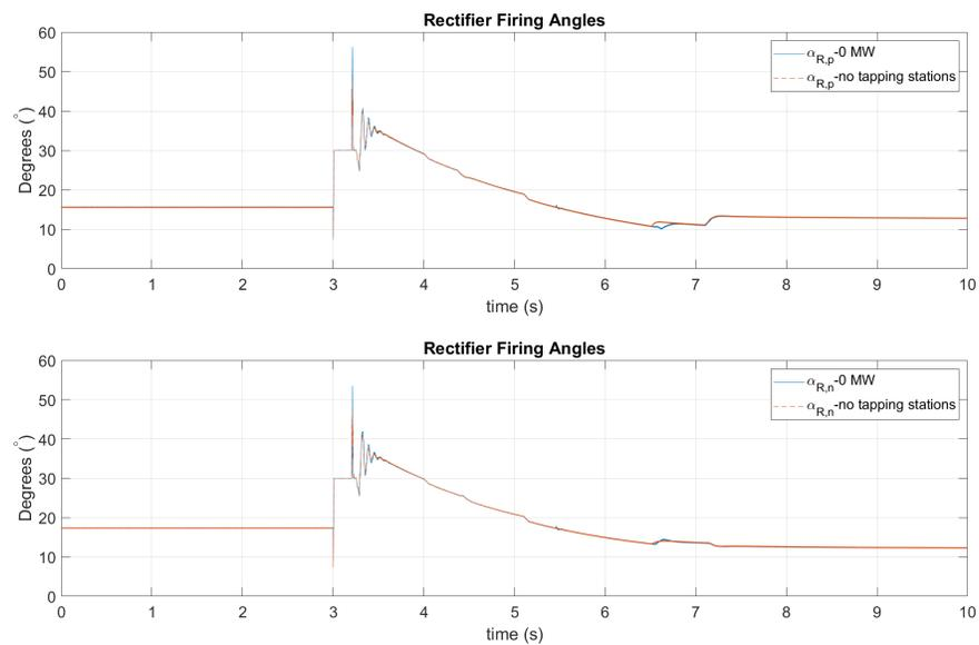
Figure A.1: Comparison of Rectifier Firing Angles with and without the presence of tapping stations
