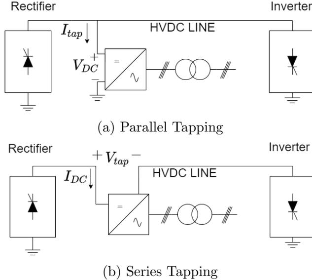
Figure 1.3: Concept of Series and Parallel Tapping [21]
