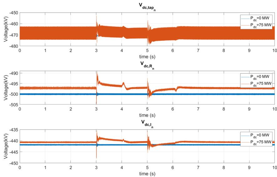
Figure 4.10: LCC-HVDC Negative Pole DC Voltages variations during an MVDC bus DC Fault
