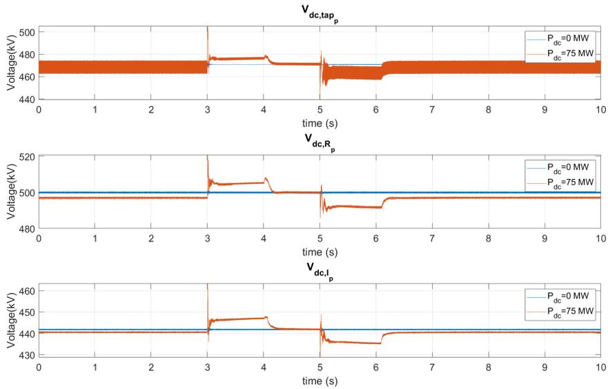
Figure 4.9: LCC-HVDC Positive Pole DC Voltages variations during an MVDC bus DC Fault at positive pole tapping station
