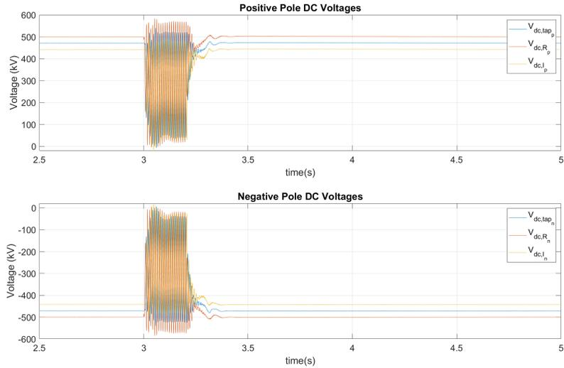
Figure 4.22: Pole DC Voltage Variations during a single line-to-ground AC Fault
