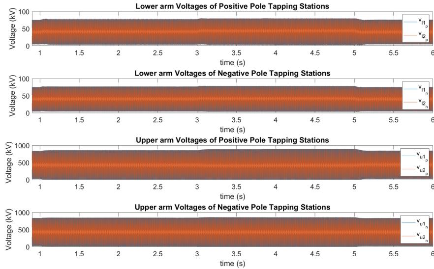
Figure 3.13: Arm Voltages of Tapping Stations M2DC-CTs,  $P_{dc,p} = 2P_{dc,n}$
