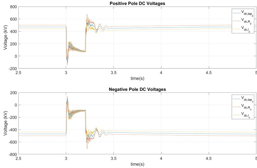
Figure 4.16: HVDC DC Link Pole Voltages during a Symmetrical AC Fault imposed at rectifier commutation bus
