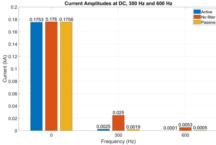
Figure 2.17: FFT Analysis of  $i_{dc,tap}$  at  $P_{dc} = 75 \text{ MW}$  considering different filtering Schemes
