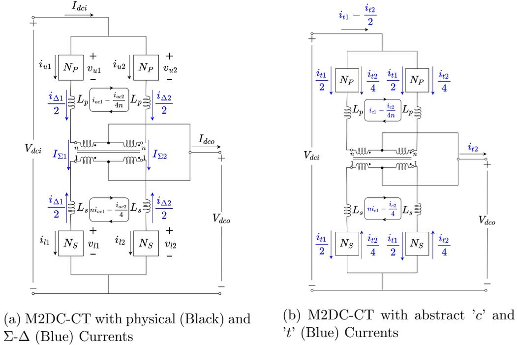
Figure 2.7: M2DC-CT with different current configurations
