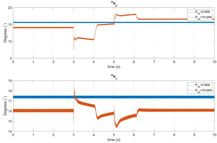
Figure 4.11:  $\alpha_{R_p}$  and  $\alpha_{R_n}$  variations during an MVDC bus DC Fault at positive pole tapping station
