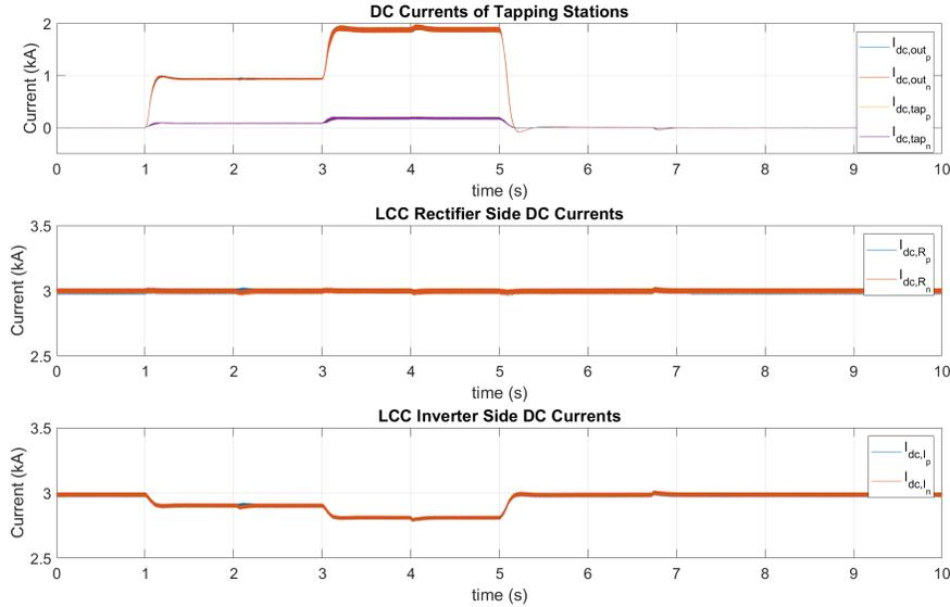
Figure 3.5: DC Currents Variations during Symmetrical Tapping,  $P_{dc,p} = P_{dc,n}$
