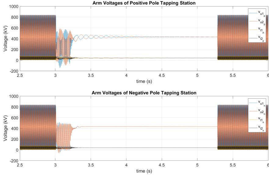
Figure 4.26: Tapping Stations Arm Voltages when  $P_{dc,p} = P_{dc,n} = 0$  MW during an Asymmetrical AC Fault
