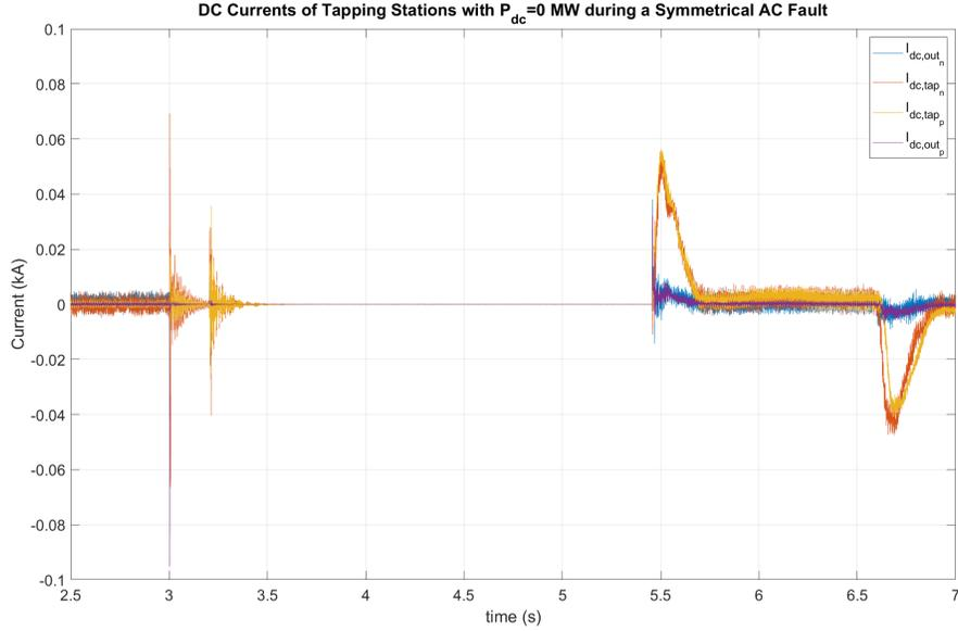
Figure 4.19: Tapping Stations Input and Output DC Currents during a Symmetrical Fault with  $P_{dc,p} = P_{dc,n} = 0 \text{ MW}$
