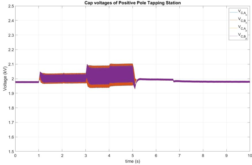
Figure 3.9: Capacitor Voltages of SMs in the Positive Pole Tapping Station where  $P_{dc,p} = P_{dc,n}$
