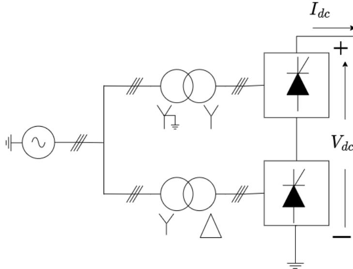
Figure 2.3: Classical 12-Pulse LCC arrangement
