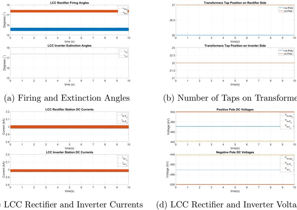
Figure 3.3: Steady State Results for LCC System with  $P_{dc}$  set at  $0\text{ MW}$  at each pole
