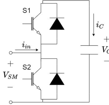
Figure 2.5: Half Bridge Submodule [34]
