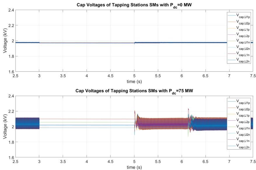
Figure 4.7: SMs capacitor voltage variations during an HVDC DC link Fault
