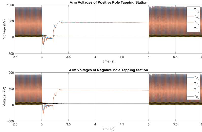
Figure 4.34: Arm Voltage Variations of Tapping Stations during a Three phase AC Fault at the Inverter Station with pre-fault loading scenario  $P_{dc,p} = P_{dc,n} = 0 \text{ MW}$
