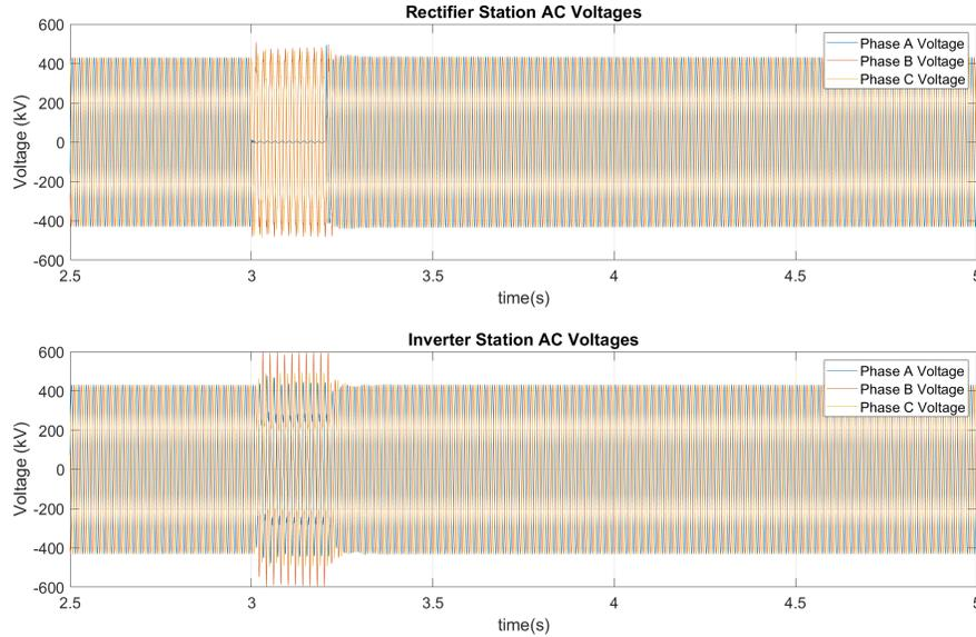
Figure 4.21: AC Network Voltages of LCC-HVDC System under a Single line-to-ground Fault at the Rectifier Station
