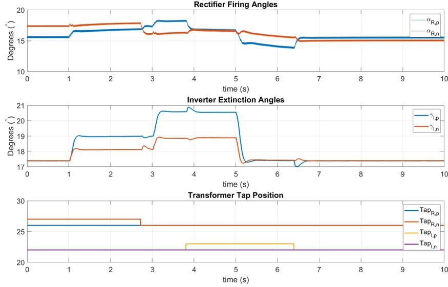
Figure 3.11: Firing Angles, Extinction Angles and Transformer Taps of the LCC Bipole HVDC System,  $P_{dc,p} = 2P_{dc,n}$
