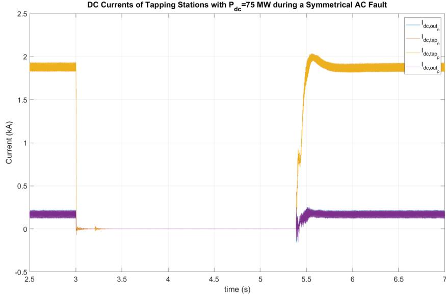
Figure 4.28: Tapping Stations DC Currents during a Symmetrical AC Fault when  $P_{dc,p} = P_{dc,n} = 75 \text{ MW}$
