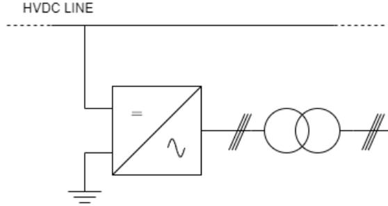
Figure 1.4: AC Tapping using parallel connection [24]
