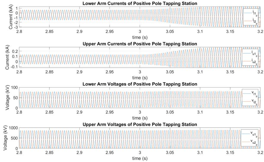
Figure 3.8: Arm Currents and Voltages of Positive Pole Tapping Station M2DC-CT,  $P_{dc,p} = P_{dc,n}$  for  $2.8 \leq t \leq 3.2$
