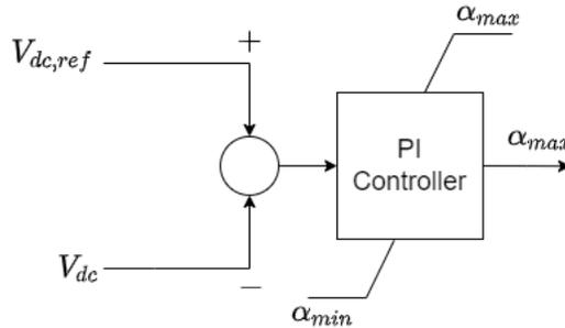
Figure 2.12: Voltage Control Amplifier [35]
