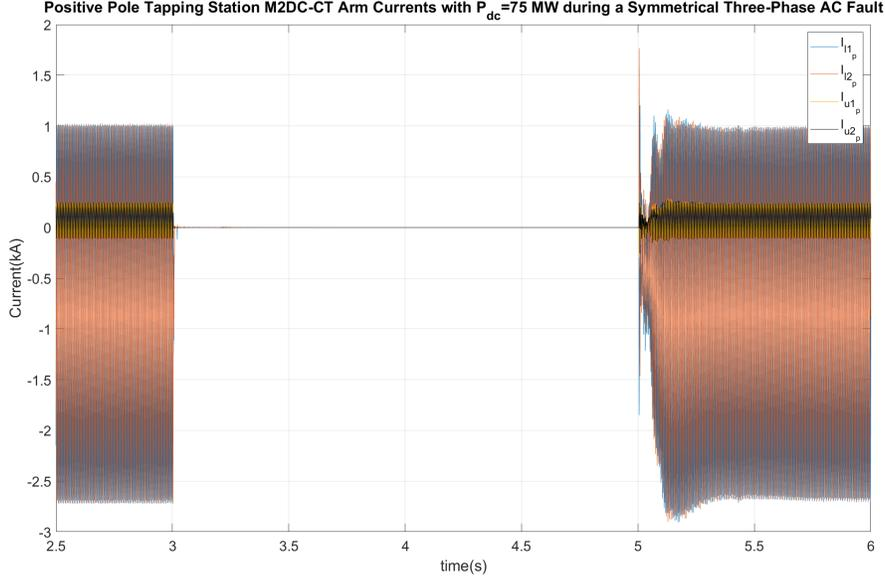
Figure 4.29: Positive Pole Tapping Station M2DC-CT Arm Currents during a Symmetrical AC Fault when  $P_{dc,p} = P_{dc,n} = 75 \text{ MW}$
