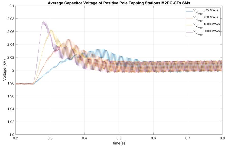
Figure 3.22: Average Capacitor Voltages of Positive Pole Tapping Station M2DC-CTs SMs for different power ramp rates
