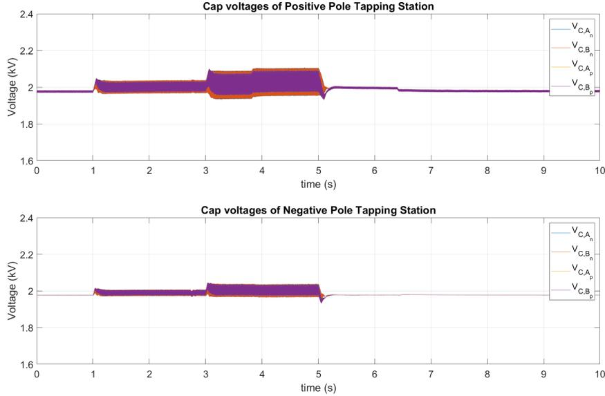
Figure 3.14: Capacitor Voltages of SMs in the Tapping Stations,  $P_{dc,p} = 2 \times P_{dc,n}$
