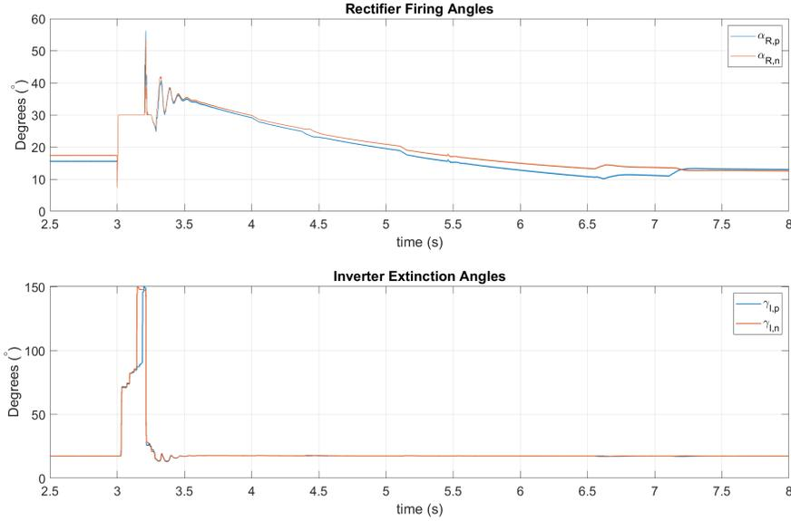
Figure 4.18: Firing and Extinction Angles Variation during a Symmetrical AC Fault
