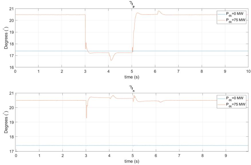
Figure 4.12:  $\gamma_{R_p}$  and  $\gamma_{R_n}$  variations during an MVDC bus DC Fault at positive pole tapping station
