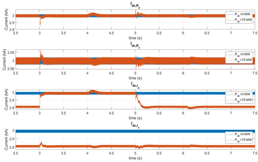
Figure 4.8: LCC-HVDC Bipole System DC Currents variations during an MVDC bus DC Fault at positive pole tapping station
