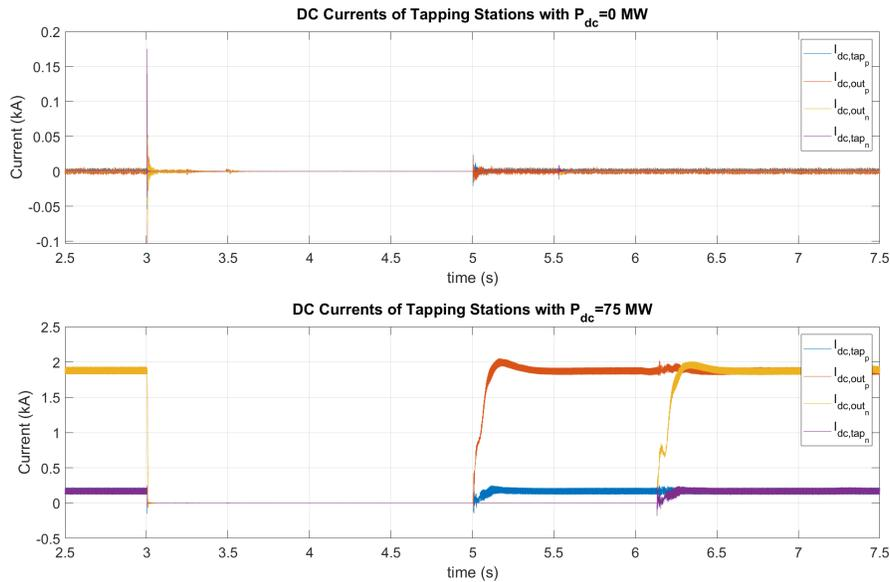
Figure 4.6: Tapping Stations DC Input and Output Currents during an HVDC DC link Fault
