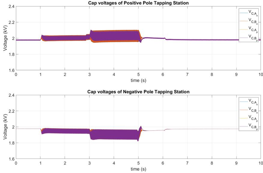
Figure 3.19: Capacitor Voltages of SMs in the Tapping Stations when  $P_{dc,p} = -P_{dc,n}$
