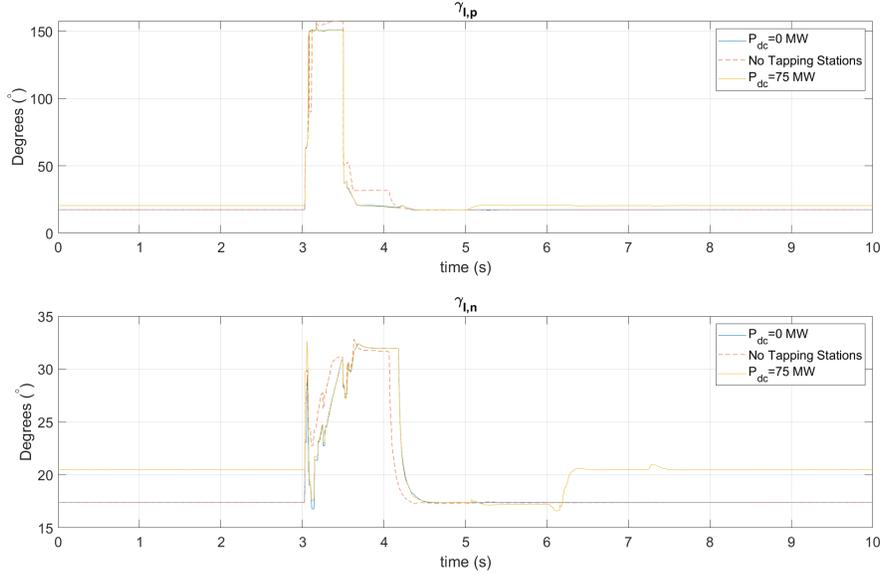
Figure 4.5: Inverter Stations  $\gamma$  variation in different pre-fault loading scenarios
