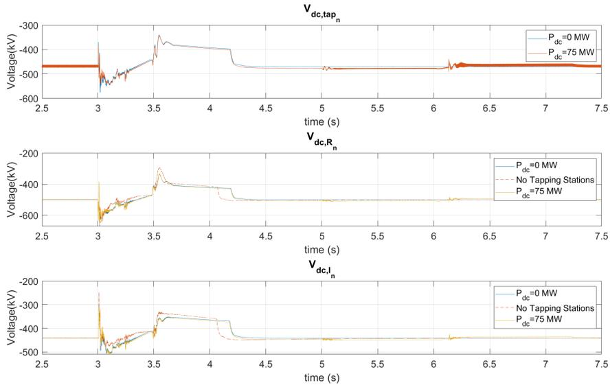
Figure 4.3: Negative Pole DC Voltages Variation during positive pole HVDC-link DC Fault for different pre-fault loading scenarios
