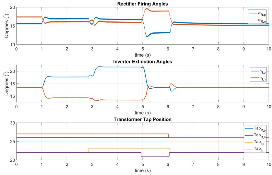
Figure 3.16: Firing Angles, Extinction Angles and Transformer Taps of the LCC Bipole HVDC System when  $P_{dc,p} = -P_{dc,n}$
