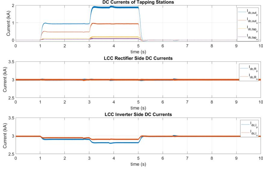
Figure 3.10: DC Currents Variations during asymmetrical Tapping,  $P_{dc,p} = 2 \times P_{dc,n}$
