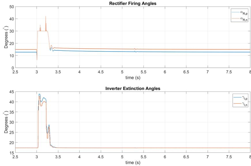
Figure 4.24: Rectifier Firing Angles and Inverter Extinction Angles during an Asymmetrical AC Fault
