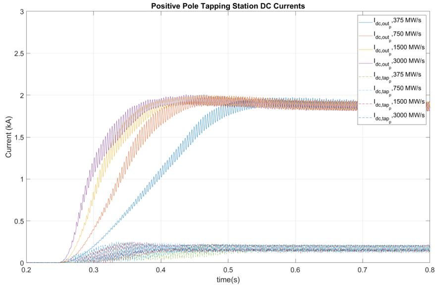
Figure 3.21: Positive Pole Tapping Station M2DC-CT Input and Output DC Currents for different power ramp rates
