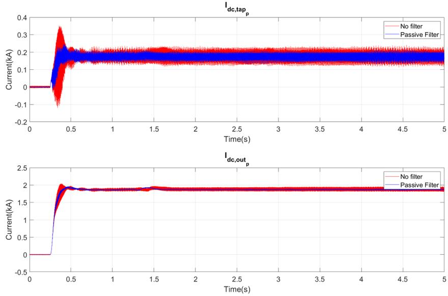
Figure 2.18:  $I_{dc,tap_p}$  and  $I_{dc,out_p}$  for  $P_{dc} = 75 MW$  demand initiated at  $t = 0.25s$
