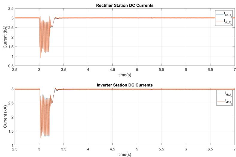
Figure 4.23: LCC-HVDC DC Currents under an Asymmetrical AC Fault
