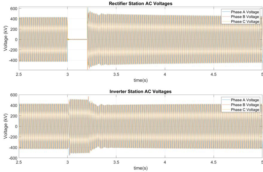
Figure 4.15: Rectifier and Inverter Stations AC network voltages during a Symmetrical AC Fault at the Rectifier
