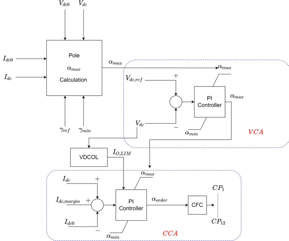
Figure 2.10: LCC Control Structure at inverter stations [35]
