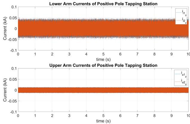
(c) Arm Currents of M2DC-CT at Positive Pole Tapping Station
