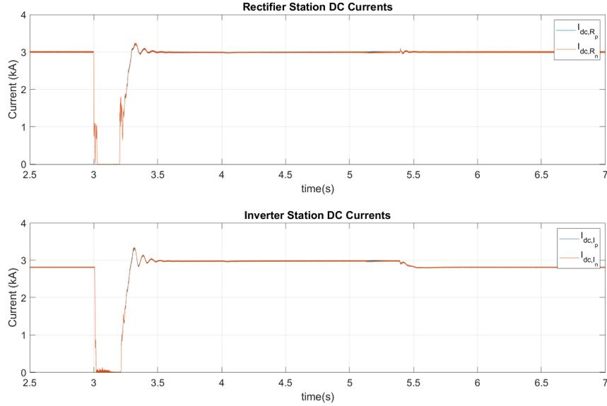
Figure 4.27: LCC-HVDC System DC Currents during a Symmetrical AC Fault when  $P_{dc,p} = P_{dc,n} = 75 \text{ MW}$
