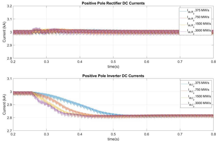
Figure 3.20: LCC-HVDC System Positive Pole DC Currents for different power ramp rates
