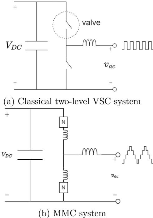
Figure 1.2: VSC operating principle for single phase leg
