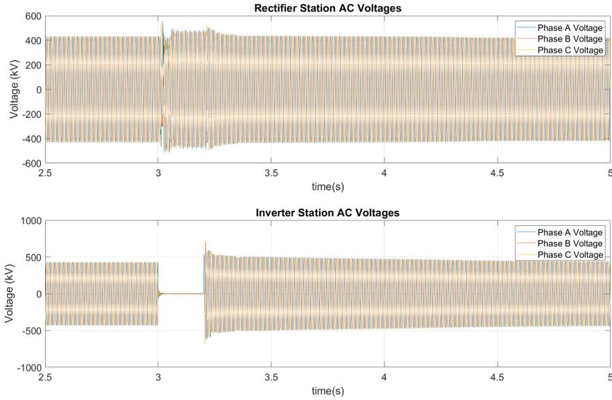
Figure 4.30: AC Network Voltages of LCC-HVDC System during a Three phase AC Fault at the Inverter Station with pre-fault loading scenario  $P_{dc,p} = P_{dc,n} = 0 \text{ MW}$
