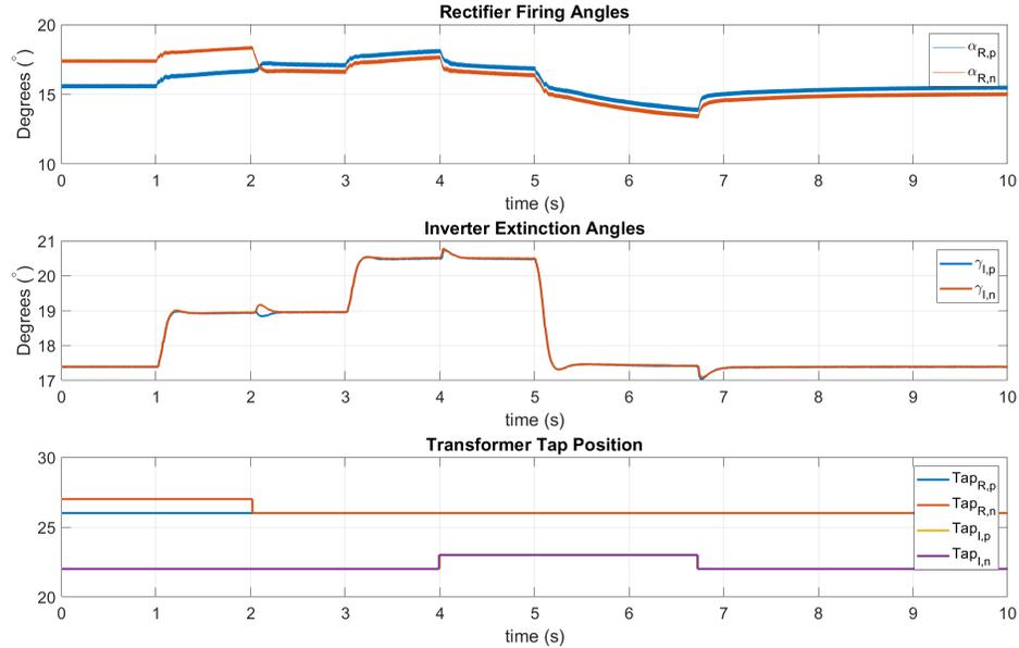
Figure 3.6: Firing Angles, Extinction Angles and Transformer Taps of the LCC Bipole HVDC System,  $P_{dc,p} = P_{dc,n}$
