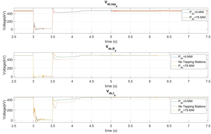
Figure 4.2: Positive Pole DC Voltages Variation during positive pole HVDC-link DC Fault for different pre-fault loading scenarios
