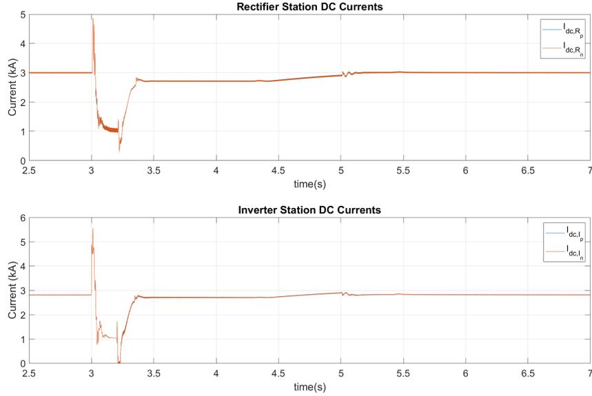
Figure 4.32: DC Currents of LCC-HVDC System during a Three phase AC Fault at the Inverter Station with pre-fault loading scenario  $P_{dc,p} = P_{dc,n} = 0 \text{ MW}$
