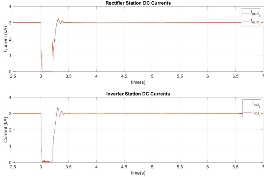
Figure 4.17: LCC-HVDC Bipole System DC Currents variations during a Symmetrical AC Fault
