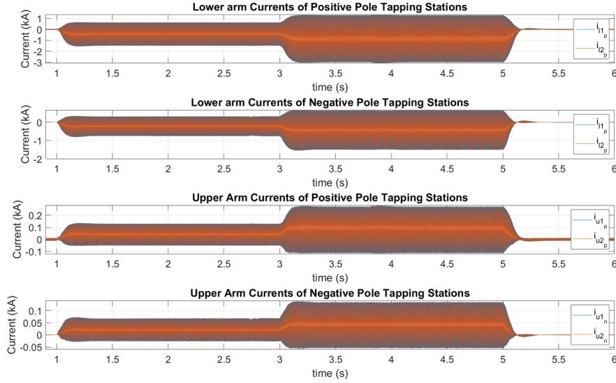
Figure 3.12: Arm Currents of Tapping Stations M2DC-CTs,  $P_{dc,p} = 2P_{dc,n}$
