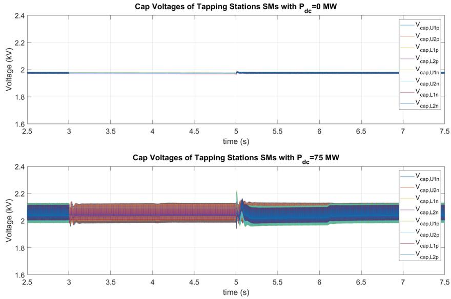
Figure 4.14: SMs capacitor voltage variations during an MVDC bus DC Fault at positive pole tapping station
