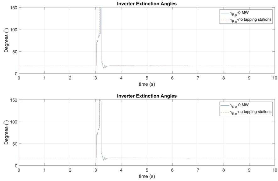
Figure A.2: Comparison of Inverter Extinction Angles with and without the presence of tapping stations
