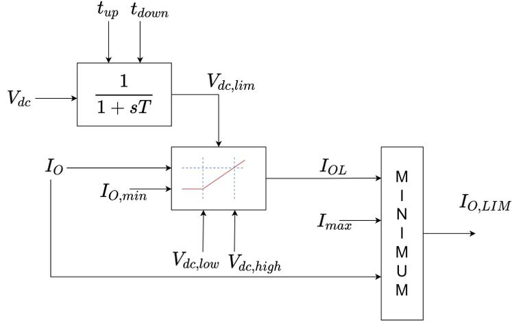
Figure 2.15: Voltage Dependent Current Order Limit Control [35]
