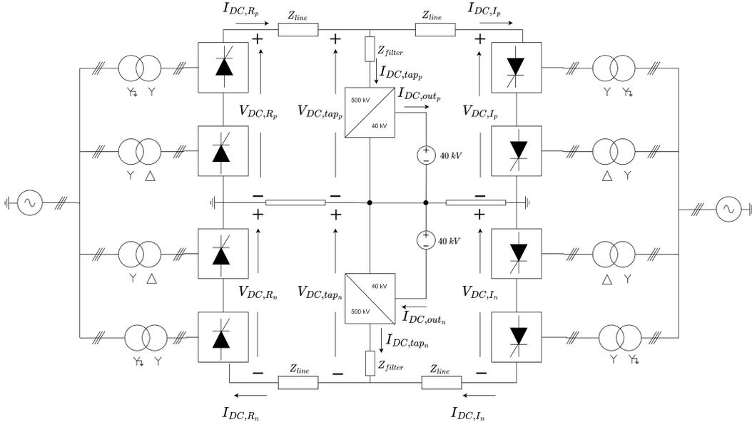
Figure 2.9: LCC Bipole System with MMC-based tapping stations
