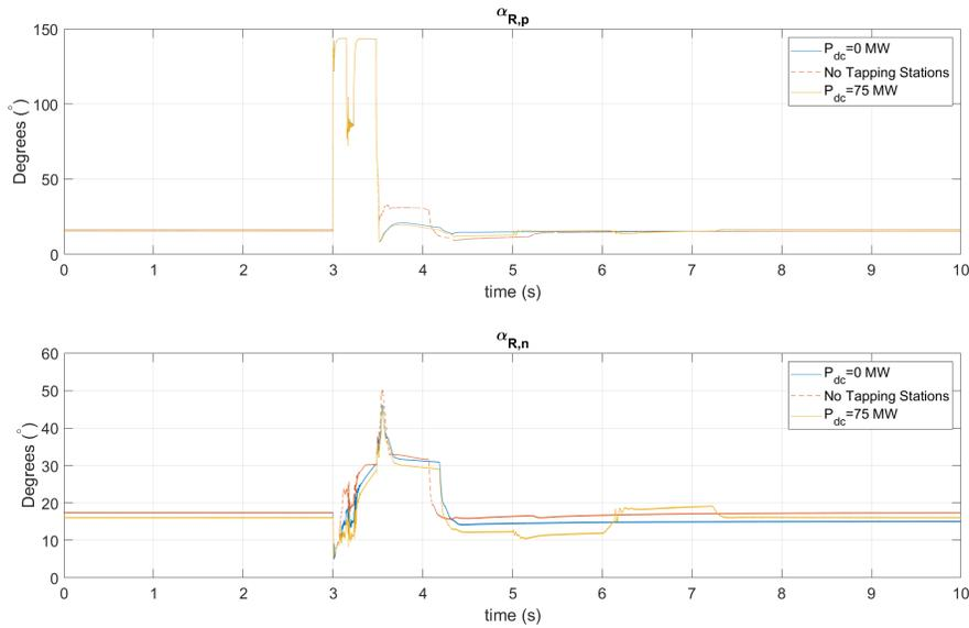
Figure 4.4: Rectifier Stations  $\alpha$  variation in different pre-fault loading scenarios
