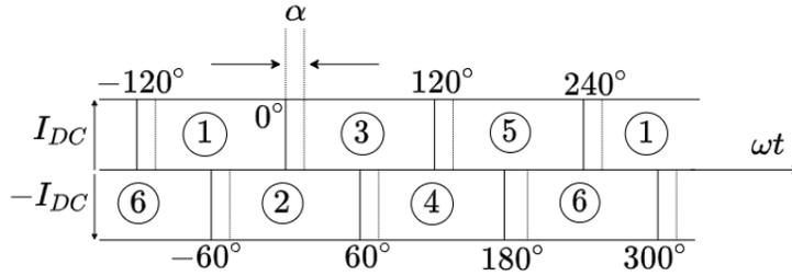
Figure 2.2: LCC Commutation Process [33]
