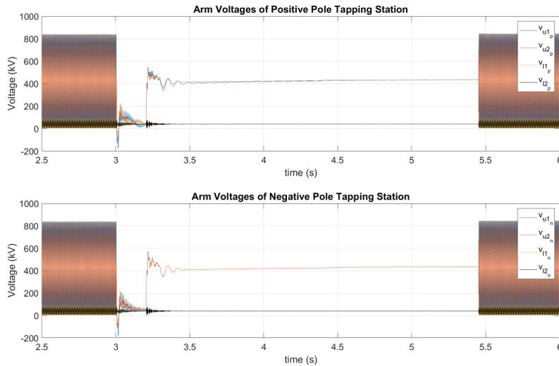
Figure 4.20: Tapping Stations Arm voltages with  $P_{dc,p} = P_{dc,n} = 0 \text{ MW}$  during a Symmetrical AC Fault
