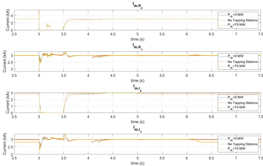
Figure 4.1: LCC-HVDC System DC Currents during a line-to-ground DC Link Fault for different pre-fault loading scenarios
