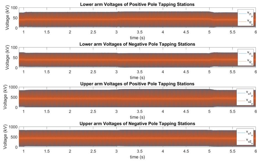
Figure 3.18: Arm Voltages of Tapping Stations M2DC-CTs when  $P_{dc,p} = -P_{dc,n}$
