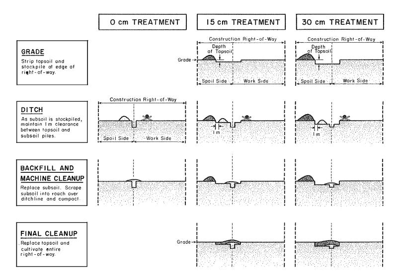
Figure 3. Topsoil and spoil stripping and storage.
