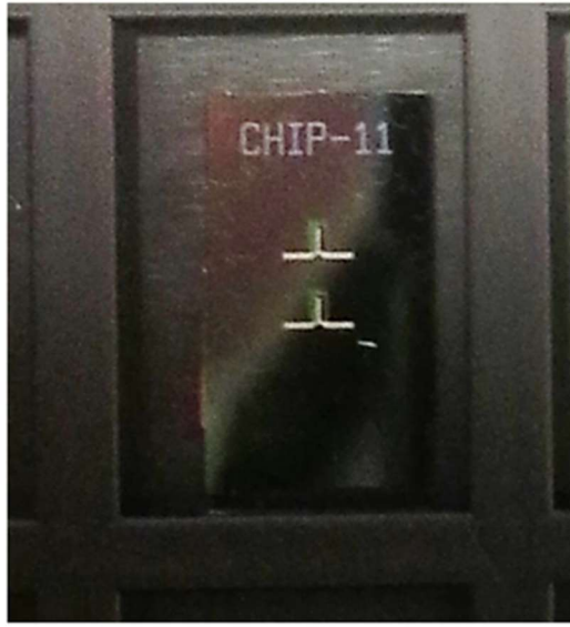
Figure 3.5. A picture of Chip 11 after completion of the fabrication process. This chip contains two microfluidic cantilever devices.
