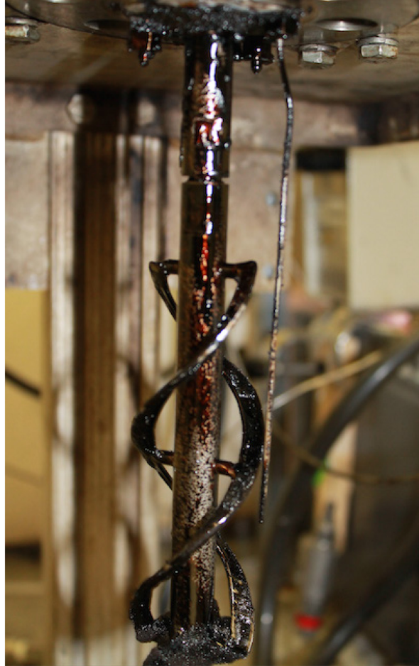
Figure 19. Helical impeller after a dynamic extraction of bitumen with SC-CO 2 (May 2, 2016 extraction).
