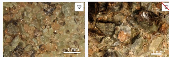
Figure 6. The piece of the sample that went into the SELFRAG (figure on the left) is separated into its individual minerals and is more uniform compared to the sample that underwent conventional disaggregation (figure on the right).
