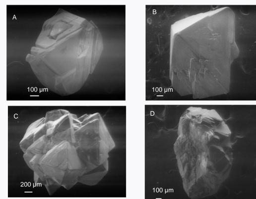
Figure 7. Diamonds released from the SELFRAG imaged with a Scanning Electron Microscope (SEM). Most diamonds liberated showed no signs of visible breakage (Fig 7b,c) but a few show signs of possible damage, although it may have occurred during the kimberlite eruption. (Fig 7a,d).
