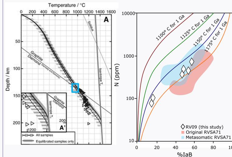
Figure 8. Using Electron Probe Microanalysis (EPMA), we calculated the temperature of the garnets and clinopyroxene at Mg-Fe equilibrium. (6) Then we plotted the point on a Finsch geotherm (7), which indicates that our eclogite lies at the diamond-graphite transition.
