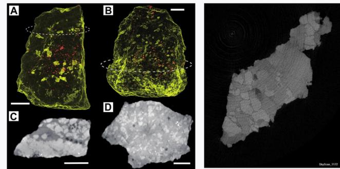
Figure 5. Using methods similar to Ishikawa et al (figure on the left), we probed our sample RV09 for its constituent minerals (figure on right). The brighter areas correspond to garnet, while the larger spots of dark grey are clinopyroxene. The dark spots found on the right are likely diamond. (3)
