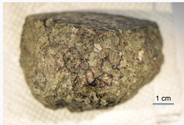
Figure 2. Map of southern Africa detailing the occurrence of major kimberlite pipes within the Kalahari craton. (2) Figure 3. Visible light image of the RV09 sample before it was halved. One half underwent jaw crushing while the other half went into the SELFRAG.
