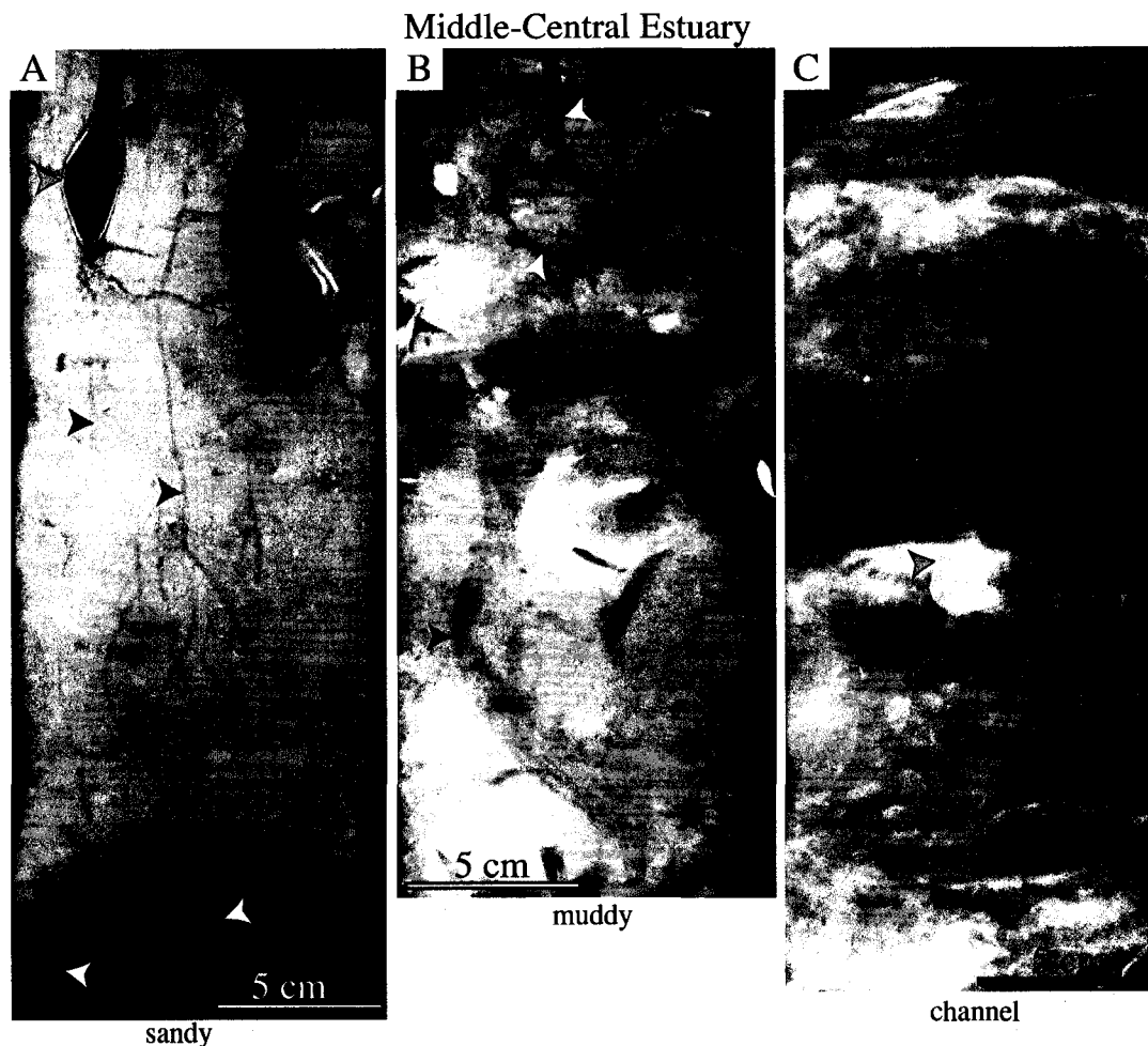
Figure 2.11- X-rays of sediments from the middle-central estuary. A) Sandy deposits from the margins of the middle-central estuary. Primary sedimentary structures are thoroughly reworked by infauna, which consist of Capitella (black arrows) and M. arenaria (grey arrows). The dark colored deposits at the base of the X-ray comprise palimpsest salt-marsh deposits exposed through bay-margin wave activity, subsequently burrowed with Psilonichnus -like structures (white arrows). B) Muddy deposits from the margins of the middle-central estuary. Only vestigial muddy laminations are observed here due to abundant bioturbation. Shell debris and eelgrass debris are common. Distinct burrow structures consist Skolithos -like burrows (white arrows) and Teichichnus -like burrows (black arrow) of Nereis . C) Muddy channel deposits from the middle-central estuary. Primary sedimentary structures are more likely to be preserved here, consisting in this case of ripple-cross lamination (black arrow). The current ripples form exclusively in the fecal pellets of Capitella . The temporally erosive nature of the channel and the resultant exposure of stiffground / firmground is evidenced by the presence of the firmground bivalve Petricola pholadiformis (grey arrow).
