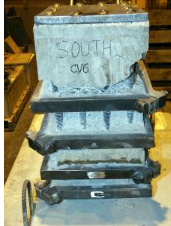
(e) At end of test (No slippage of collars even under significant concrete spalling)
