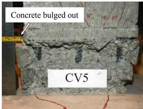
(j) Shear displacement
