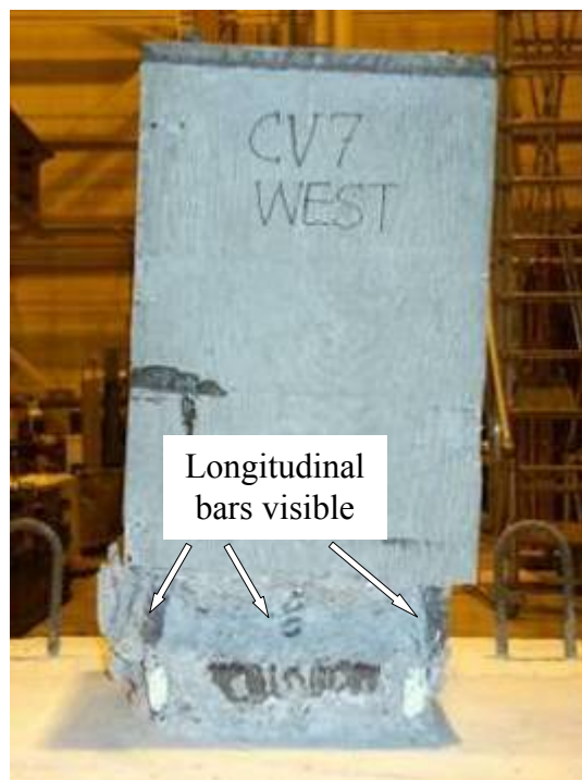
(g) Minor damage except at the bottom (West side)
