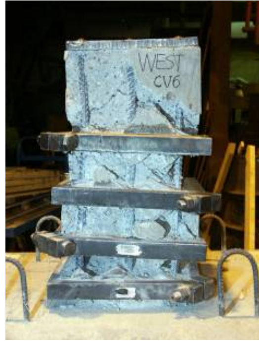
(b) No collar slippage after significant spalling
