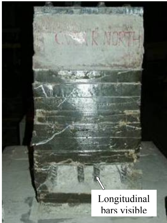
(c) At end of test (North side)
