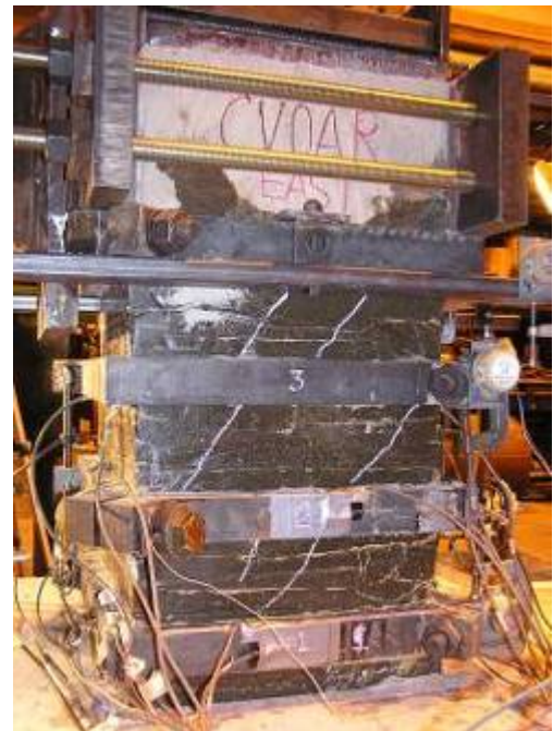
(b) Cracks at cycle 16 ( \mu=2 ) (East side)
