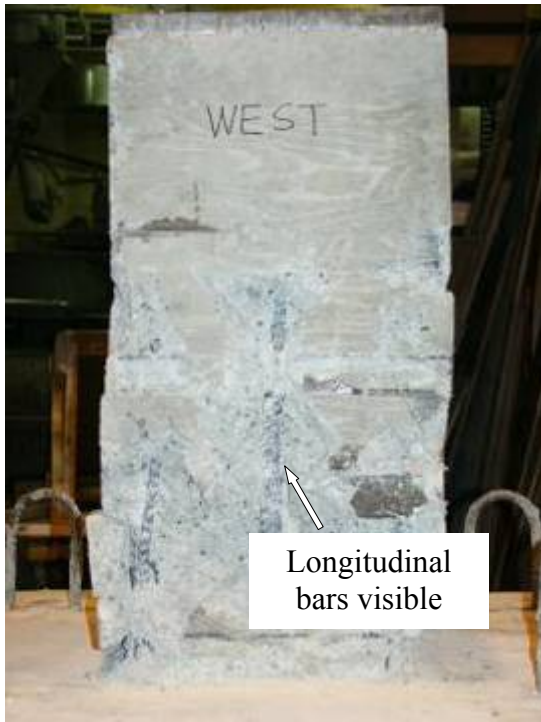
(g) At end of test (West side)
