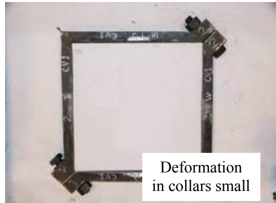
(j) Collars after test (collar 2)
