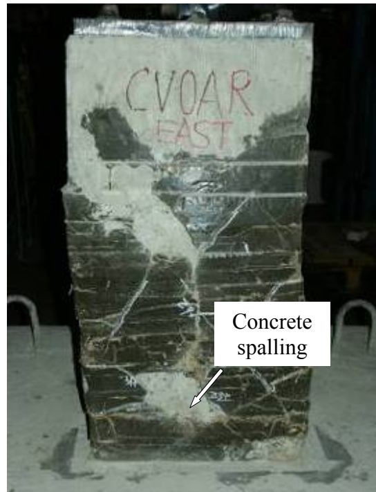
(f) At end of test (East side)
