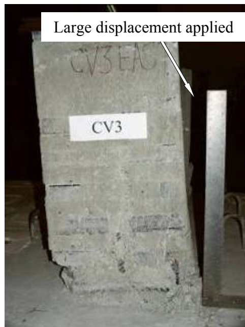
(a) Column sustained large displacement
