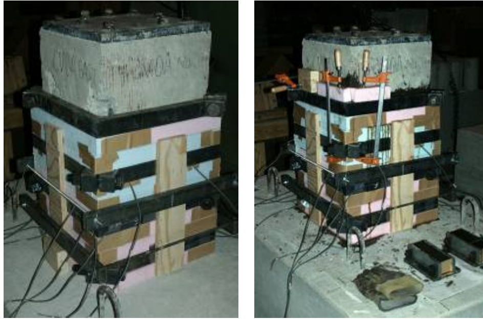
(a) Form and brace system for grout repair (b) After epoxy mortar grout
