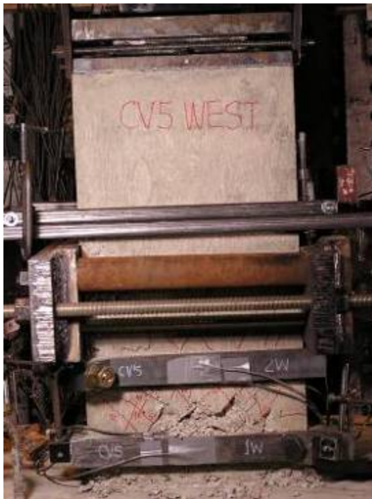
(c) Damage at cycle 26 ( \mu=4.52 ) (West side)
