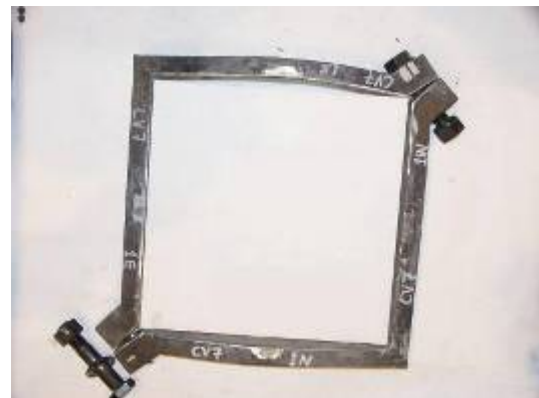
(b) Collar deformation (collar 1)
