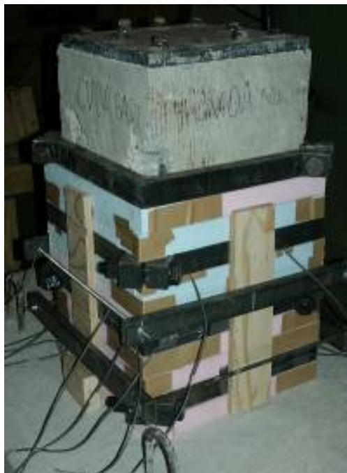
(c) Brace system for form
