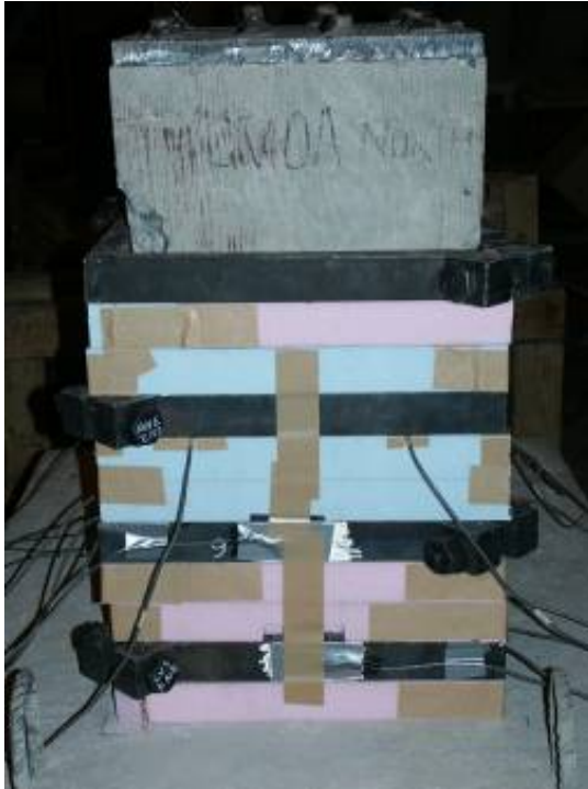
(a) Form for grout
