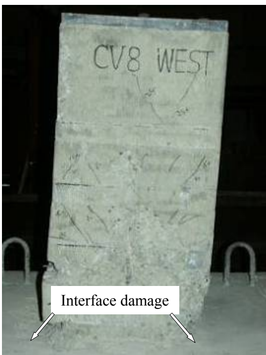
(e) At end of test (West side)
