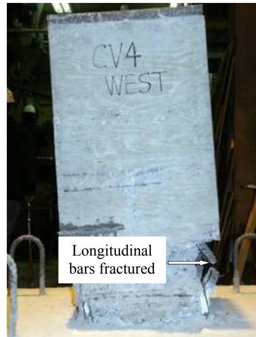
(b) At the end of the test
