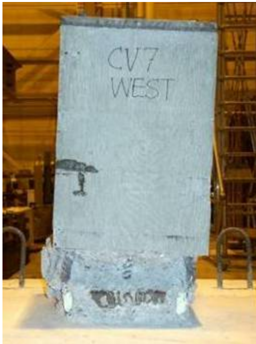
(a) Minor damage even at the end of the test
