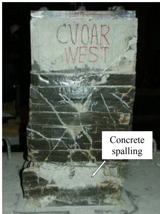
(e) At end of test (West side)
