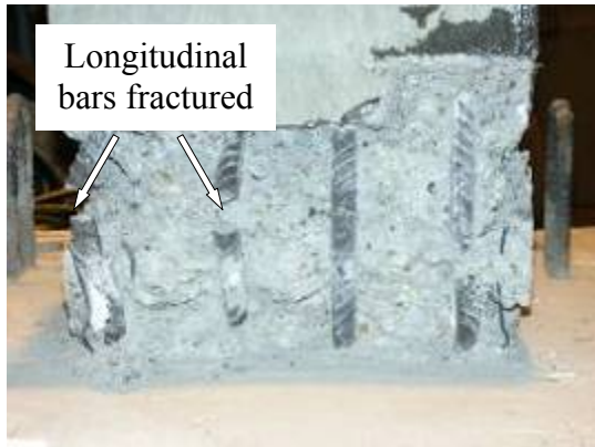
(g) Fracture of bars (South side)
