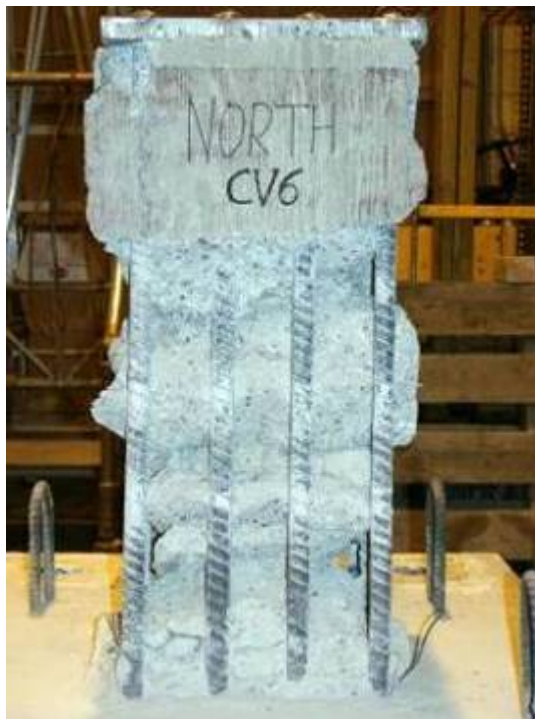
(f) At end of test (North side)
