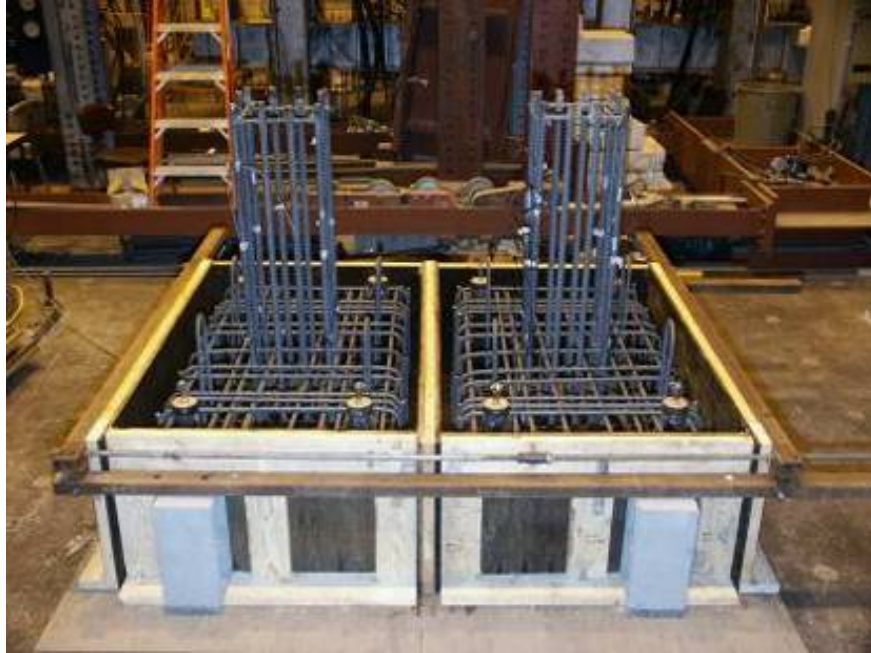
Figure 3-7 Two specimens ready for concrete casting of footings
