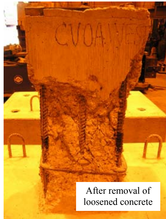
(b) At the end of the test
