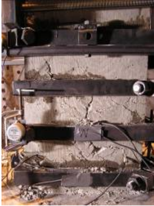
(a) Cracks at cycle 16 ( \mu=4 )
