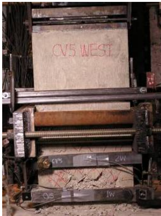
(a) Damage at cycle 26 ( \mu=4.52 )
