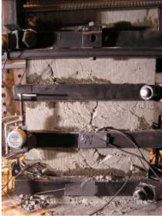
(a) Cracks at cycle 16 ( \mu=4 ) (West side) (b) Damage at cycle 18 ( \mu=4 ) (West side)
