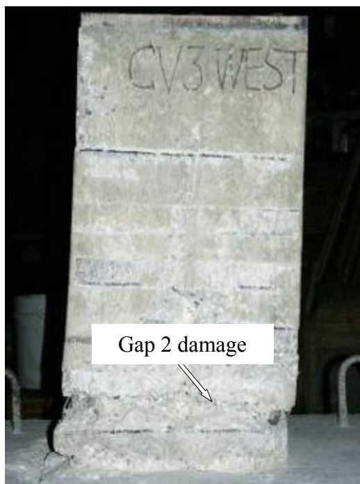
(g) At end of test (West side)
