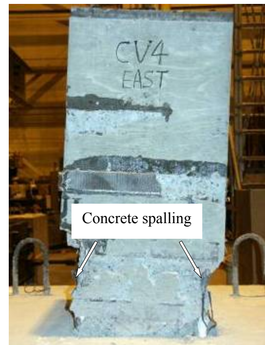
(f) At end of test (East side)
