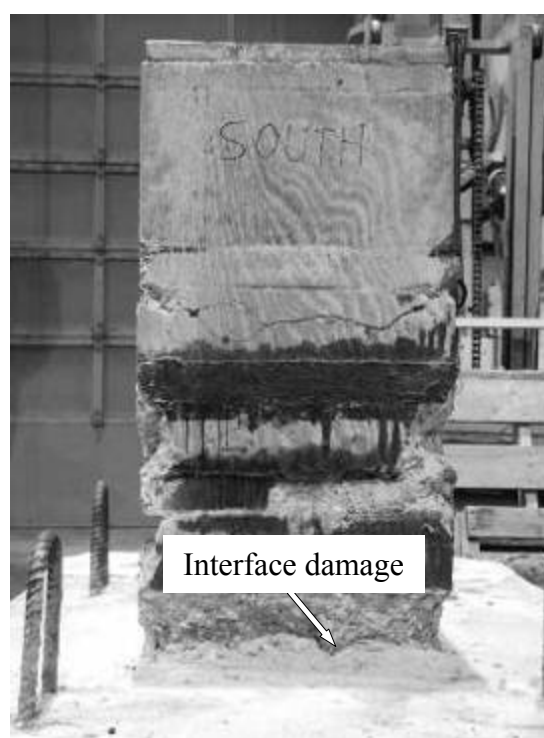
(f) At end of test (South side)
