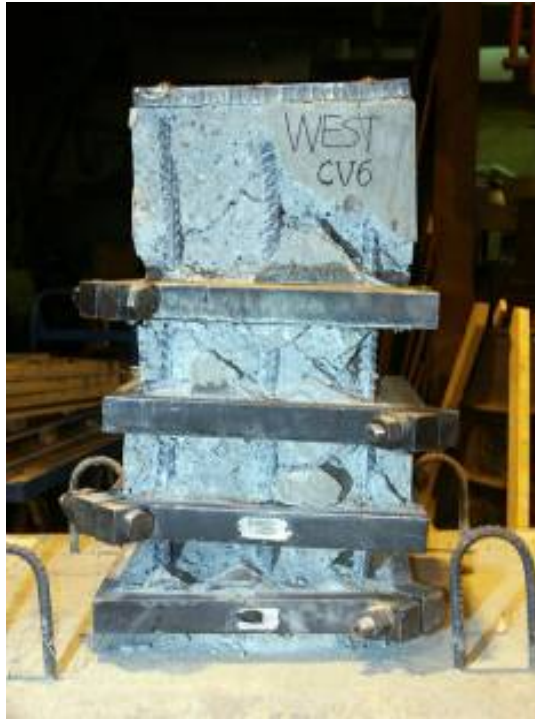
(e) At end of test (No slippage of collars even under significant concrete spalling)
