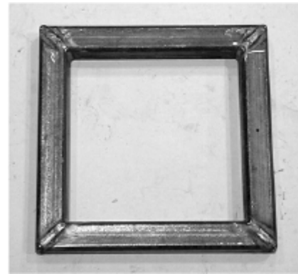
(b) Welded steel HSS collars
