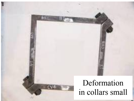
(h) Collar after test (collar 1)
