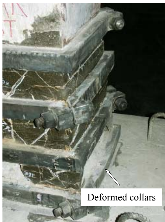
(g) End of test-bending of collars (South side) (h) Crushing (Southwest corner at cycle 52)
