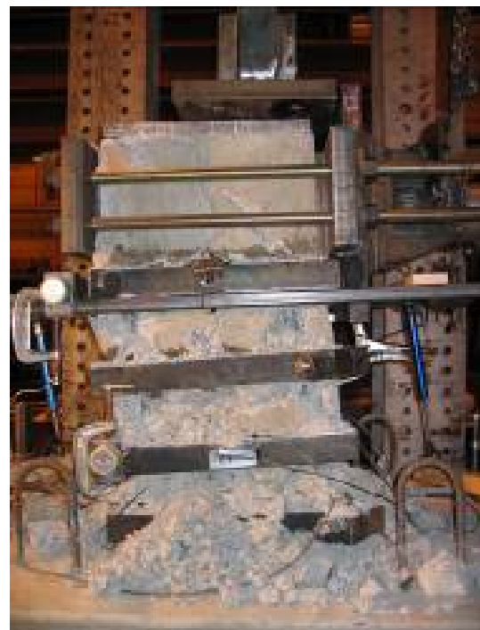
(c) Damage at cycle 21 ( \mu=6 ) (West side) (d) Damage at cycle 26 ( \mu=7 ) (West side)
