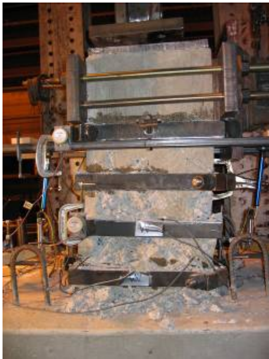
(c) Damage at cycle 21 ( \mu=6 ) (West side) (d) Damage at cycle 26 ( \mu=7 ) (West side)
