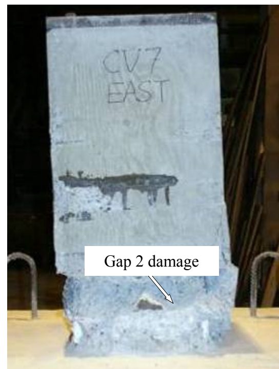
(h) At end of test (East side)
