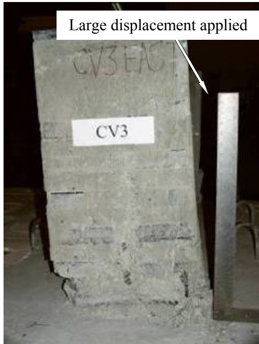
(c) Column sustained large displacement (d) Damage at the interface (North side)
