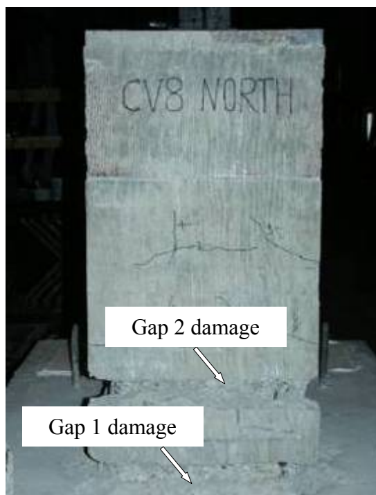
(c) At end of test (North side)
