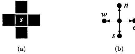
Figure 4.2: A small structure (a) and its edge-oriented assembly graph (b). The edges of the graph in (b) have been marked with their directions.
