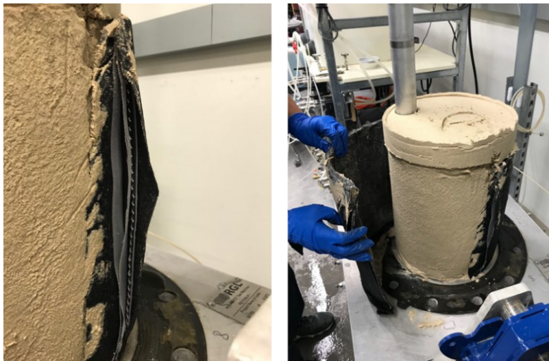
Figure 4-19. The photo illustration of the sand sample surface with the new mesh
