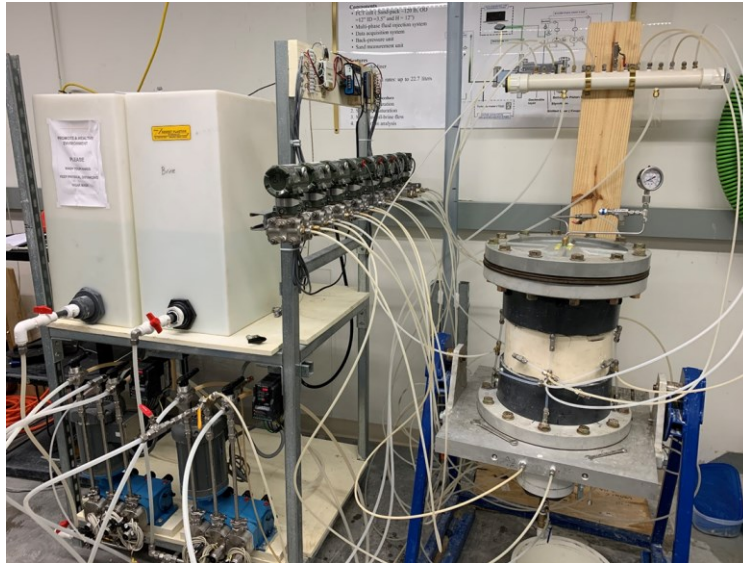
Figure 3-11. The photo illustration of the fluid injection system in the horizontal position
