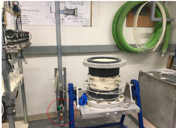
Figure 4-14. The photo illustration of the pressure regulator in the system, as highlighted in the red circle
