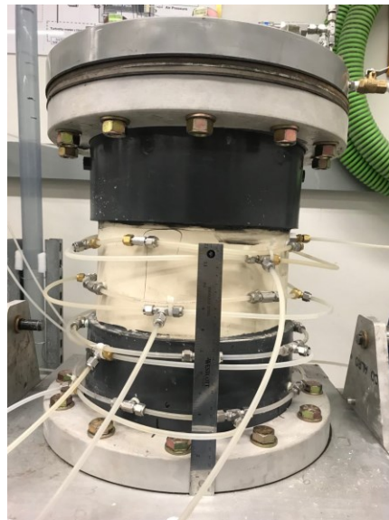
Figure 3-10. The photo illustration of the fluid injection ports in the vertical FCT test
