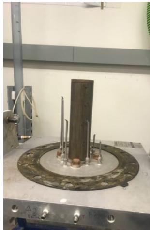
Figure 3-8. The photo illustration of the base plate with the slotted liner
