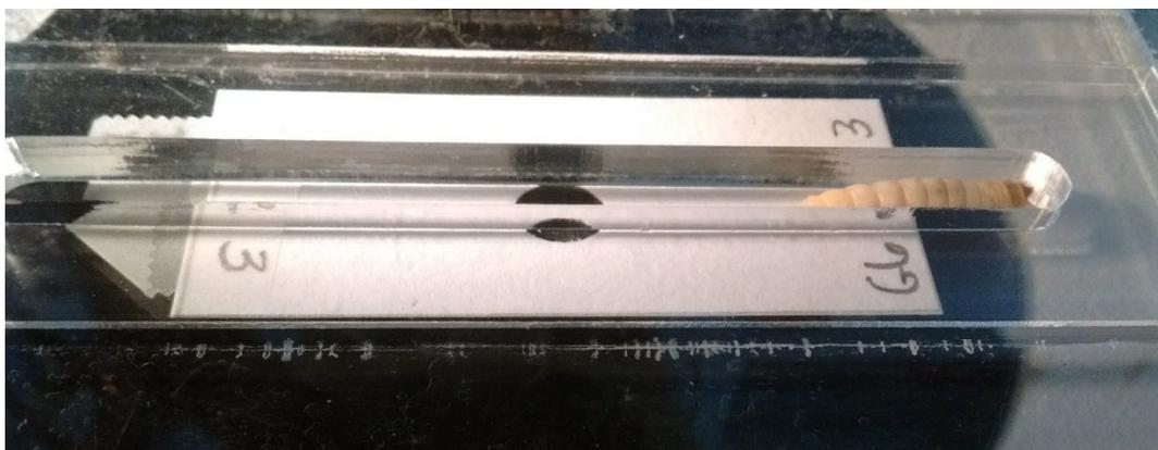
Figure 3.8 The acrylic holder with mounted paper tab and *Galleria* larva walking along the channel.
