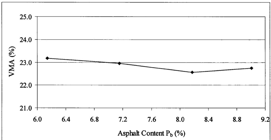
**Figure 4.15 Relationship between asphalt content and VMA for dense-graded ARM**
