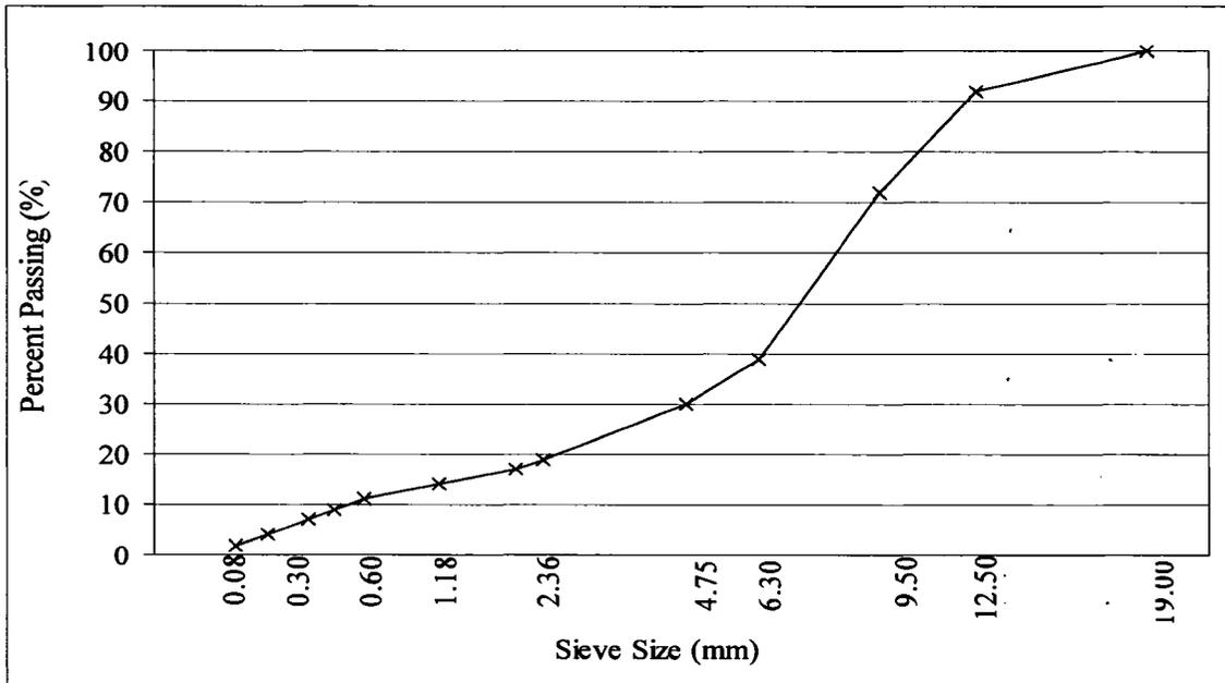
Figure 3.7 Aggregate gradation for the ARM design (Highway 623:03)
