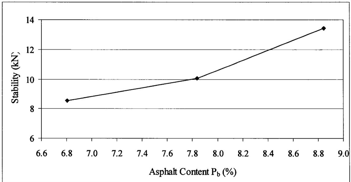
**Figure 4.7 Relationship between asphalt content and stability for open-graded ARM**
