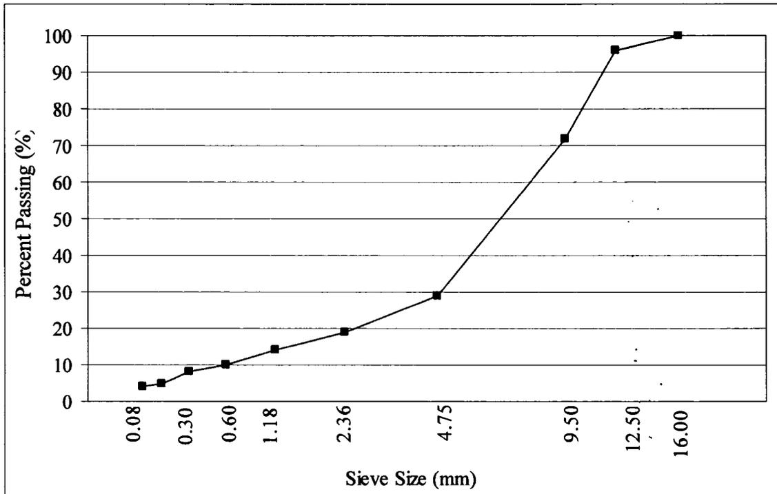
**Figure 3.3 Aggregate Gradation for Calgary aggregate gradation**
