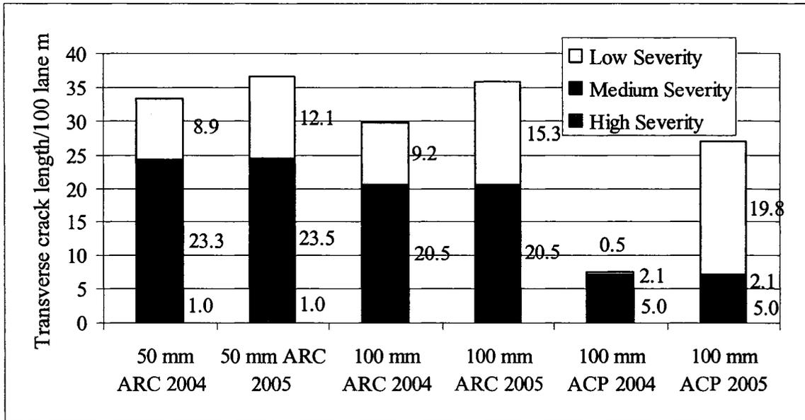
**Figure 3.17 Transverse crack measurements at 137 Avenue project locations**
