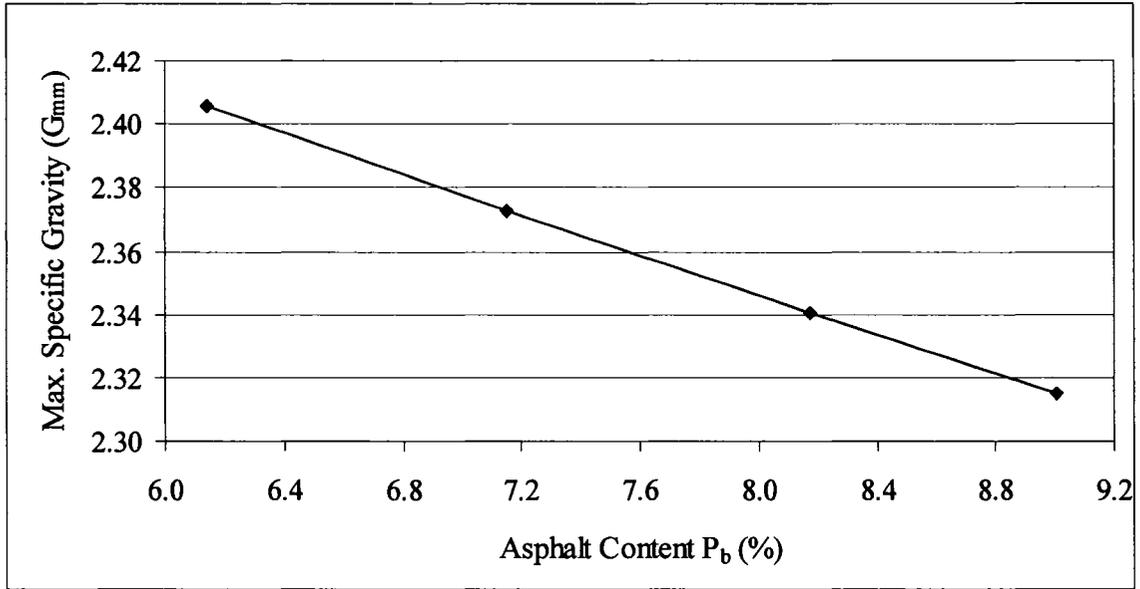
**Figure 4.12 Relationship between asphalt content and maximum specific gravity for dense-graded ARM**
