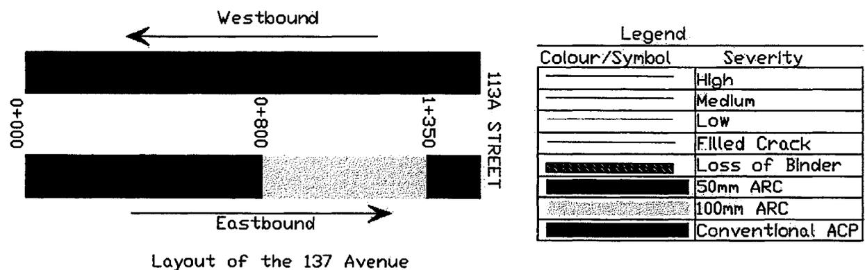
**Figure 3.19 Crack measurements at 137 Avenue project location**
