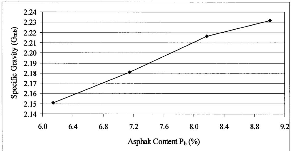
**Figure 4.11 Relationship between asphalt content and specific gravity for dense gradation
