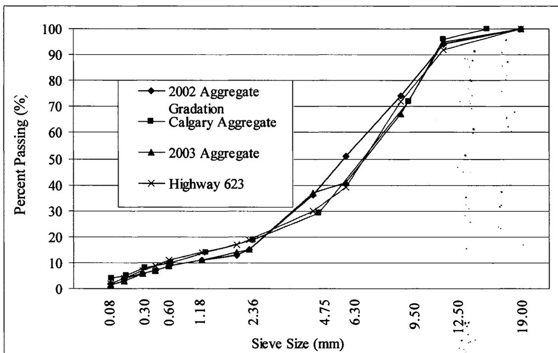
Figure 3.9 Aggregate gradation for 2002 and 2003 Alberta Asphalt Rubber project
