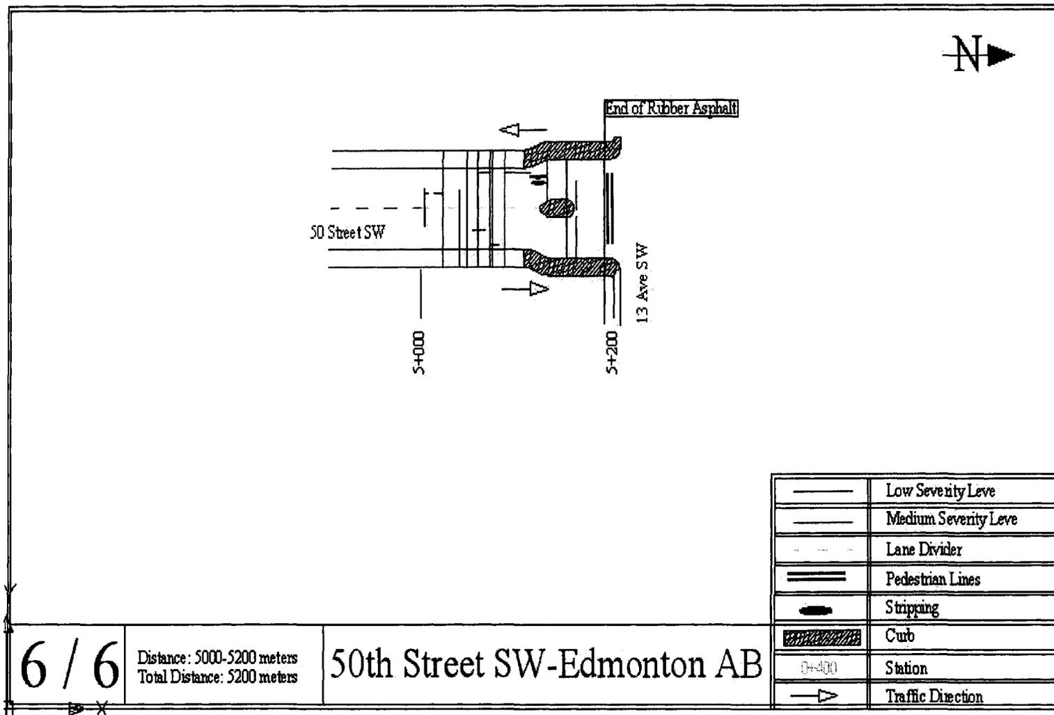
Figure 3.28F Crack measurements map at the 50 Street project locations (5000-5200 m)
