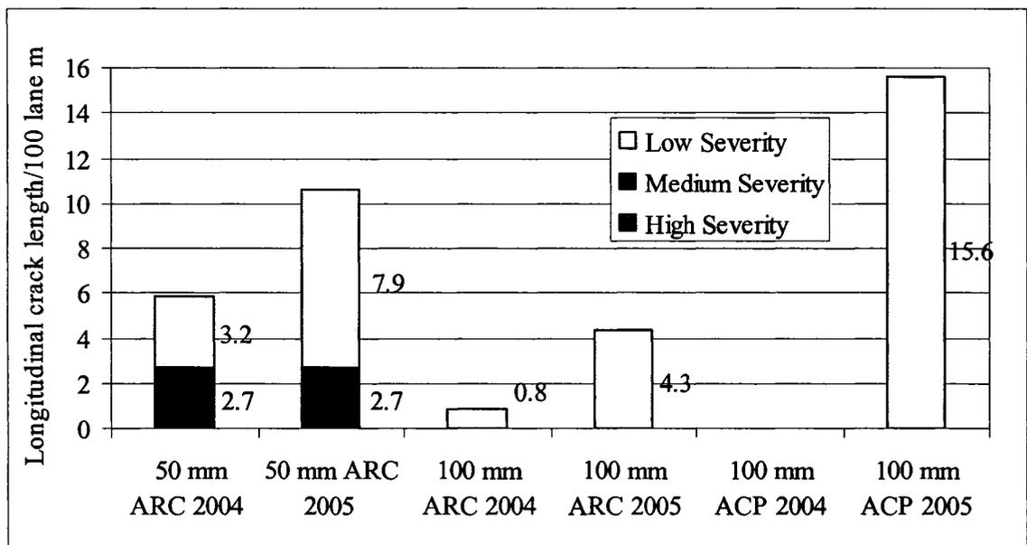
**Figure 3.18 Longitudinal crack measurements at 137 Avenue project locations**
