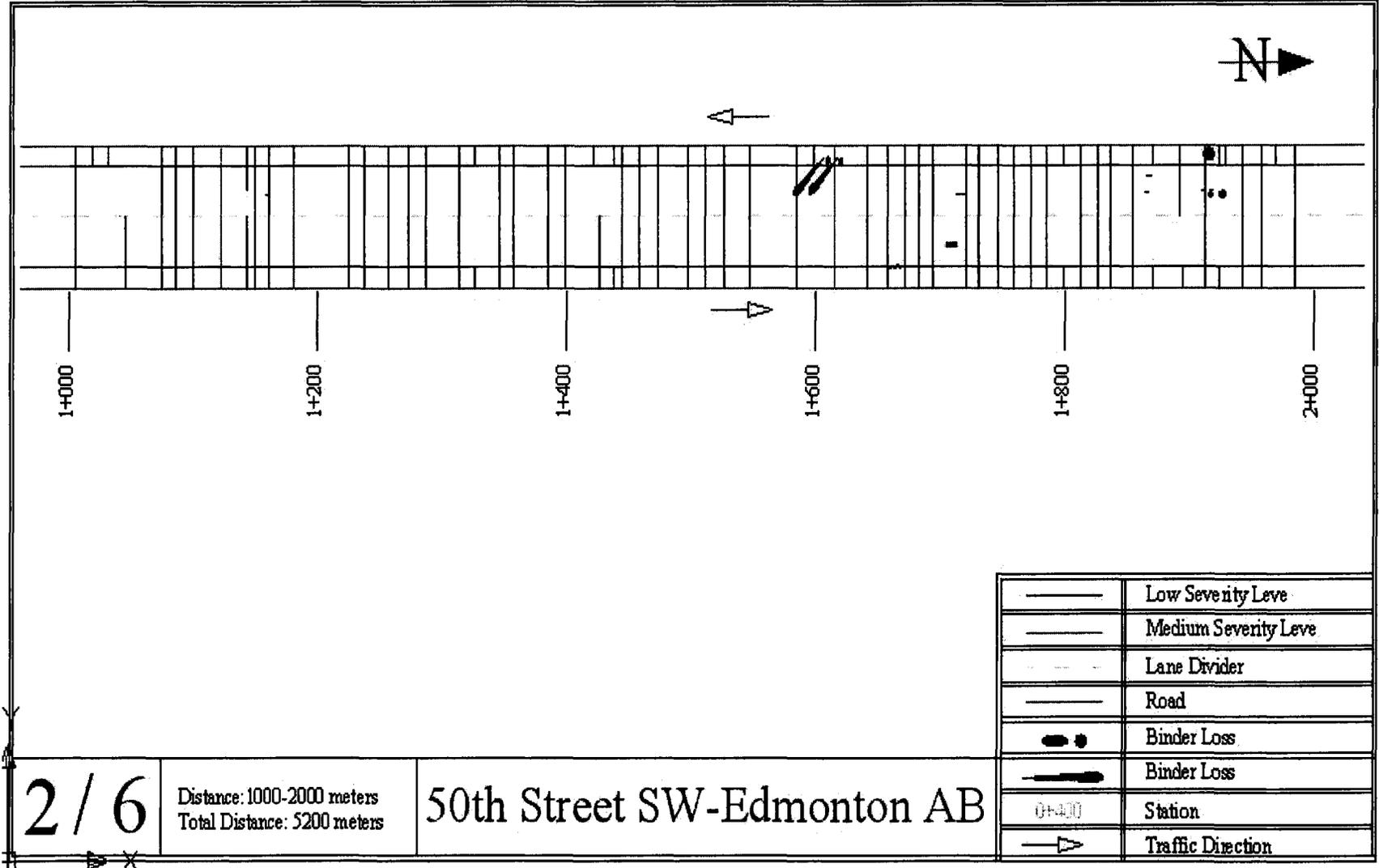
Figure 3.28B Crack measurements map at the 50 Street project locations (1000-2000 m)
