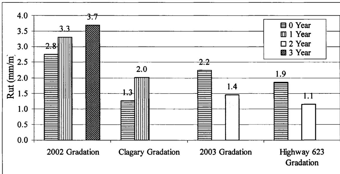
**Figure 3.44 Comparison of the Rut for different aggregate gradation used in 2002 and 2003 AR project**
