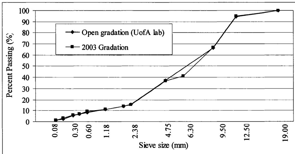
**Figure 4.2 Comparison of the 2003 gradation and lab prepared open gradation**
