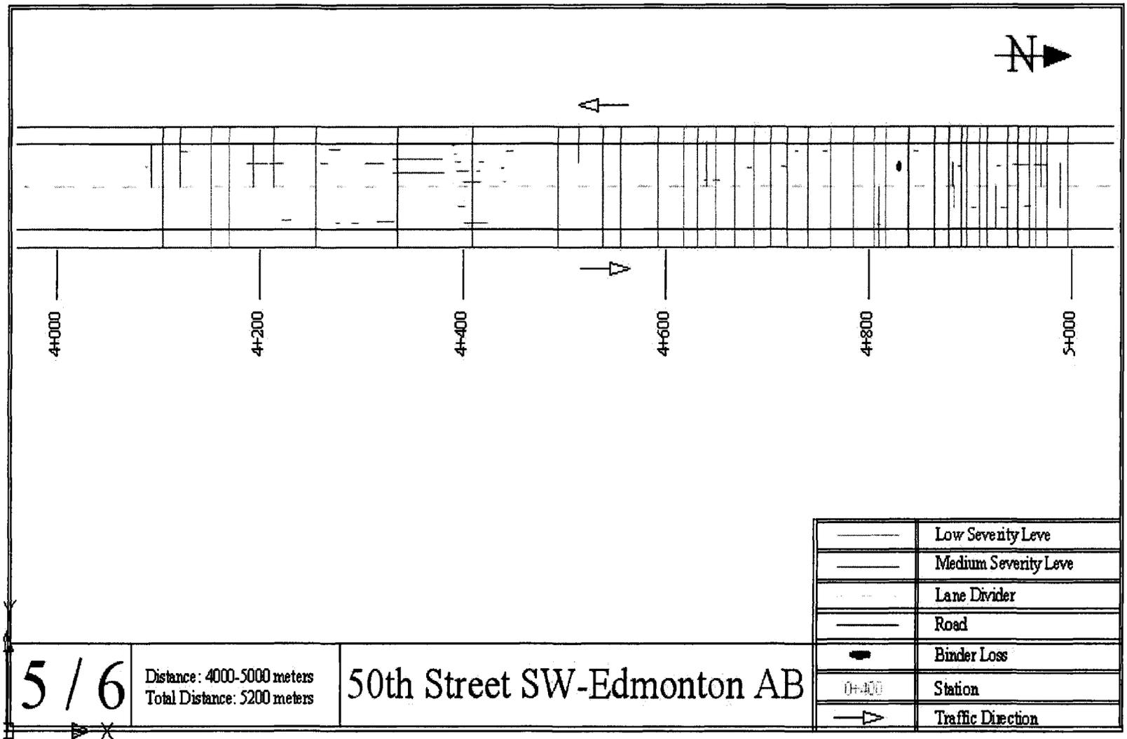
Figure 3.28E Crack measurements map at the 50 Street project locations (4000-5000 m)
