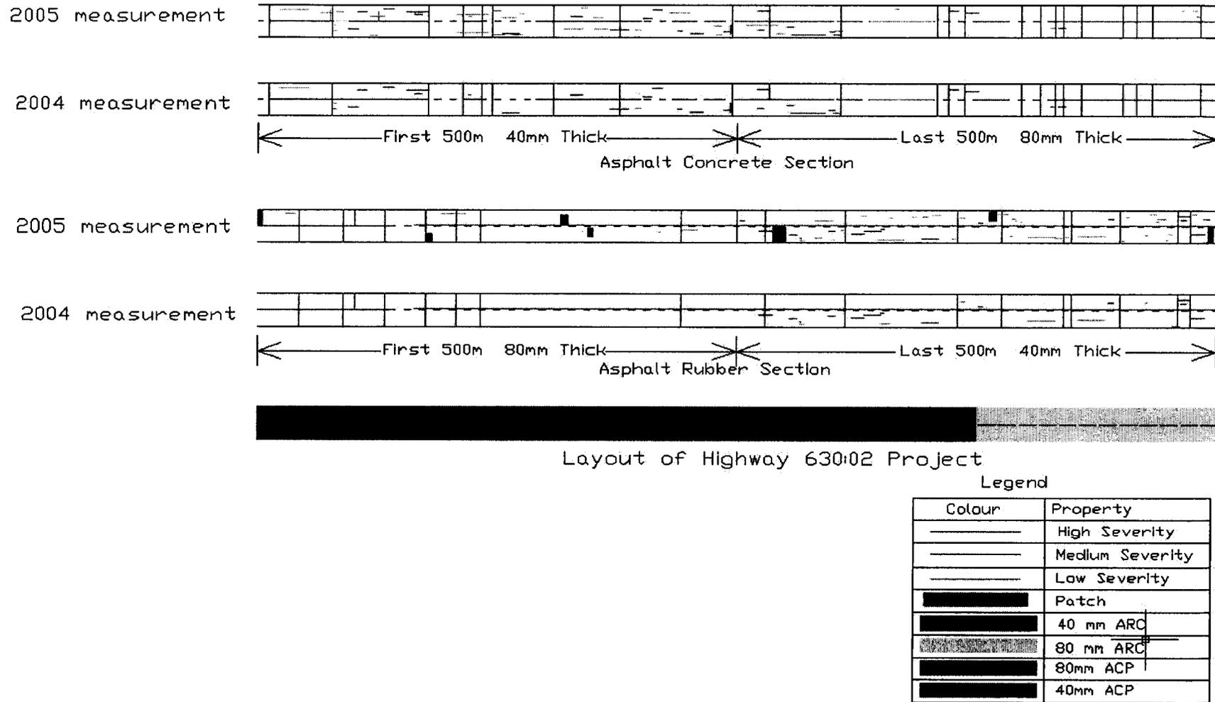
**Figure 3.22 Crack measurement map at Highway 630:02 project location**
