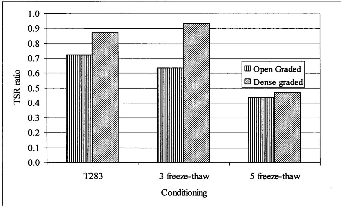
**Figure 4.17 Results of moisture sensitivity test on open and dense-graded aggregate gradation**
