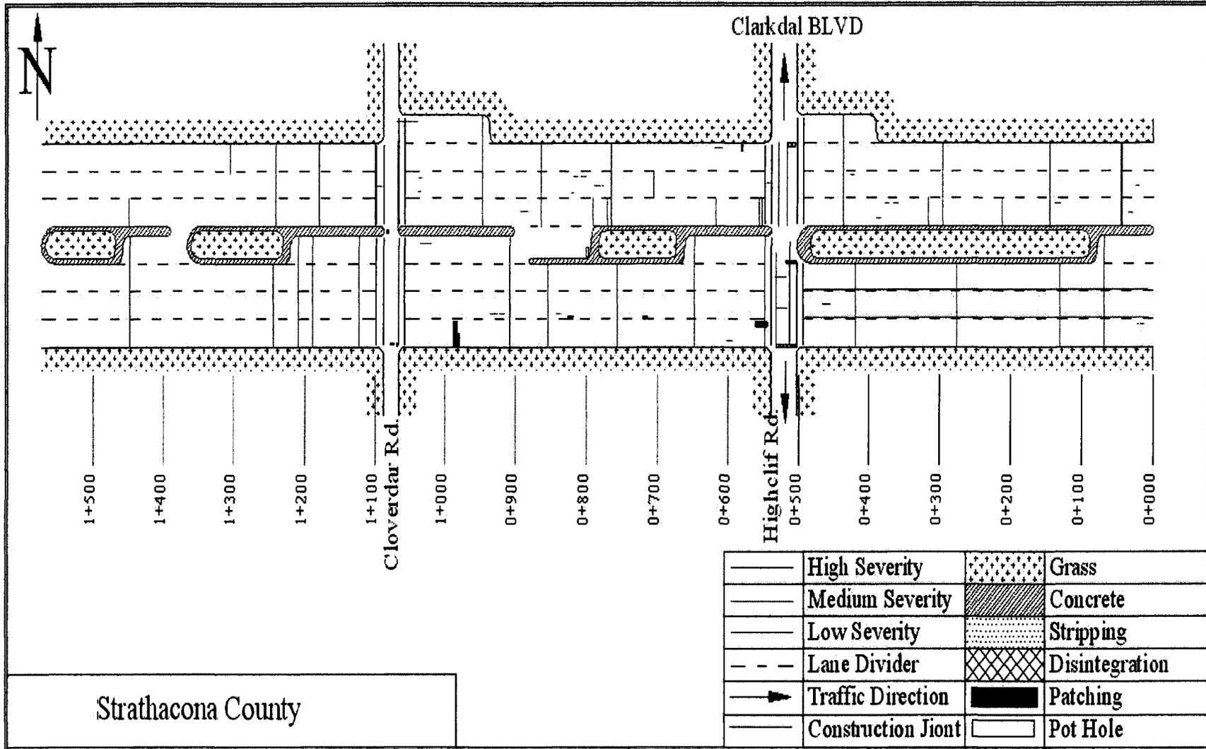
Figure 3.37 Crack measurements map at the Baseline Road (Chelsea Way to Highway 21)
