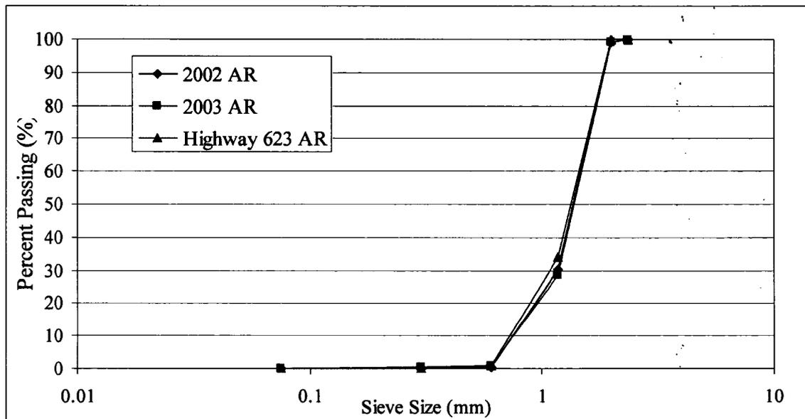
**Figure 3.8 Gradation of CR for Alberta Asphalt Rubber project**
