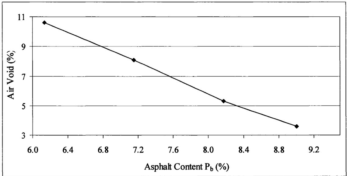
**Figure 4.13 Relationship between asphalt content and air void for dense-graded ARM**
