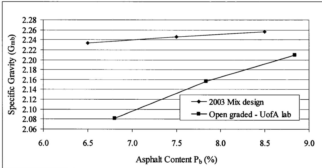
**Figure 4.10 Comparison of  $G_{mb}$  measurement with Corelok with  $G_{mb}$  for 2003 mix design**
