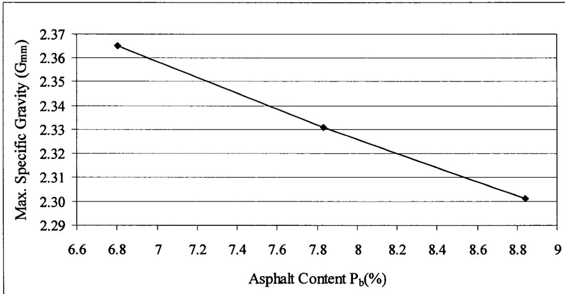
**Figure 4.5 Relationship between asphalt content and maximum specific gravity for open-graded ARM**
