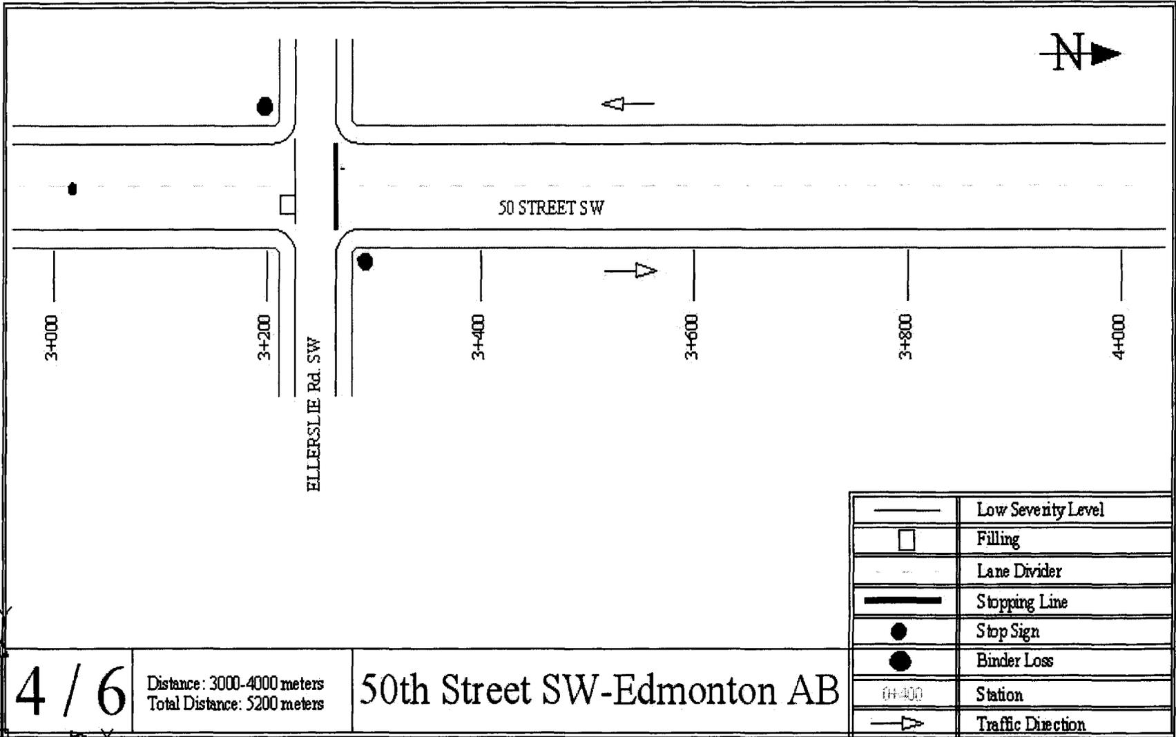
Figure 3.28D Crack measurements map at the 50 Street project locations (3000-4000 m)
