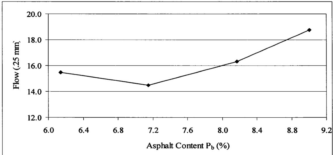
**Figure 4.16 Relationship between asphalt content and flow for dense-graded ARM**
