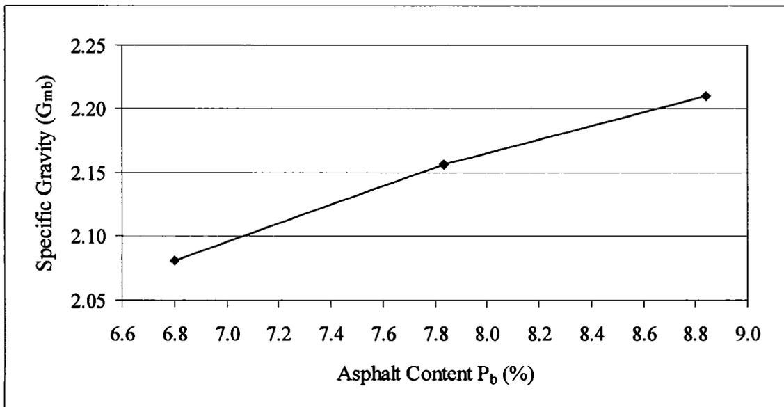
**Figure 4.4 Relationship between asphalt content and specific gravity for open-graded ARM**
