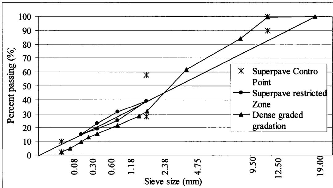
**Figure 4.3 Dense-graded aggregate formulation**
