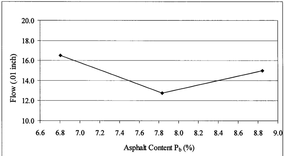
**Figure 4.9 Relationship between asphalt content and flow for open-graded ARM**
