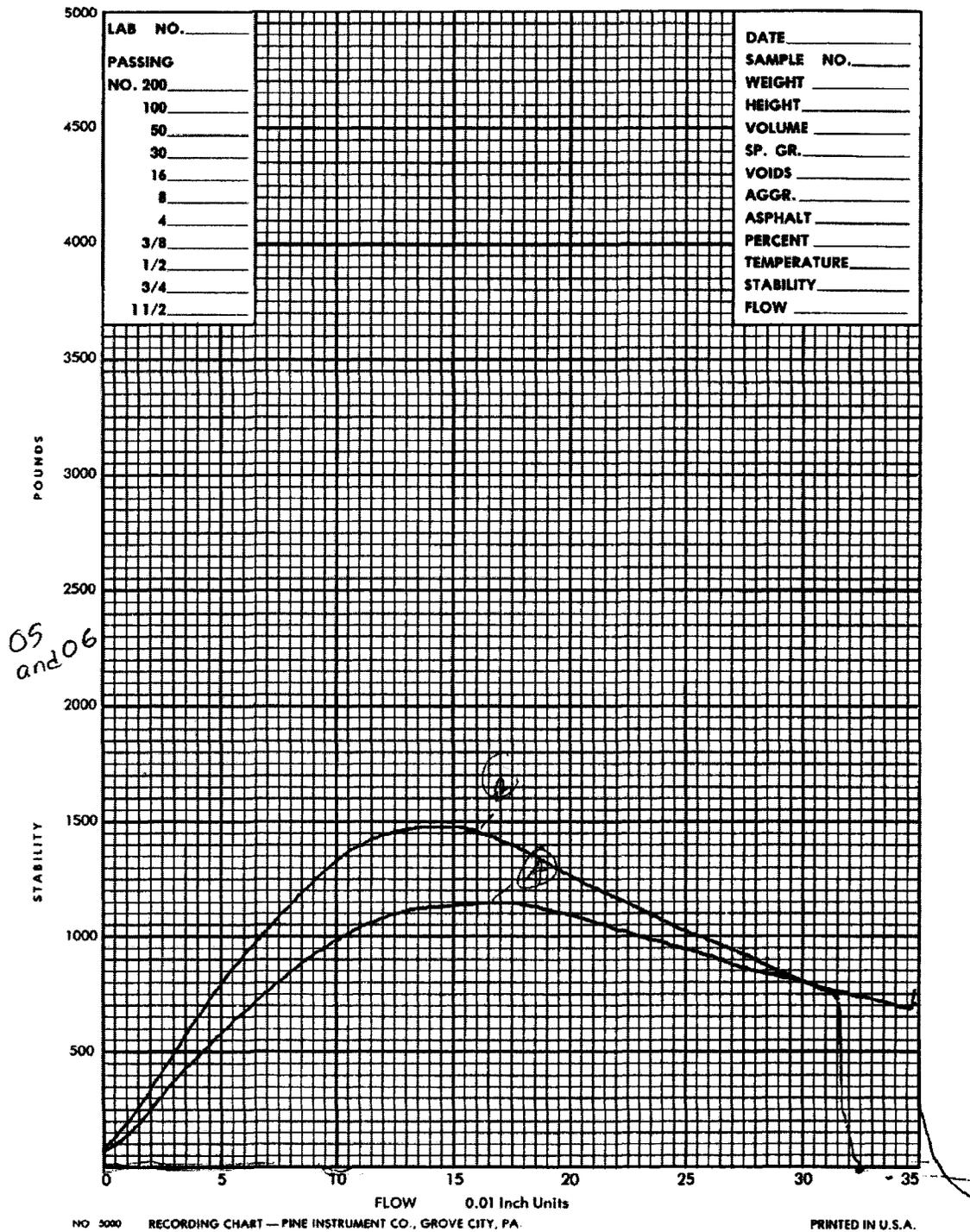
Figure C-5 Tensile strength test for samples O5 and O6
