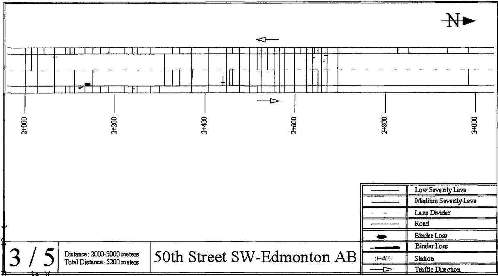
**Figure 3.28C Crack measurements map at the 50 Street project locations (2000-3000 m)**
