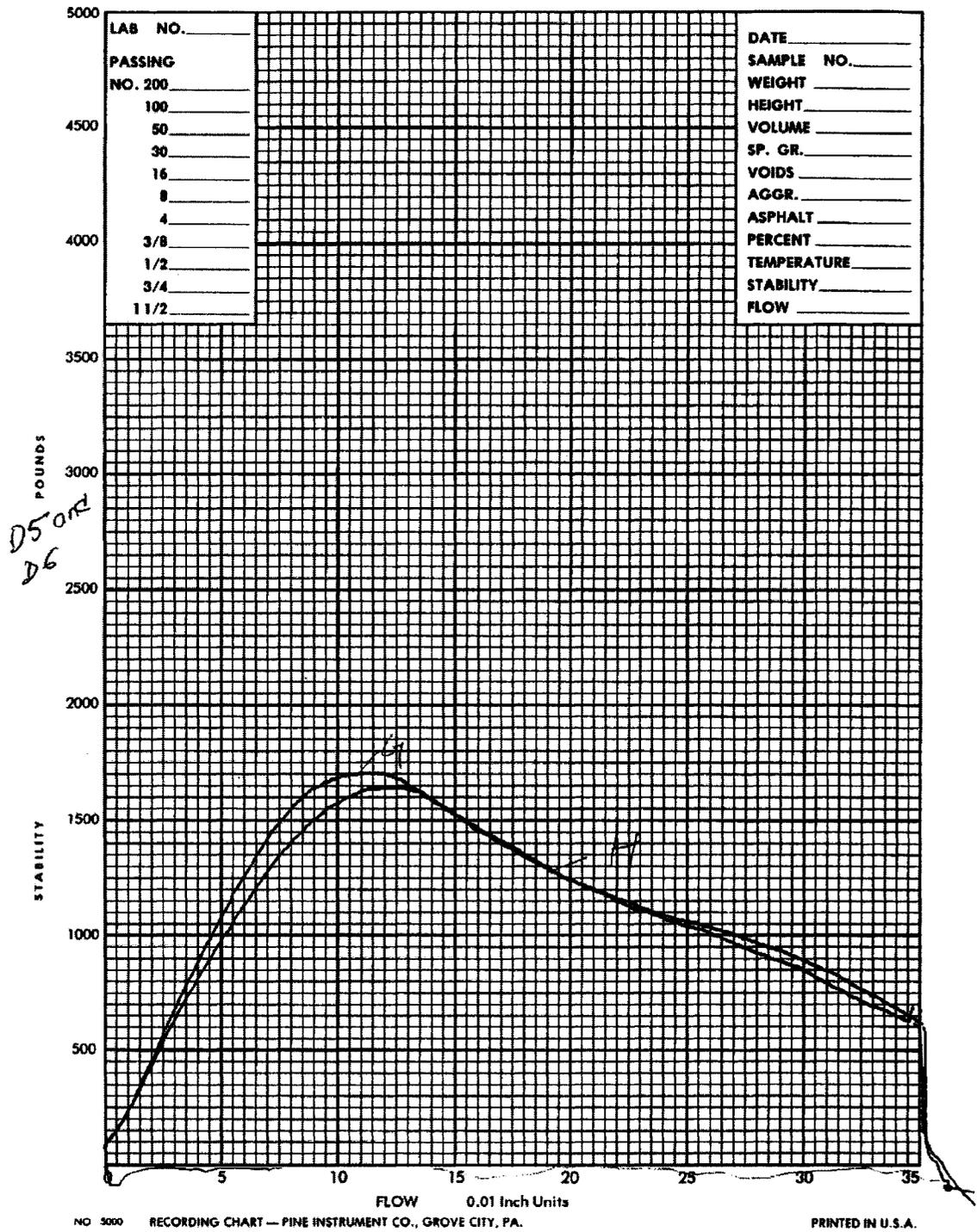
Figure C-6 Tensile strength test for samples D5 and D6
