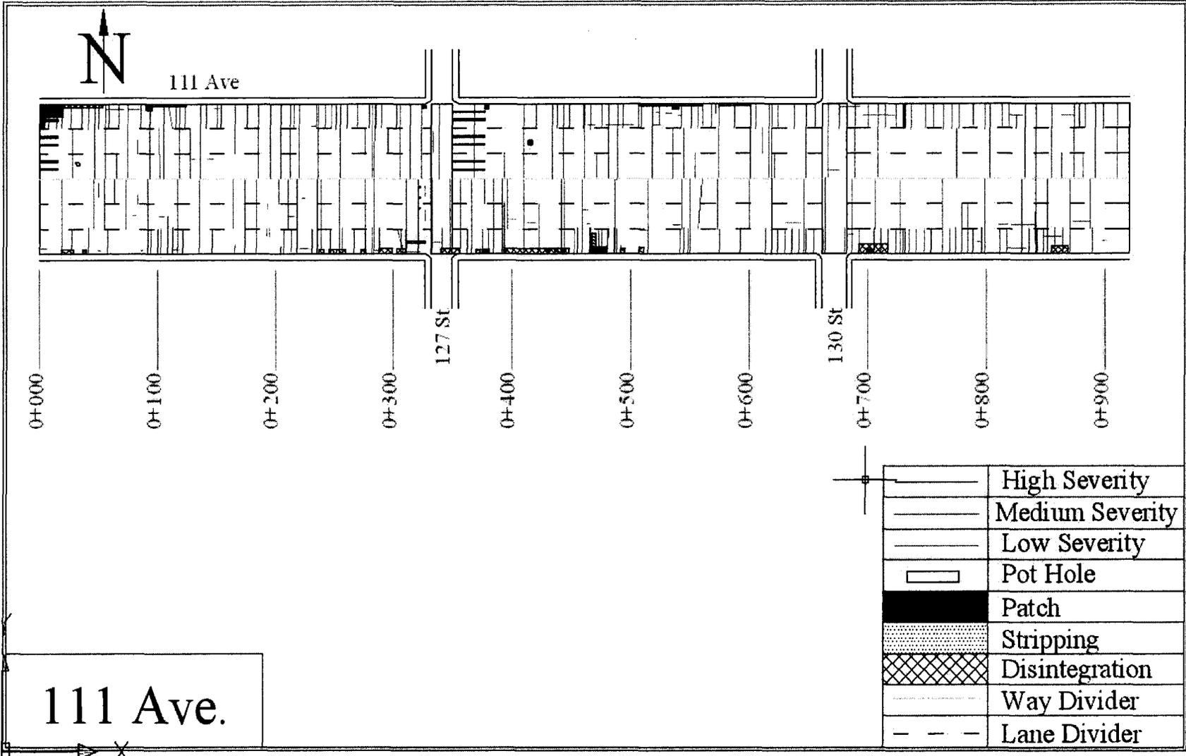
Figure 3.34 Crack measurements map at the 111 Avenue
