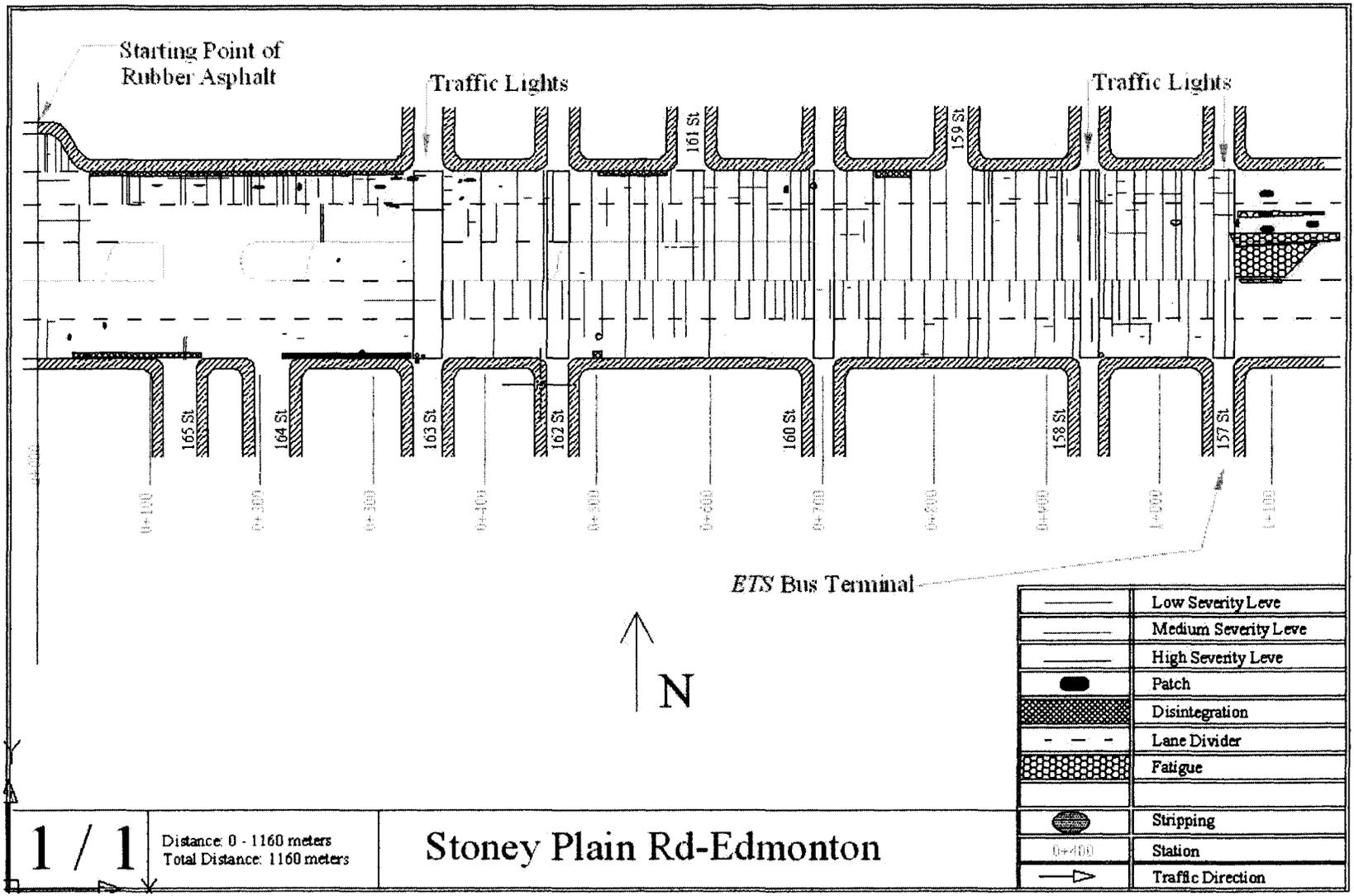
Figure 3.31 Crack measurements map at the Stony Plain Road
