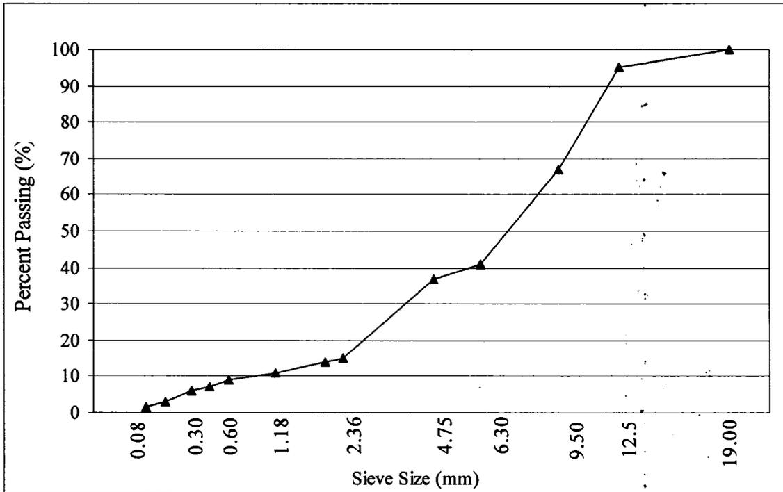
**Figure 3.5 Aggregate gradation for the ARM design (2003 project)**
