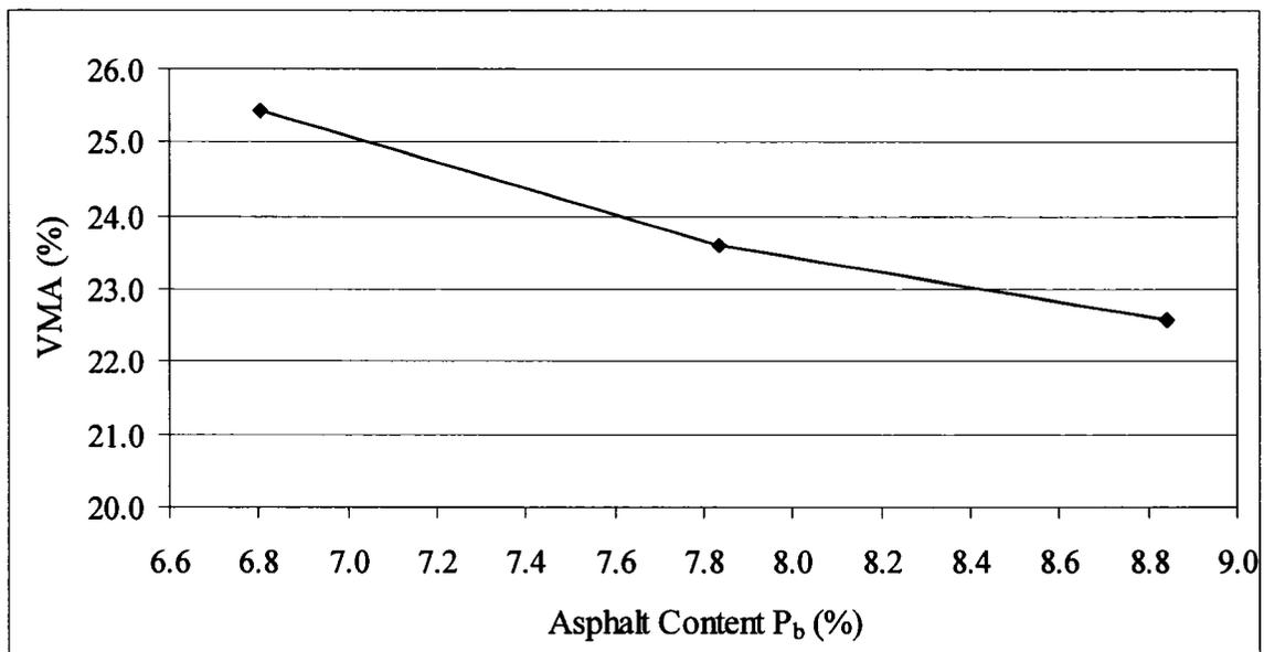
**Figure 4.8 Relationship between asphalt content and VMA for open-graded ARM**
