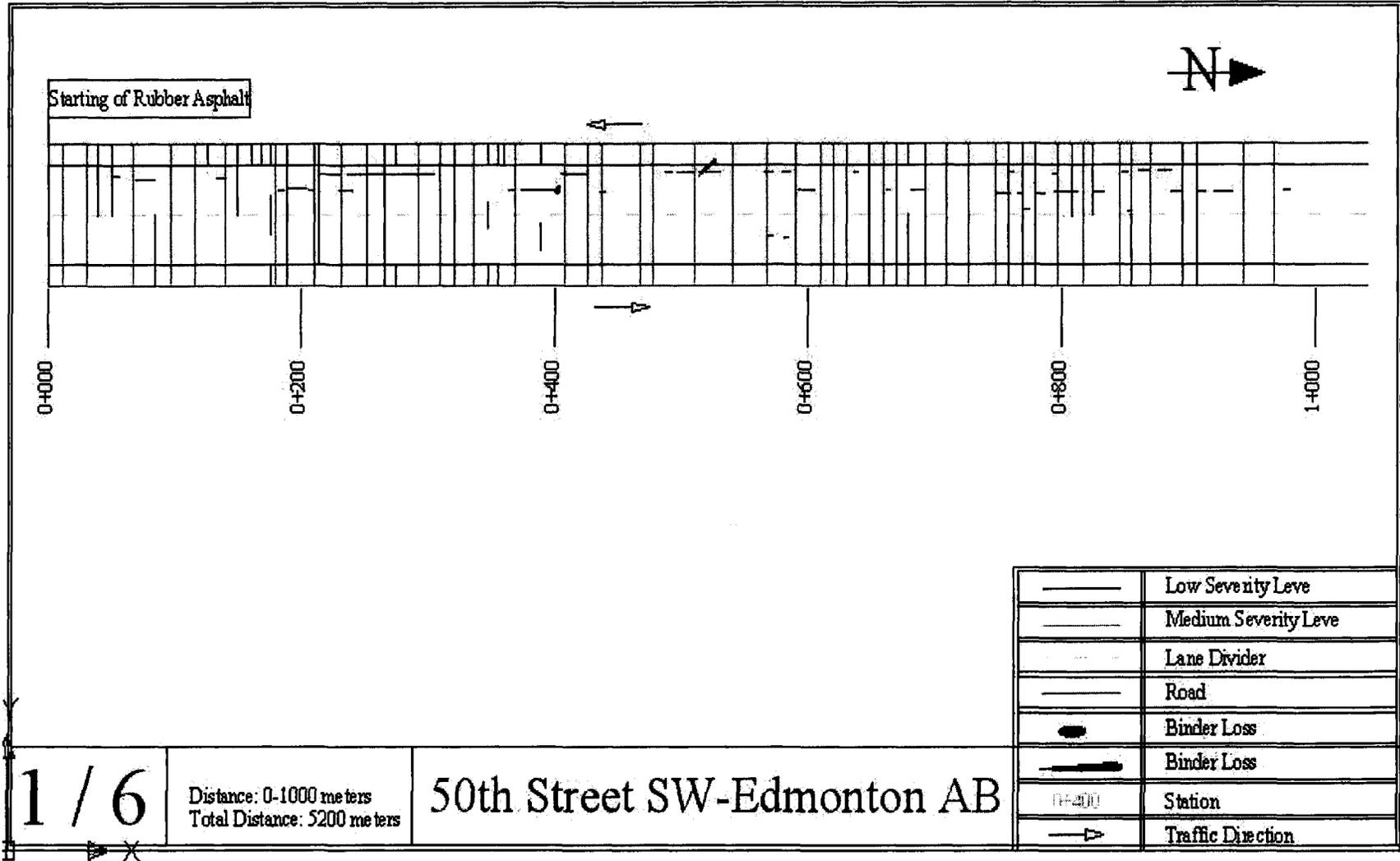
Figure 3.28A Crack measurements map at the 50 Street project locations (0-1000 m)
