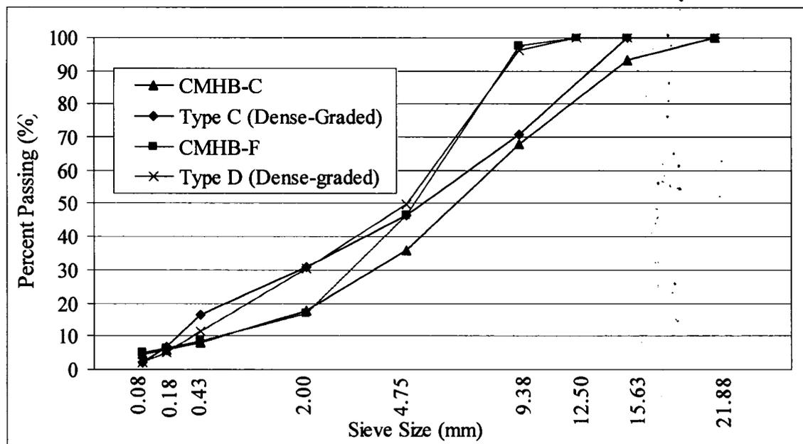
**Figure 2.2 Texas DOT aggregate gradation for ARM overlays**
