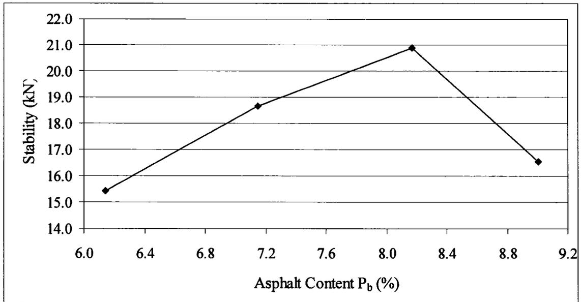
**Figure 4.14 Relationship between asphalt content and stability for dense-graded ARM**
