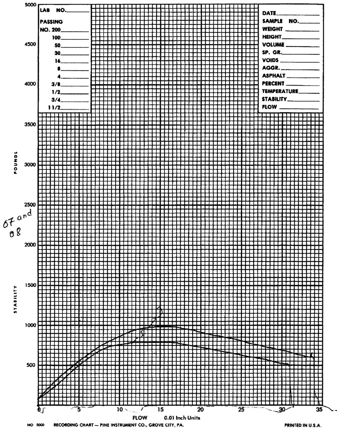
**Figure C-7 Tensile strength test for samples O7 and O8**
