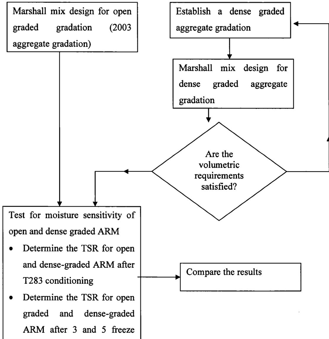
**Figure 4.1 Flowchart showing experimental design**
