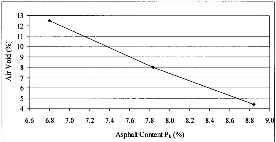
**Figure 4.6 Relationship between asphalt content and air void for open-graded ARM**
