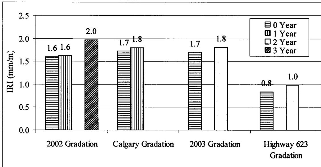
**Figure 3.43 Comparison of the IRI for different aggregate gradation used in 2002 and 2003 Asphalt Rubber project**
