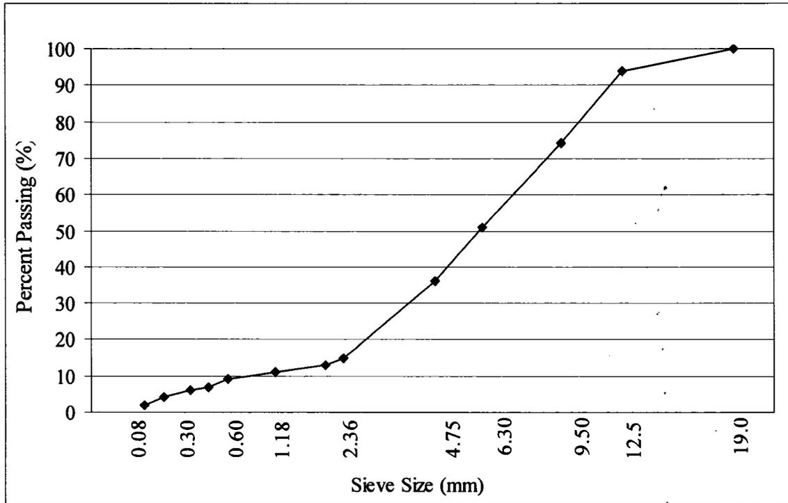
**Figure 3.2 Aggregate gradation for ARM design (2002 projects)**
