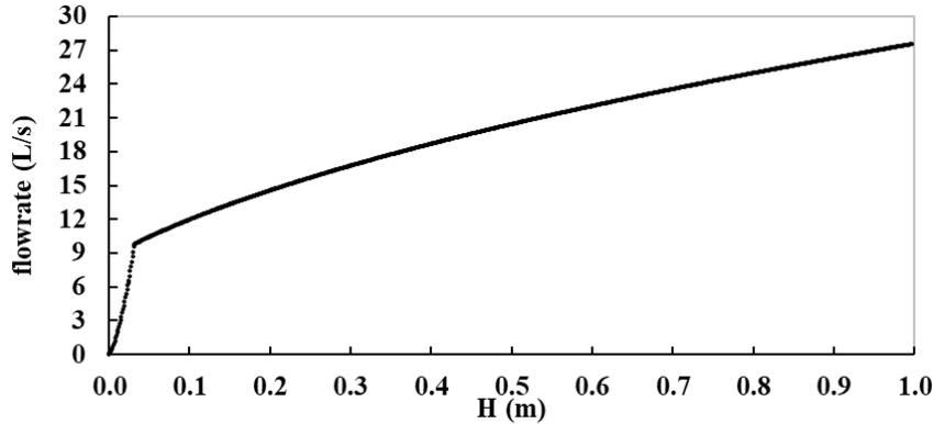
Figure 3-5. Stage outlet discharge curve for the Rocky Ridge wetland where  $Q$  is the discharge and  $H$  is the head on the weir or orifice. Note that zero head corresponds to the NWL.
