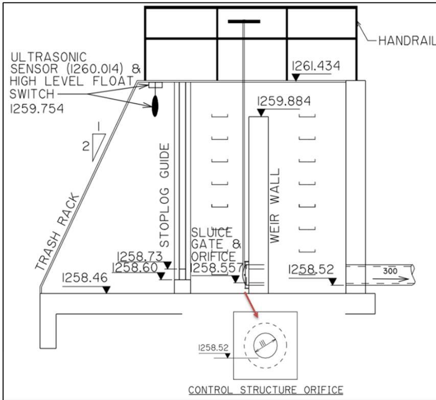
Figure 3-4. Side view of the outlet structure of the Rocky Ridge wetland.
