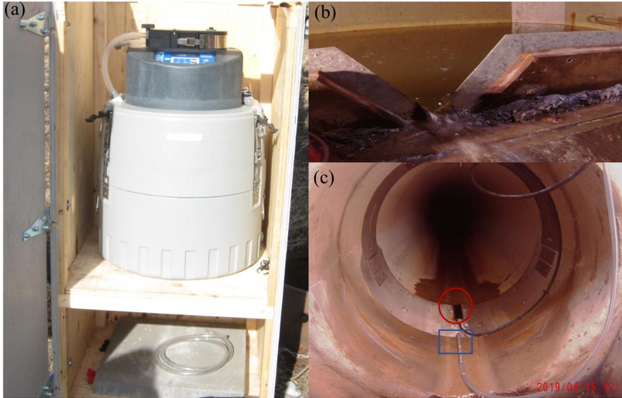
Figure 3-11. (a) ISCO-Teledyne Model 6712 automated sampler located at the outlet of Royal Oak wetland; it was used to collect stormwater samples and store hydrologic data at the sampling point (blue rectangle) in the outlet pipe. Influent and effluent monitoring for wetland: (b) V-notch weir in Royal Oak outlet, (c) outlet pipe, AVM (red circle) inside outlet pipe.
