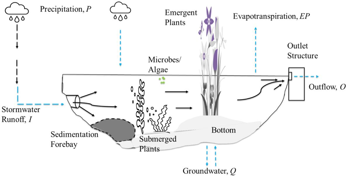
Figure 2-1. Schematic of a stormwater wetland (free water surface), the blue dotted lines indicate components of the water budget.
