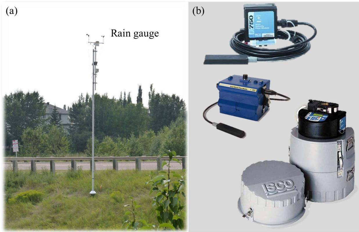
Figure 3-10. A rain gauge (a, Onset Computer Corp., U.S) and the portable auto-samplers Teledyne-ISCO-6712 were equipped with 750/2150 area velocity flow modules (b, Teledyne Isco Inc, U.S).
