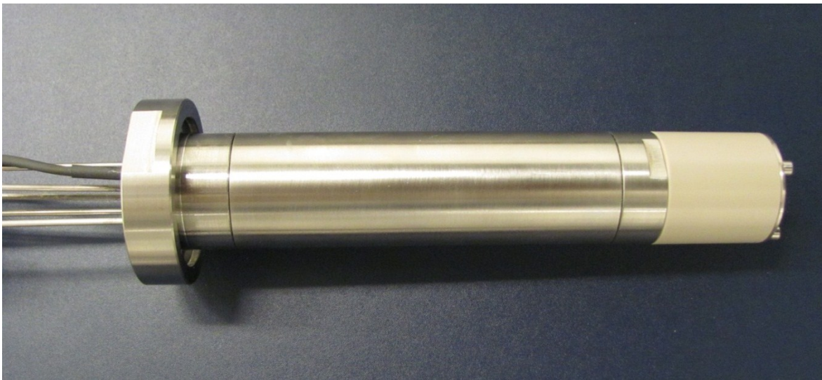
Figure 2.8. Finished atomizer ready to be inserted into commercial spray dryer (Buchi B-190, Buchi Labortechnik AG, Flawil, Switzerland)
