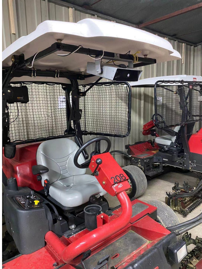
Figure B.1: Cameras mounted on mower
