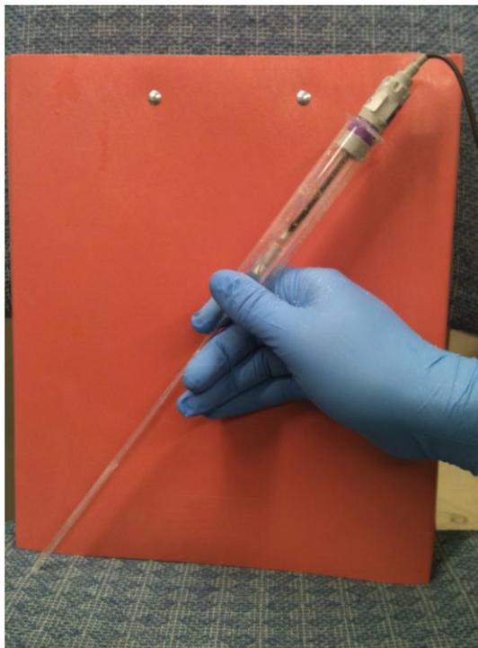
**A.4. Micro-electrodes used for determining the pH inside coating disbondments**
