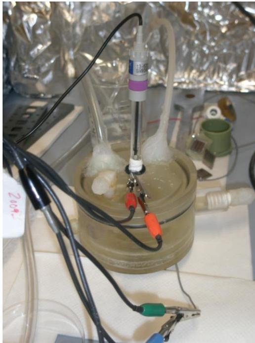
**Figure 5.1: Digital camera image of the test setup used of electrochemical polarization tests.**
