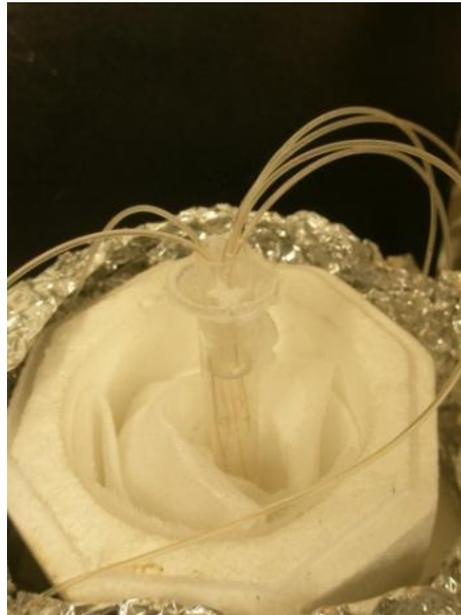
**A.5. Oxygen probe used for determining oxygen concentration in soil solution**
