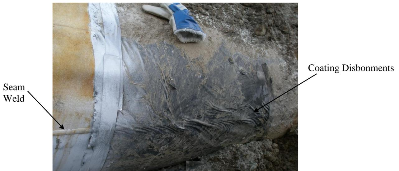
Figure 6.1: Typical image of coating disbondments formed on a seam weld of a pipe section.
