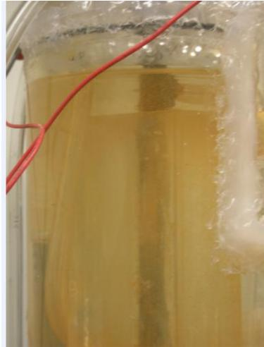
**Figure 5.6: Digital camera image of the specimen inside the corrosion cell at the end of Test B (the test with 1% oxygen).**
