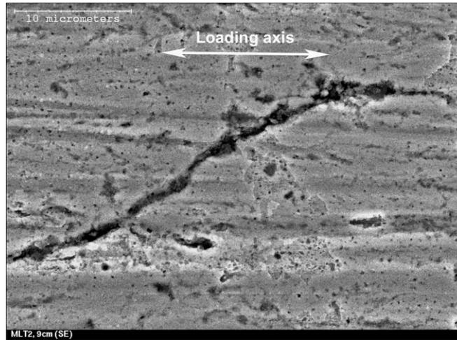
**Figure 4.11: High magnification image showing the formation of several sub-micrometer pits in and around the surface micro-cracks after Test C.**
