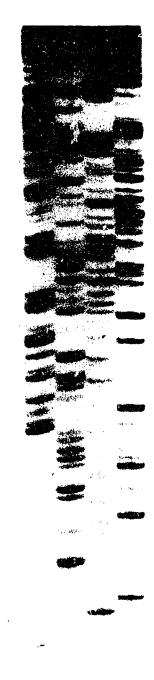
Figure 3.8 - Autoradiograph of the cDNA sequence of a PCR product generated from bursa of Fabricius RNA. cDNA was sequenced by a modified dideoxy cycle sequencing method, electrophoresed on 6% polyacrylamide gels and stained with silver nitrate.
