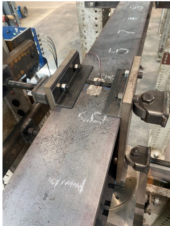
Figure 4-19: Strain gauge mounted to top flange at fulcrum support
