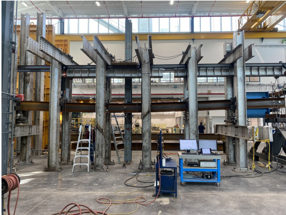
Figure 5-2: Downward deflection on back span and upward deflection at cantilever for LRC4-0.80 at the end of the test
