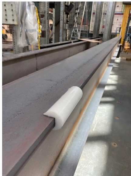
Figure 4-11: Cylindrical Acetal on test girder flange
