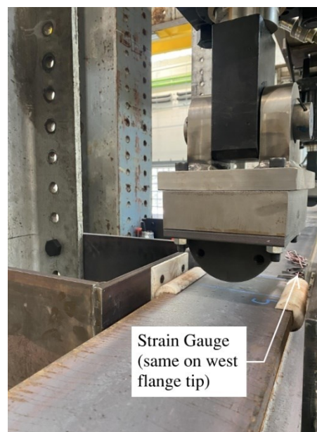
Figure 4-17: Strain gauges mounted to top flange at second load point on back span
