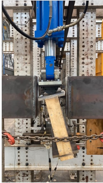
Figure 5-4: Cross-sectional view of cantilever tip at end of LRC2-0.38 test
