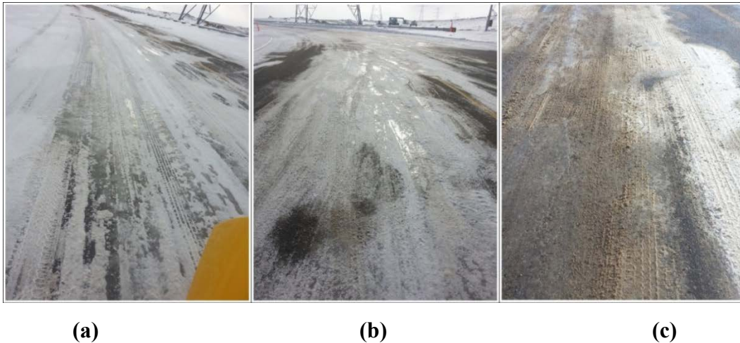
Figure 4-5. Icy road conditions during Feb. 21 tests: (a) Existing ice, (b) plowed ice, and (c) sanded ice after high sanding.
