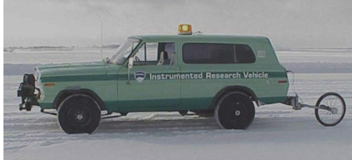
Figure 2-12. The Cold Regions Research and Engineering Laboratory (CRREL) Instrumented Vehicle (CIV) side force friction measurement device (Coutermarsh and Shoop 2009).
