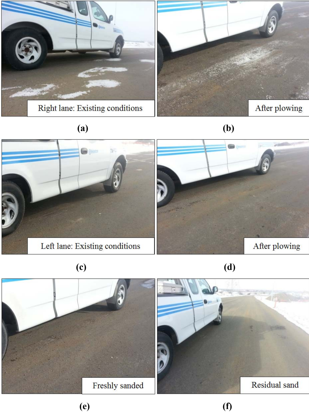
Figure 4-3. Dry road conditions during Feb. 21 tests: (a) dry surface with ice patches along the right lane, (b) plowed right lane, (c) bare dry surface on 200-m of left lane, (d) plowed left lane, and (e) sanded dry surface; (f) Residual sand on dry surface, Mar. 4.
