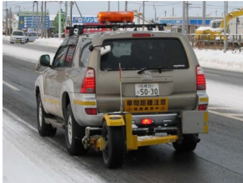
Figure 2-11. Continuous Friction Tester (CFT), a side force friction measurement device, used in a study in Japan (after Tokunaga et al. 2013).
